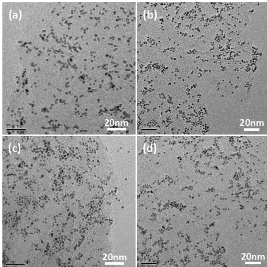
**Figure 6.** TEM images of fresh Pt/Gr. (a) Pt/Gr-200, (b) Pt/Gr-300, (c) Pt/Gr-400, (d) Pt/Gr-500. Different amount of micropores and oxygen active sites of Gr result in various Pt loading and dispersing.
