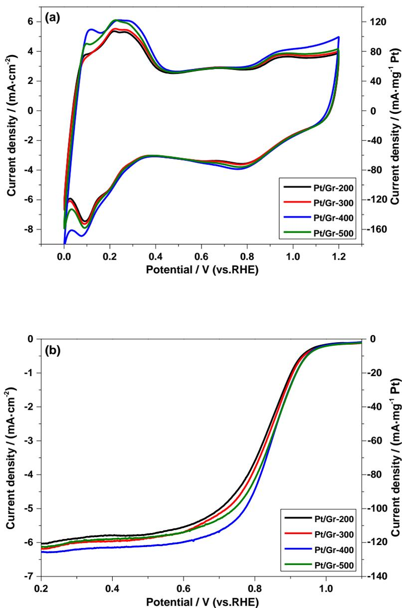
**Figure 7.** The cyclic voltammograms (CVs): (a) and the oxygen reduction linear sweep voltammeteries (LSVs): (b) on fresh Pt/Gr electrodes; CVs were recorded in  $N_2$ -saturated 0.1 M  $HClO_4$  ( $50 \text{ mV}\cdot\text{s}^{-1}$ , room temperature) and LSVs were recorded in  $O_2$ -saturated 0.1 M  $HClO_4$  ( $5 \text{ mV}\cdot\text{s}^{-1}$ , 1600 rpm, room temperature).
