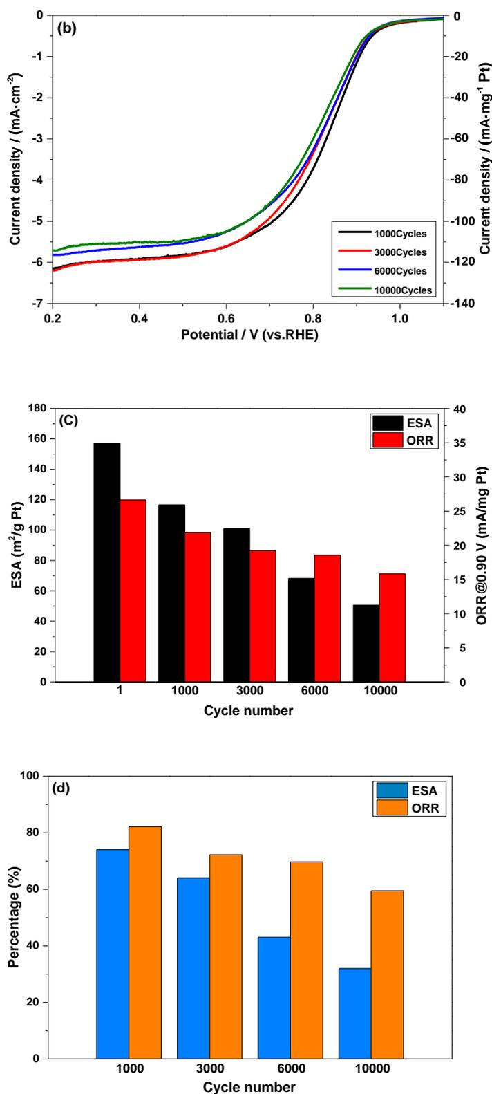
**Figure 8.** Electrochemical properties of Pt/Gr-400 after the durability test under potential steps of 0-1.2 V for 10000 cycles in 0.1 M HClO<sub>4</sub> aqueous solution. (a) Cyclic voltammograms under a scan rate of 50 mV·s<sup>-1</sup>; (b) polarization curves for the O<sub>2</sub> reduction (5 mV·s<sup>-1</sup>, 1600 rpm); (c) original values of ESA and ORR activity at 0.90 V; (d) the percentage of retaining ESA and ORR activity after degradation.
