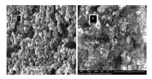
**Figure 2.** SEM image of carbon support (treated with 30 ml  $H_2O_2$  at 80 °C for 24 Hours) A= 0.5µm Bar, B = 10µm Bar.
