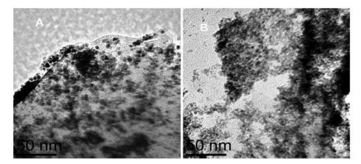
Figure 5. TEM micrograph of 5% PtRu/C nanophase electrocatalyst A) BG-3 B) C3
