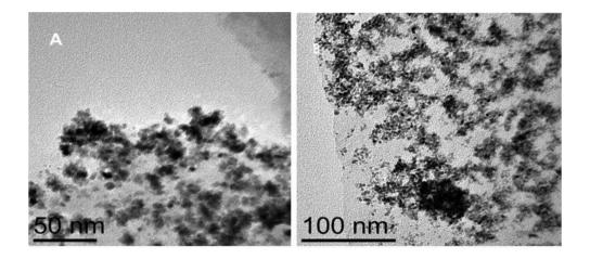
Figure 4. TEM micrograph of 5% PtRu/C nanophase electrocatalyst A) BG-1 at 50 nm B) BG-1 at 50 nm
