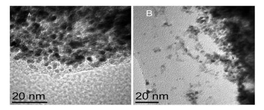
Figure 6. TEM micrograph of 5% PtRu/C nanophase electrocatalyst A) BG-5 B) BG-6
