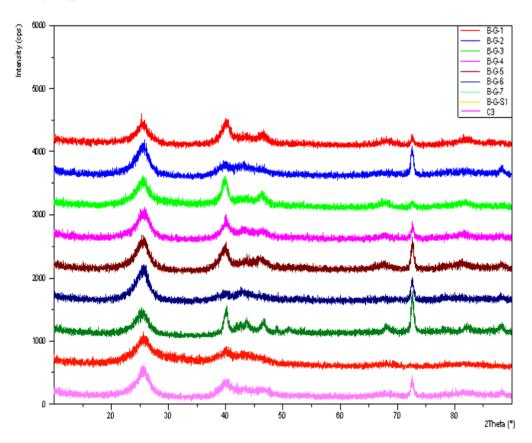
Figure 1. Combined PXRD pattern of synthesized 5% PtRu/C electrocatalysts
