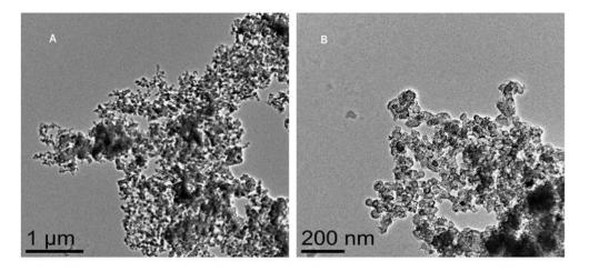
Figure 3. TEM micrographs of carbon support A) 1µm B) 200nm Scale
