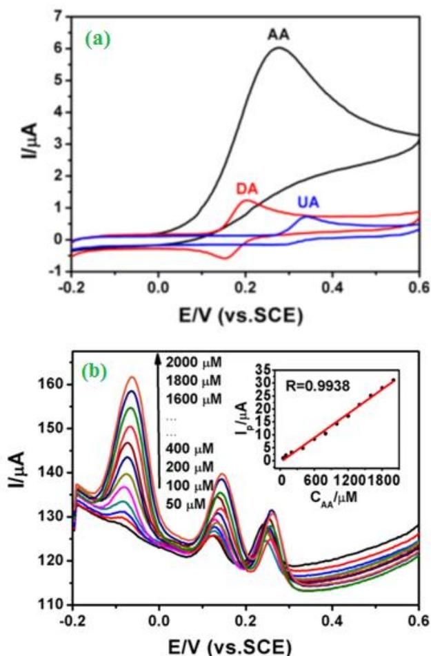
**Figure 6.** (a) Cyclic voltammograms of 400  $\mu\text{M}$  AA, 15  $\mu\text{M}$  DA, and 30  $\mu\text{M}$  UA at GCE (b) Differential pulse voltammograms at N-S-PC/GCE in 0.1 M PBS (pH 7.0) containing 3  $\mu\text{M}$  DA, 4  $\mu\text{M}$  UA, and different concentration of AA. ("Reprinted with permission from (*ACS Appl. Mater. Interfaces* 6 (2014) 19109-19117). Copyright (2014) American Chemical Society").
