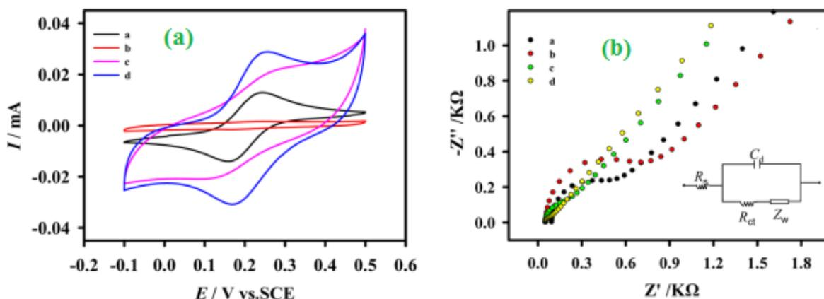
**Figure 3.** CVs (a) and EIS (b) of bare GCE (a), GO/GCE (b), PDA-rGO/GCE (c), and Fc-NH-PDA-rGO/GCE (d) in 2mM  $\text{Fe}(\text{CN})_6^{3-/4-}$  containing 0.1 M  $\text{Na}_2\text{SO}_4$ . ("Reprinted with permission from (*ACS Appl. Mater. Interfaces* 7 (2015) 17935-17946). Copyright (2015) American Chemical Society")
