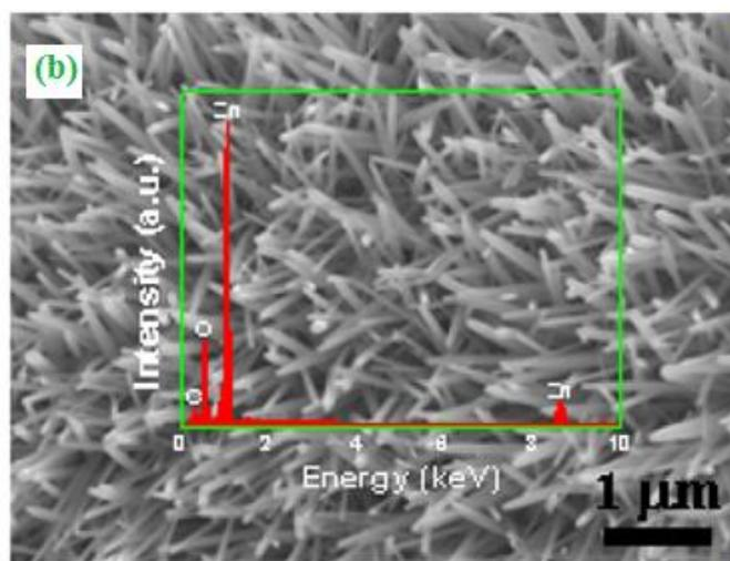
**Figure 2.** (a) Schematic of the ZnO NWA/GF electrode and detection of UA, DA, and AA. (b) SEM images of the ZnO NWAs on the 3D GF at different magnifications. Inset: EDX of the ZnO NWAs. ("Reprinted with permission from (*ACS Nano* 8 (2014) 1639-1646). Copyright (2014) American Chemical Society")
