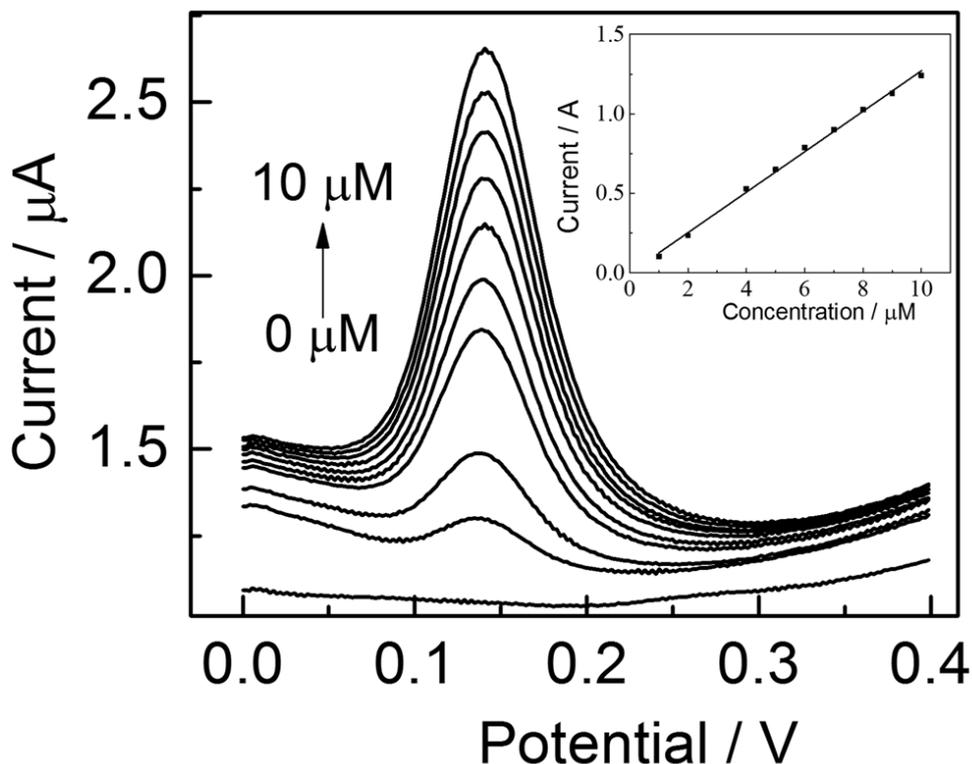
**Figure 7.** Square wave voltammetry in the potential range 0 to + 0.4 V at carbon-black modified glassy carbon (CB-GCE) in 0.1 M phosphate buffer with continual addition of dopamine (DA) such that [DA] varies between 0 µM to 10 µM. ("Reprinted with permission from (*ACS. Appl. Mater. Interfaces* 8 (2016) 28338-28348). Copyright (2016) American Chemical Society").
