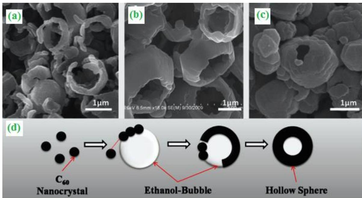
**Figure 8.** Studies on the plausible mechanism for the formation of C<sub>60</sub> hollow microspheres. SEM of (a) C<sub>60</sub> hemi-rings, (b) bows, and (c) almost completely spheres and (d) Plausible mechanism for the formation of C<sub>60</sub> hollow microspheres with bubble-template. ("Reprinted with permission from (*ACS Appl. Mater. Interfaces* 4 (2012) 1594-1600). Copyright (2012) American Chemical Society").
