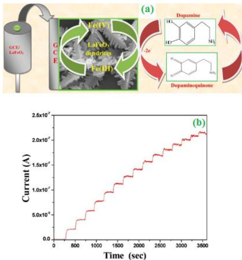
**Figure 5.** (a). Schematic illustration of electrocatalytic dopamine oxidation at the  $LaFeO_3$  dendrite nanostructure modified GCE. (b) Amperometric i-t curve for the determination of DA at the  $LaFeO_3$  dendrite modified electrode in 10 mM PBS 7.2. Each addition increases the concentration of 100 nM at regular intervals of 180s. ("Reprinted with permission from (*Cryst. Growth Des* 13 (2013) 291-302). Copyright (2013) American Chemical Society")
