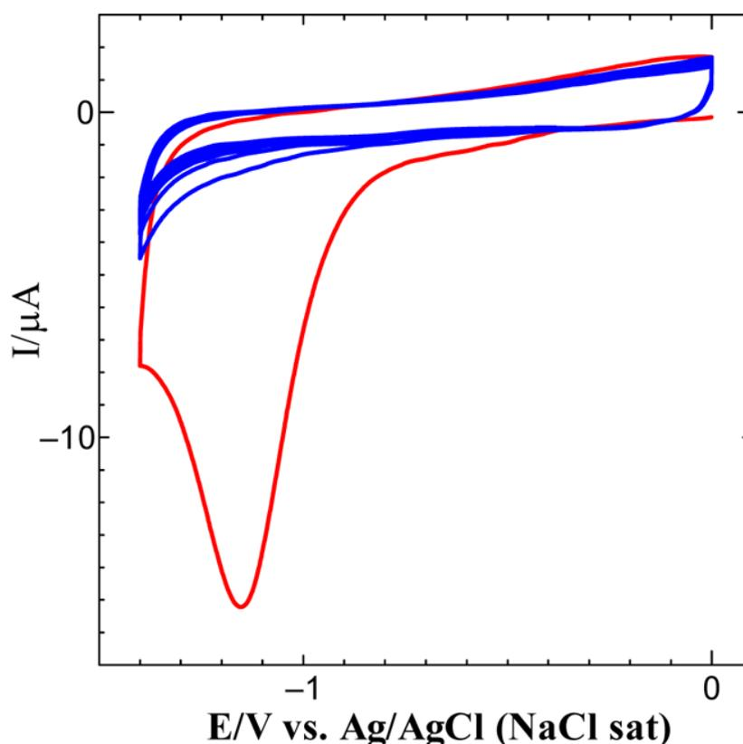
**Figure 1.** Electrochemical reduction of electrostatically assembled GO on GC/HDA electrode (15 cycles) in 0.2 M PB solution (pH 7.2) at a scan rate of  $100 \text{ mV s}^{-1}$ . ("Reprinted with permission from (*J. Phys. Chem. C* 117 (2013) 4326-4335). Copyright (2016) American Chemical Society")
