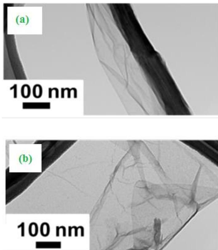
**Figure 4. (a & b)** Transmission electron microscopy images of a single as-received multi-walled carbon nanotube and graphene oxide nanoribbons derived from unzipping by treatment with  $\text{H}_2\text{SO}_4 + \text{H}_3\text{PO}_4$  with dissolved  $\text{KMnO}_4$  under microwave powers of 150 and 250 W applied for 4 min. ("Reprinted with permission from *ACS Nano* 5 (2011) 7788-7795). Copyright (2011) American Chemical Society")
