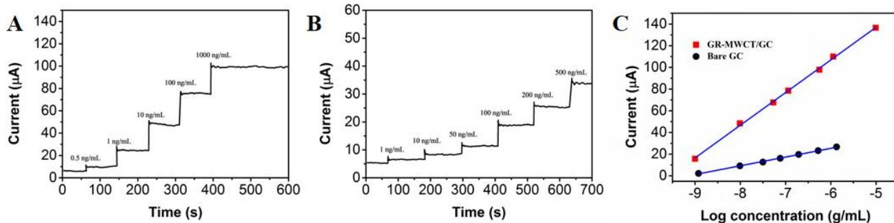
**Figure 3.** Amperometric results for (A) GR-MWCT/GC electrode and (B) bare GC electrode constructed electrochemical immunosensor incubated with different concentrations of human Apo-A protein in the range of 0.5-1000 ng/mL. (C) The calibration plots of amperometric response in function of logarithm of human Apo-A concentration.
