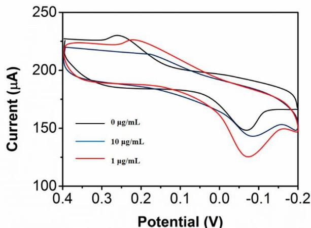
**Figure 2.** CVs of as-prepared immunosensor with Apo-A at different concentrations. The red dash line represents the reduction potential of  $\text{H}_2\text{O}_2$  at  $-0.08$  V.
