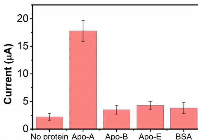
**Figure 4.** Current responses of as-prepared Apo-A electrochemical immunosensors for the detection of different analytes (0.5 μg/mL Apo-A, 1 μg/mL BSA, 1 μg/mL Apo-B and 1 μg/mL Apo-E). The error bars represent the standard deviation calculated with three independent experiments.
