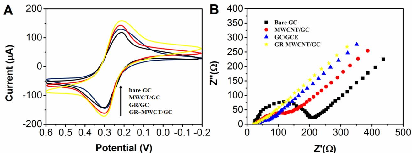
**Figure 1.** (A) Cyclic voltammograms and (B) electrochemical impedance spectra of bare GC, MWCT/GC, GR/GC and GR-MWCT/GC electrodes.
