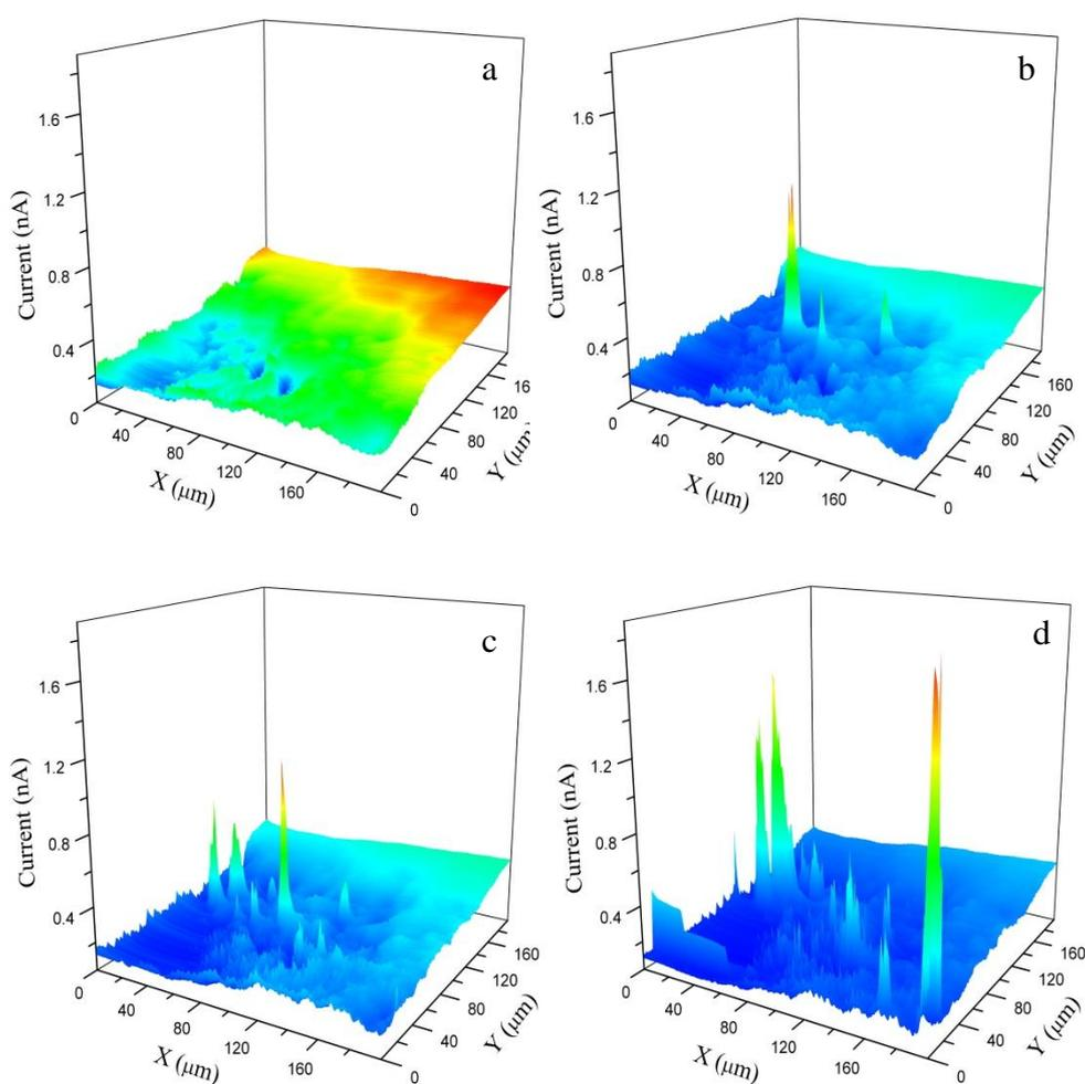
**Figure 4.** SECM images of magnesium alloy AZ91D with MAO coating anodized at 140V immersed in 0.5 mM FcMeOH + 0.1 M NaCl solution. The images were taken at (a) 0.5, (b) 1.5, (c) 3.5 and (d) 5.5 h after immersion in the solution.
