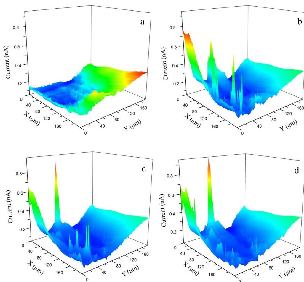
**Figure 5.** SECM images of magnesium alloy AZ91D with MAO coating anodized at 100V immersed in 0.5 mM FcMeOH + 0.1 M NaCl solution. The images were taken at (a) 0.5, (b) 1.5, (c) 3.5 and (d) 5.5 h after immersion in the solution.
