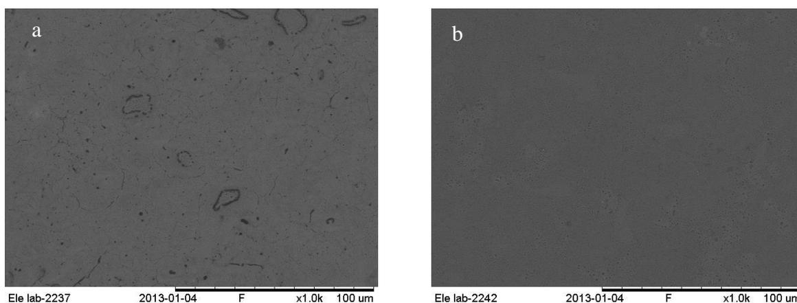
**Figure 1.** Typical SEM micrographs of the MAO coating anodized under different applied voltage: (a) 140 V and (b) 100 V.
