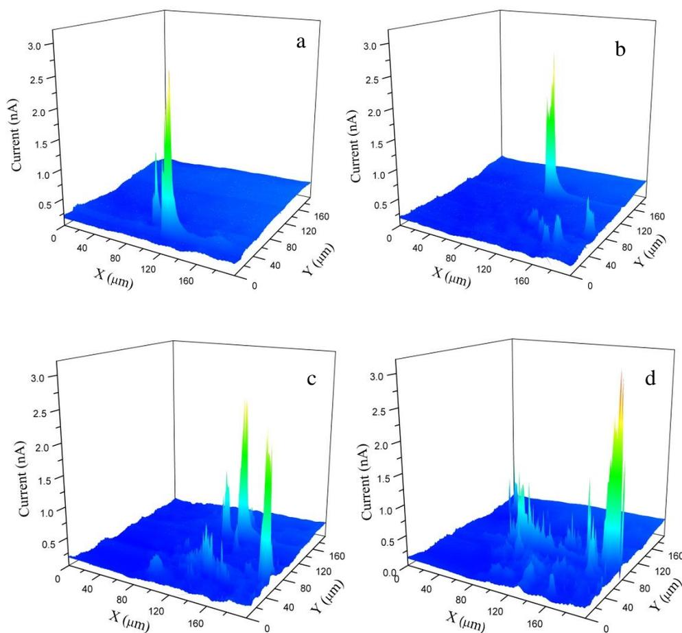
**Figure 3.** SECM images of magnesium alloy AZ91D with MAO coating anodized at 140V immersed in 0.5 mM FcMeOH + 0.62 M NaCl solution. The images were taken at different immersion time, (a) 0.5, (b) 1.5, (c) 3.5 and (d) 5.5 h.
