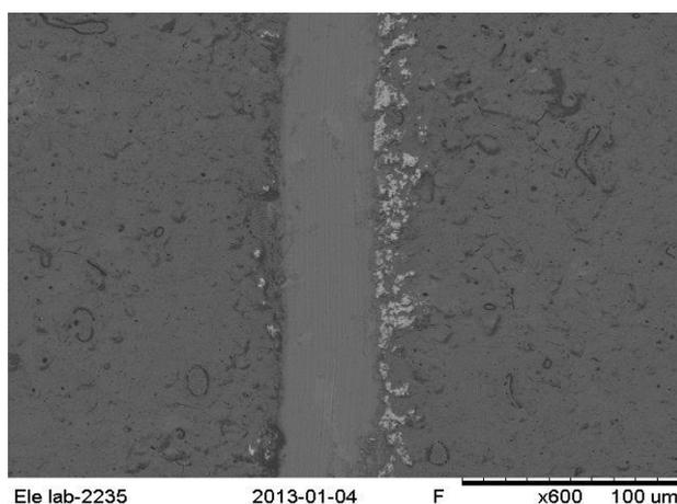
**Figure 6.** SEM surface images of the artificial scratch on AZ91D magnesium alloy with MAO coating.
