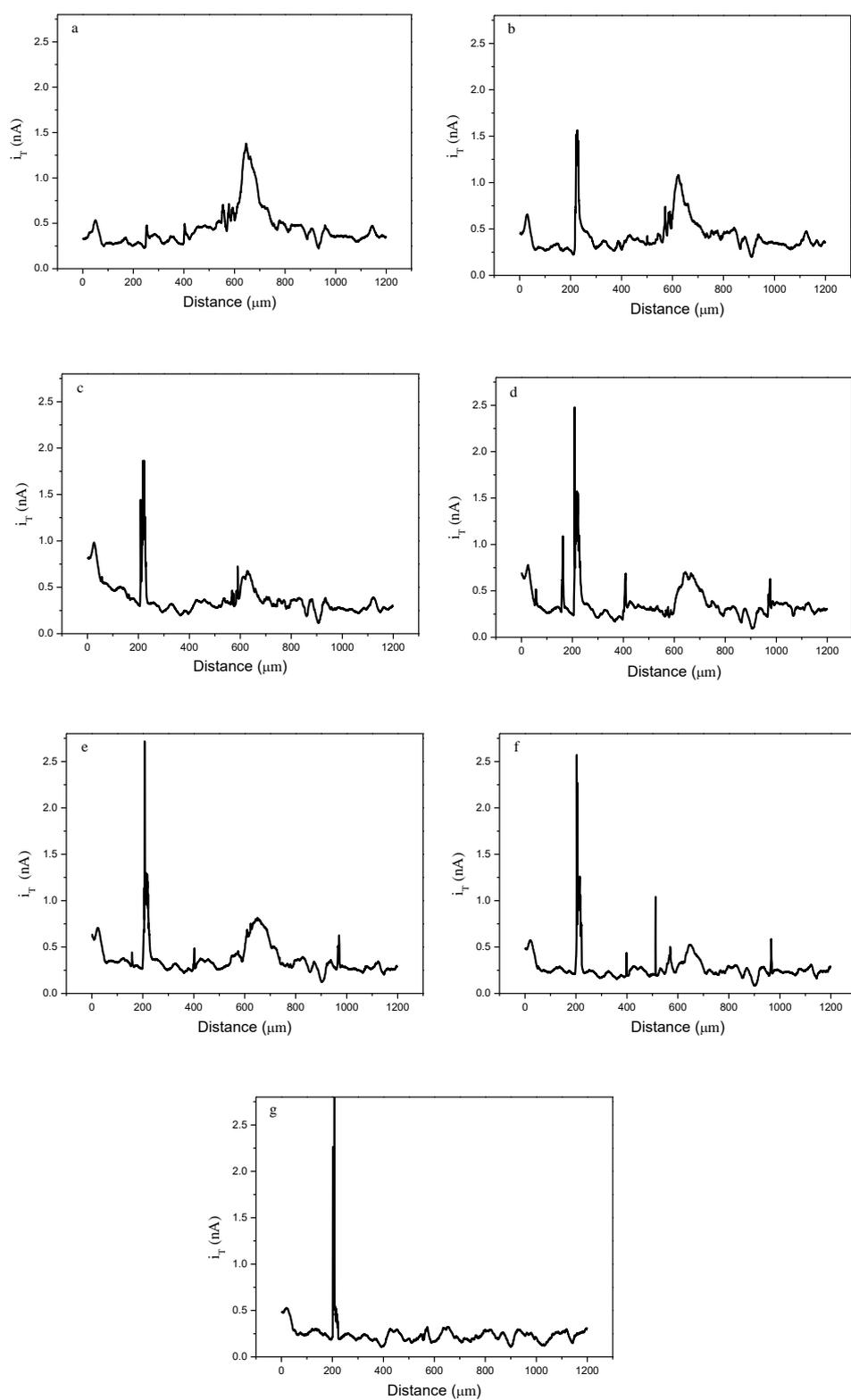
**Figure 7** Scanning lines across an artificial scratch of magnesium alloy AZ91D with MAO coating immersed in 0.5 mM FcMeOH + 0.1 M NaCl solution for different time: (a) 30, (b) 40, (c) 50, (d) 60, (e) 70, (f) 80 and (g) 120 min.
