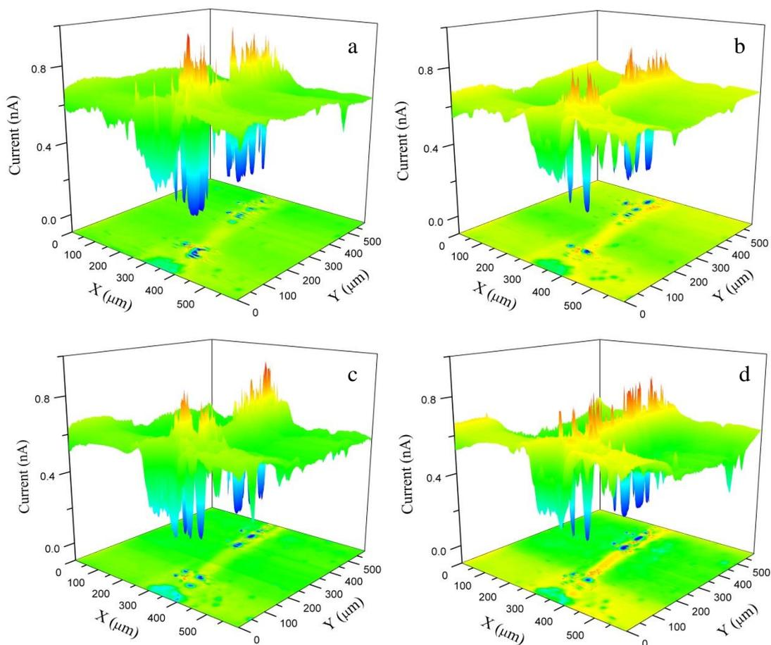
**Figure 8.** SECM images over the artificial scratch on AZ91D magnesium alloy with MAO coating immersed in 0.5 mM FcMeOH + 0.1 M NaCl solution. The images were taken at different immersion time, (a) 0.5, (b) 1.5, (c) 3.5 and (d) 5.5 h.
