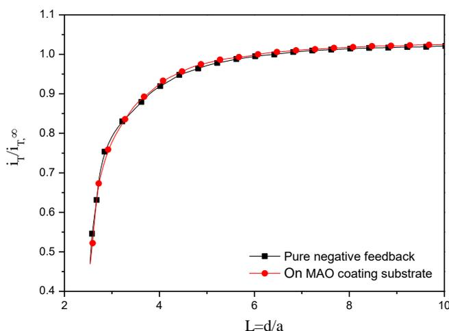
**Figure 2.** Probe approach curves to the MAO coating substrate recorded in 0.5 mM FcMeOH + 0.1 M NaCl aqueous solution with 10  $\mu\text{m}$  Pt tip at a bias potential of 0.45 V vs. Ag/AgCl. The black square line is pure negative feedback curve based on COMSOL simulation.
