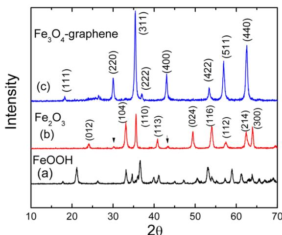
**Figure 1.** XRD patterns for the hydrothermal product: (a) FeOOH, (b) the annealed product of FeOOH under an argon atmosphere at 450°C for 2 hours, and (c) the nanostructured Fe<sub>3</sub>O<sub>4</sub>/graphene composite prepared by annealing FeOOH and graphene composite in an argon atmosphere at 450°C for 2 hours.
