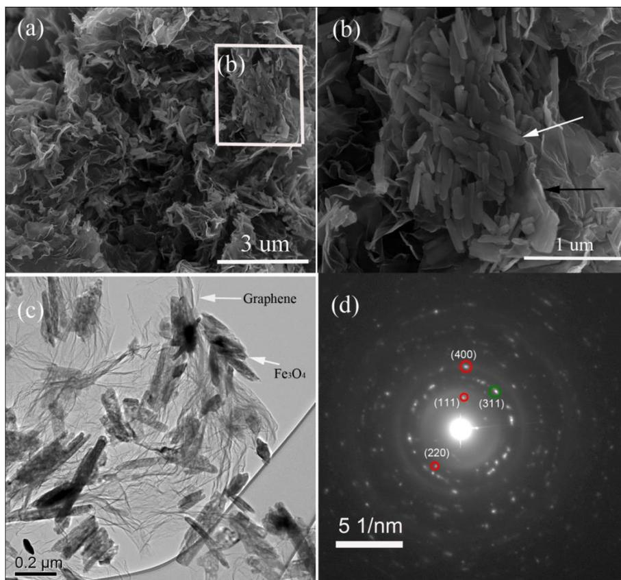
**Figure 4.** Structural characterization of the  $\text{Fe}_3\text{O}_4$ /graphene composite: SEM images obtained at low magnification (a), SEM images obtained at high magnification (b) (the white arrow indicates the  $\text{Fe}_3\text{O}_4$  nanorod, and the black arrow indicates the graphene sheets), TEM image (c), and the corresponding diffraction pattern (d).
