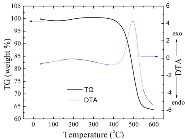
**Figure 3.** TG and DTA curves of  $\text{Fe}_3\text{O}_4$ /graphene nanocomposite. The air flow rate was  $50 \text{ cm}^3 \text{ min}^{-1}$ , and the temperature ramp rate was  $10^\circ\text{C}/\text{min}$ .
