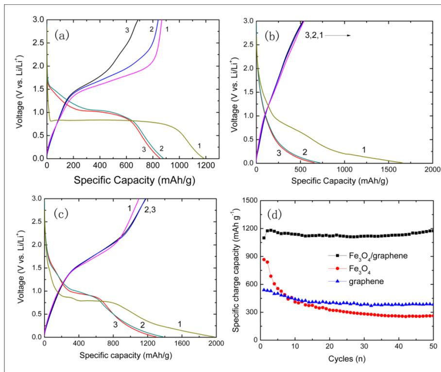
**Figure 6.** Discharge/charge curves of the first three cycles for the micro-sized  $\text{Fe}_3\text{O}_4$  electrode (a), the graphene (b), and the  $\text{Fe}_3\text{O}_4$ /graphene nanocomposite (c), and their cycling performances (d).
