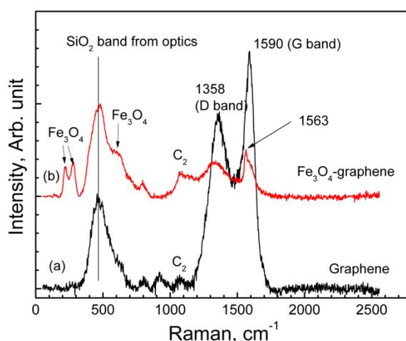
**Figure 2.** Raman results of pristine graphene (a) and  $\text{Fe}_3\text{O}_4$ /graphene nanocomposite (b).
