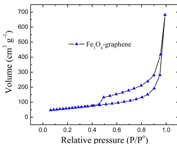
**Figure 5.** Nitrogen sorption isotherms measured at 77K of the  $\text{Fe}_3\text{O}_4/\text{graphene}$  nanocomposite.
