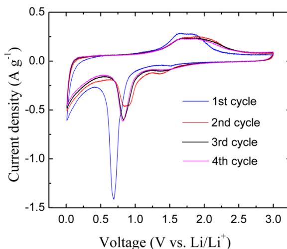
**Figure 7.** Initial four cycles of CV curves of Fe<sub>3</sub>O<sub>4</sub>/graphene electrodes.
