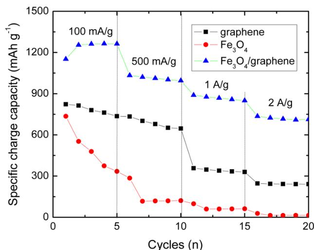
**Figure 8.** Rate capabilities of the  $\text{Fe}_3\text{O}_4/\text{graphene}$  composite, micro-sized  $\text{Fe}_3\text{O}_4$ , and graphene at various current densities. The applied current for discharge and charge process of each cycle is the same.
