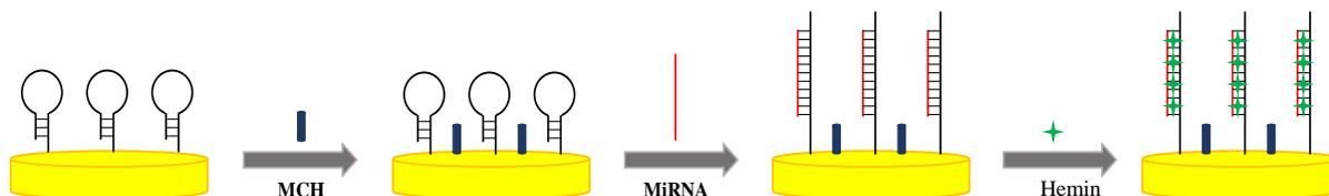
**Figure 1.** The principle behind the electrochemical detection of miRNA by porphyrin.
