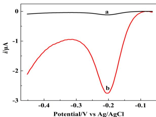
**Figure 3.** Cyclic voltammograms (CVs) acquired at hairpin probe immobilized Au electrode(a) after hybridization miRNA (b) at room temperature. Followed by intercalation of hemin. The scan rate was 0.1 V/s, and the arrow indicates the scan direction.
