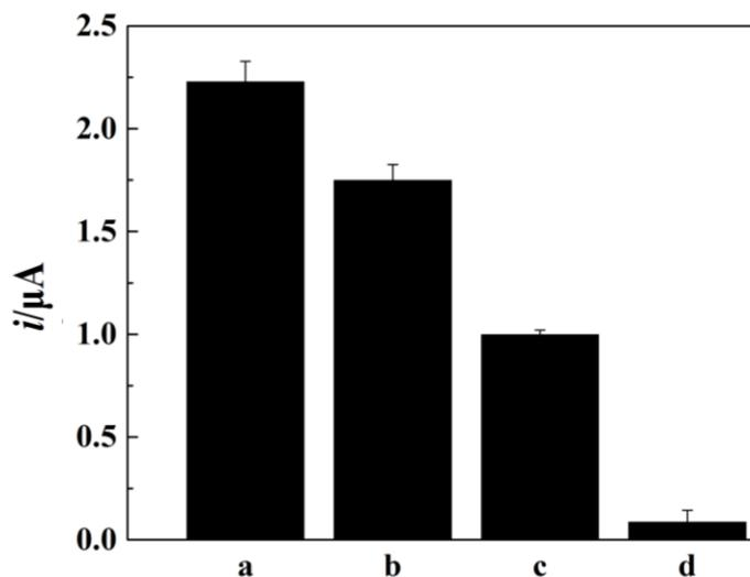
**Figure 4.** Specificity of miRNA assay. The peak currents were measured at electrodes modified with probe DNA hybridize with 0.1 nM complement (a), single mismatch (b), four-base mismatch (c), and non complement(d) miRNAs with hemin insertion. The absolute errors deduced from three replicate measurements were shown as the error bars. Other experimental conditions are the same as those in Figure 3.
