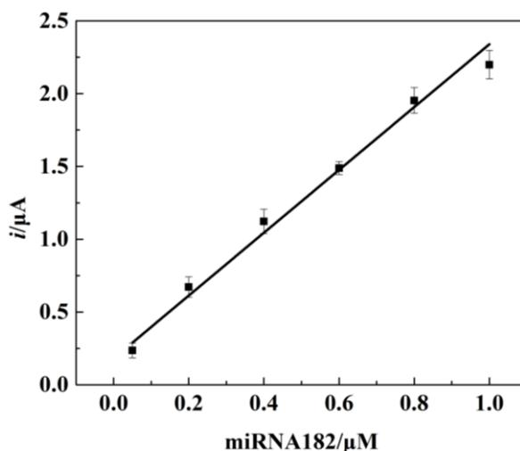
**Figure 5.** Dependence of the peak currents on the concentrations of target miRNA. The absolute errors were deduced from three replicate measurements and shown as the error bars.
