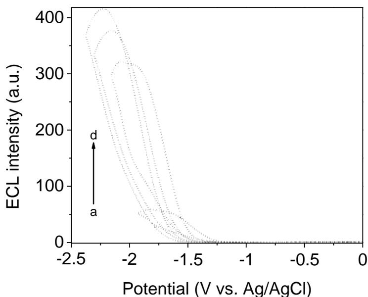
Figure 6. Effects of potential and ECL intensity on Nafion-GCE with four sized CdTe quantum dots
