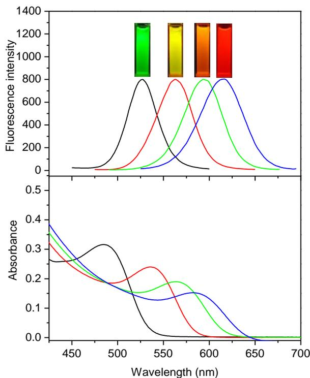
**Figure 2.** Absorption and fluorescence emission spectra of four thioglycollic acid capped CdTe quantum dots with heating (a) 80 min, (b) 135 min, (c) 175 min, and (d) 220 min, respectively
