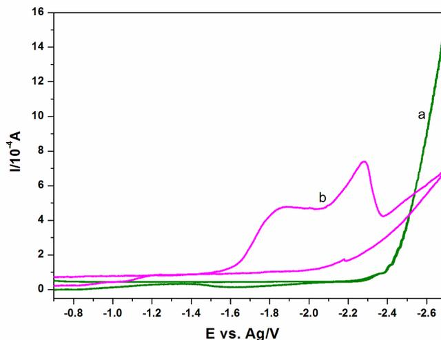
**Figure 3.** Cyclic voltammograms recorded with as-prepared nano Ag cathode (a) neat  $\text{BMIMBF}_4$ ; (b)  $\text{BMIMBF}_4$  saturated with  $\text{CO}_2$ .
