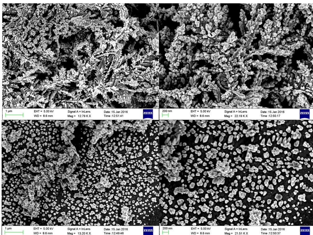
**Figure 1.** SEM image of as-prepared nano-silver (a) no PEG or PVP, (b) enlarged detail (a), (c) polyethylene glycol (PEG), and (d) PVP
