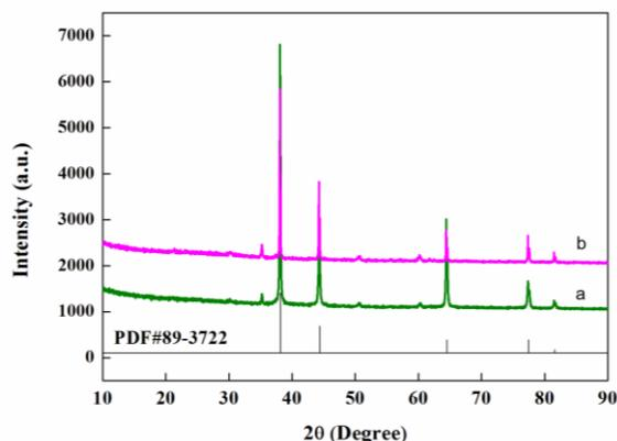
**Figure 2.** X-ray diffraction patterns as-prepared nano Ag cathode (a) PEG (b) PVP
