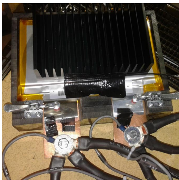
Figure 3. Connected cell holder for an AMP20M1HDA cell during testing.
