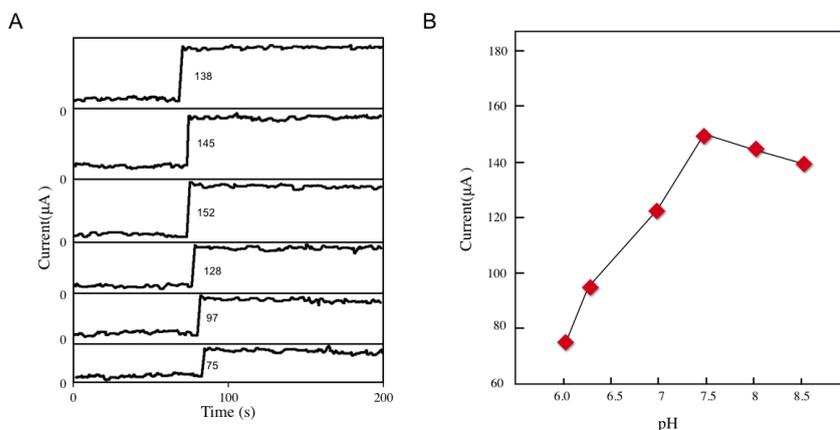
**Figure 3.** Influence of the pH of the solution on the response of the immunosensor incubated with 20 ng/ml MMP-9 in 5 mM  $\text{Fe}(\text{CN})_6^{4-/3-}$  solution containing 0.1 M KCl. All potentials are given vs. SCE and the scan rate was 50 mV/s. (A) Amperometric response curves. (B) Current response trend.
