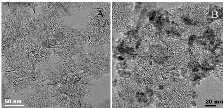
**Figure 1.** TEM images of (A) SWNHs and (B) SnO<sub>2</sub>/SWNH composites
