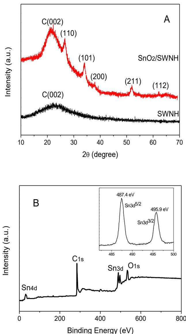
**Figure 2.** (A) X-ray diffraction (XRD) patterns of the pristine SWNHs and SnO<sub>2</sub>/SWNH composites, (B) XPS spectrum of the SnO<sub>2</sub>/SWNH and high-resolution XPS spectrum of Sn3d.
