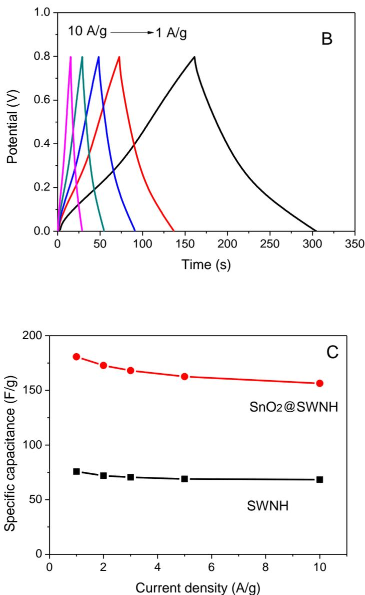
**Figure 4.** (A), (B) Galvanostatic charging/discharging (GCD) curves of SWNHs and SnO<sub>2</sub>/SWNH composites at different current densities, respectively. (C) Variation of the specific capacitance with different current density for SnO<sub>2</sub>/SWNH composites.
