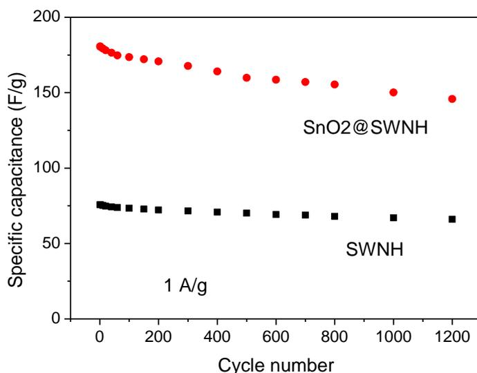
**Figure 5.** Cycle performance of SWNHs and SnO<sub>2</sub>/SWNH composites at 1 A/g
