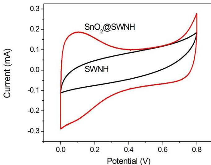
**Figure 3.** Cyclic voltammograms (CVs) for the second cycle of the SWNH and SnO<sub>2</sub>/SWNH composite electrodes at 20mV/s.
