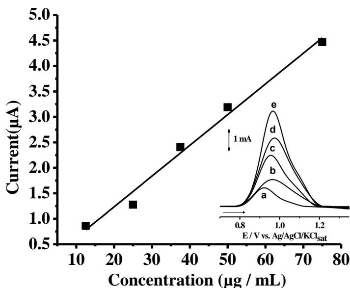
**Figure 6.** Calibration curve obtained from DPV assay with increasing concentrations of hibalactone (a: 12.5; b: 25; c: 37.5; d: 50 and e: 75 µg/mL). Inset. The related DP voltammograms.
