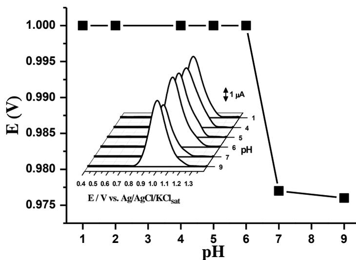
**Figure 4.** Plot of peak potential versus PBS pH value. Inset: Differential pulse voltammograms of hibalactone isolated from *H. umbellata* in different pH values of 0.1 M PBS. Pulse amplitude = 50 mV and Scan rate = 10 mV.s<sup>-1</sup>.
