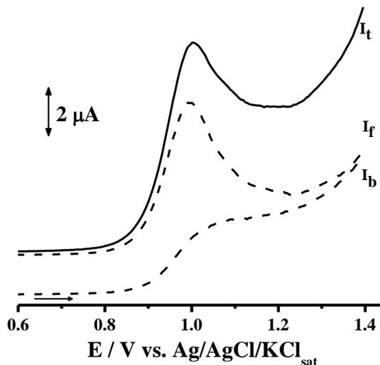
**Figure 3.** Square wave voltammetry calculated for hibalactone isolated from *H. umbellata* at CGE in 0.1 M PBS pH 6.0 ( $I_t$  = Total current;  $I_f$  = Forward current;  $I_b$  = Backward current). Pulse frequency = 30 Hz, scan rate =  $100\text{mV}\cdot\text{s}^{-1}$ , pulse amplitude = 50 mV.
