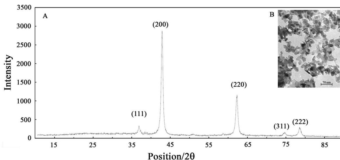
**Figure 1.** A) A typical XRD for MgO nanoparticles synthesized in this work. B) TEM image of MgO/NPs.
