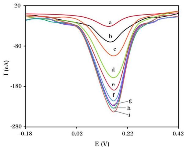
**Figure 3.** (A) DPVs of the accumulated  $\beta$ -CD on the surface of the dsDNA/SAM prepared with varying concentrations of  $\beta$ -CD. (a) to (i) represent  $\beta$ -CD concentrations from 0.015 to 0.135 mM.
