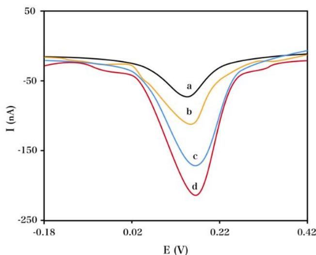
**Figure 1.** (A) DPVs of the accumulated  $\beta\text{-CD}$  on the surface of ssDNA/AuE before (voltammograms a and b) and after hybridization with the complementary DNA (voltammograms c and d) using the electrodes fabricated by the droplet self-assembly technique (voltammograms b and d) and the solution self-assembly technique (voltammograms a and c).
