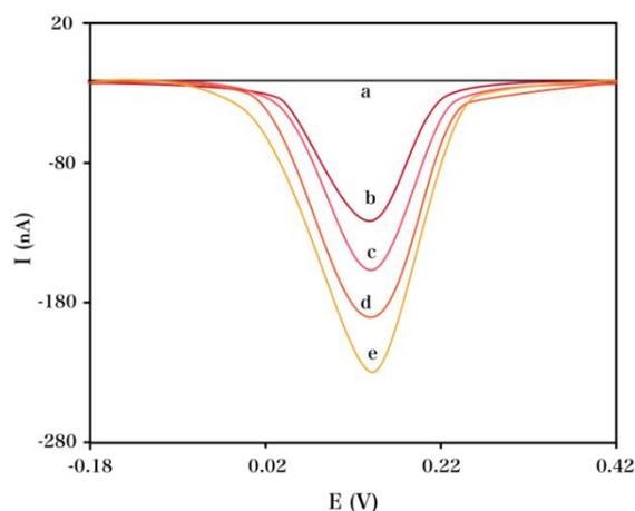
**Figure 4.** DPVs of the accumulated  $\beta$ -CD on the (a) MCH-decorated AuE and ssDNA-decorated AuE before (b) and after hybridization with oligonucleotide solutions ( $2 \mu\text{M}$ ) of the (c) non-complementary, (d) mismatched, and (e) complementary sequences in phosphate buffer solution ( $0.1 \text{ M}$ ,  $\text{pH } 7.0$ ).
