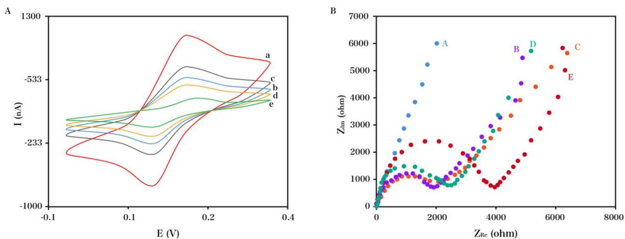
**Figure 5.** (A) CVs of the decorated electrode in a  $K_3[Fe(CN)_6]$  solution (1.0 mM) after each electrode modification step: (a) original AuE, (b) ssDNA-decorated AuE, (c) MCH/ssDNA-decorated AuE, (d) mismatched target DNA, and (e) target DNA. (B) Nyquist plots of the various electrodes in 5.0 mM  $K_3[Fe(CN)_6]/K_4[Fe(CN)_6]$  + 1.0 M KCl: (a) original AuE, (b) ssDNA-decorated AuE, (c) MCH/ssDNA-decorated AuE, (d) mismatched target DNA, and (e) target DNA.
