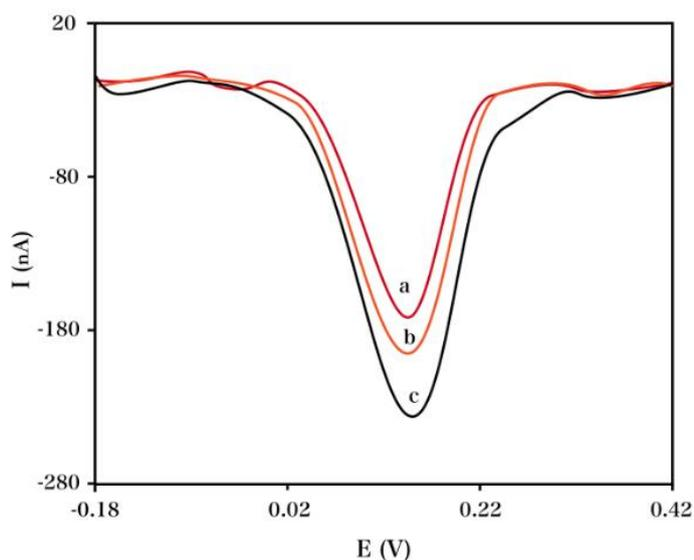
**Figure 2.** DPVs of the accumulated  $\beta$ -CD on the surface of the dsDNA/SAM prepared using varying hybridization techniques, including (a) drop, (b) preheated solution and (c) solution hybridization.
