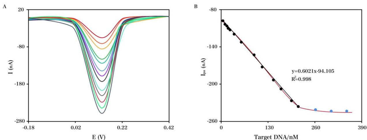
**Figure 6.** (A) DPVs of the accumulated  $\beta$ -CD on the hybridized ssDNA-decorated AuE with varying concentrations of the complementary (target) DNA in PBS (0.1 M, pH 7.0). (B) Inset: plot of the variation in the accumulated current response for the dsDNA-decorated AuE and ssDNA/SAM vs. the concentration of target DNA during hybridization.
