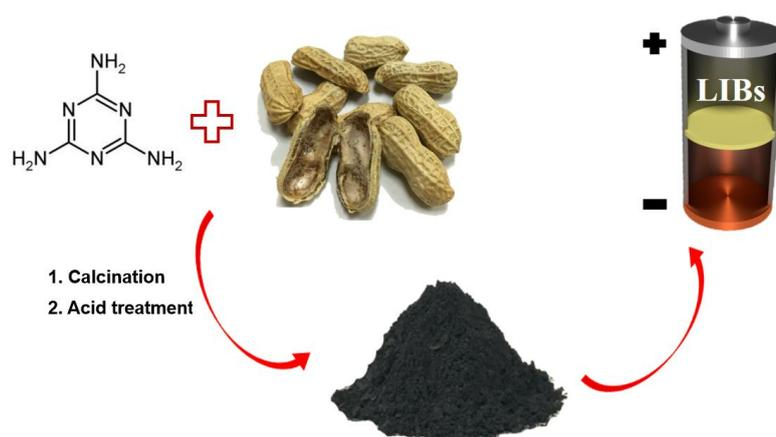
**Figure 1.** Schematic illustration for synthesis of N-doped carbon materials derived from peanut shells.
