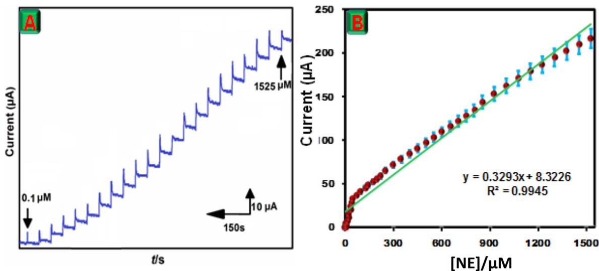
**Figure 5.** (A) Amperometric  $i-t$  response of sponge-like  $\text{Co}_3\text{O}_4$  particles modified electrode upon each addition of 0.1  $\mu\text{M}$ , 0.3  $\mu\text{M}$ , 1  $\mu\text{M}$ , 10  $\mu\text{M}$ , 30  $\mu\text{M}$ , 50  $\mu\text{M}$  and 75  $\mu\text{M}$  NE into the continuously stirred PBS (pH 7) at the rotation speed of 1200 rpm.  $E_{\text{app}} = +0.24 \text{ V}$ . (B) Plot of  $[\text{NE}]$ ,  $\mu\text{M}$  vs. peak current,  $\mu\text{A}$ .
