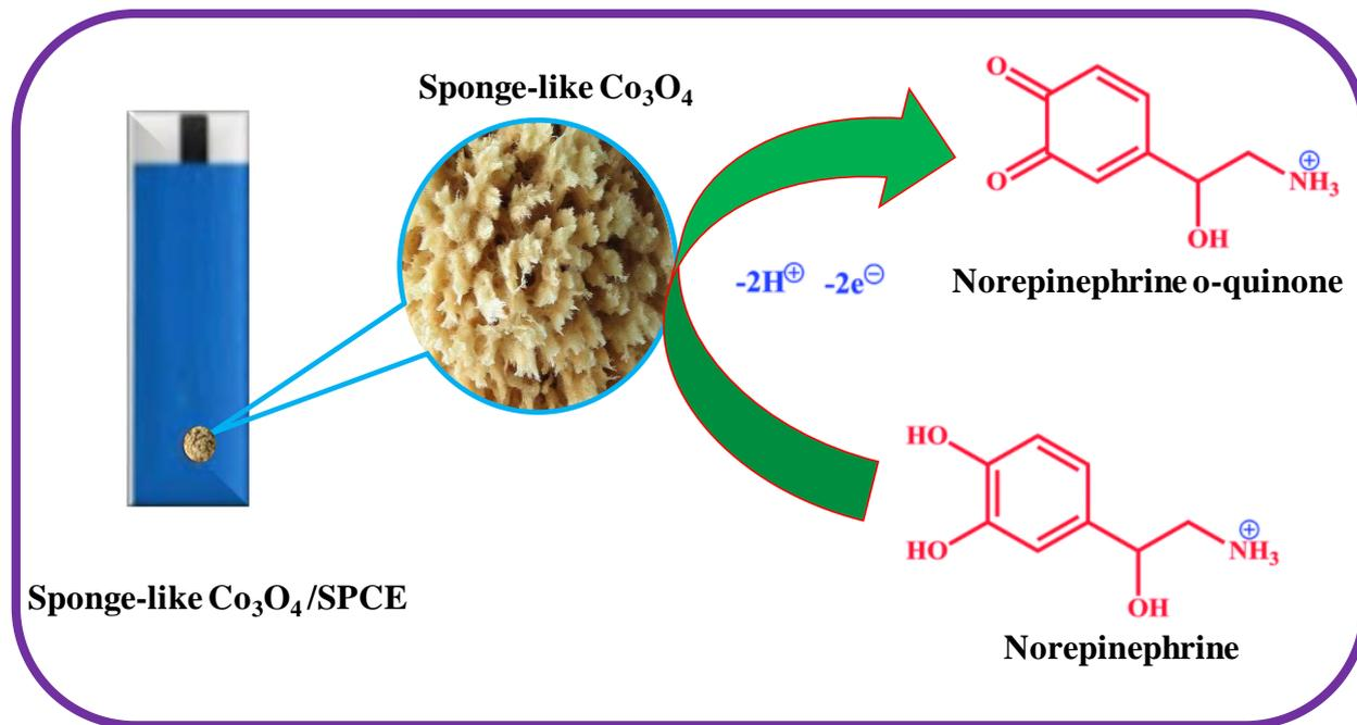
**Scheme 1** Schematic Representation for Electrochemical Detection of Norepinephrine using sponge-like  $\text{Co}_3\text{O}_4$  modified screen printed carbon electrode
