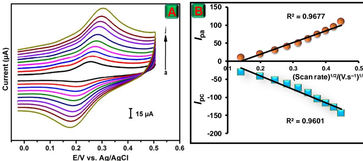
**Figure 4.** (A) Effect of the kinetics study on the cyclic voltammogram of 50  $\mu\text{M}$  NE at the sponge-like  $\text{Co}_3\text{O}_4$  particles/SPCE at 0.01 to 100  $\text{V s}^{-1}$  and (B) Plot for  $(\text{scan rate})^{1/2}$ ,  $\text{V.s}^{-1}$  vs. peak current,  $\mu\text{A}$ .
