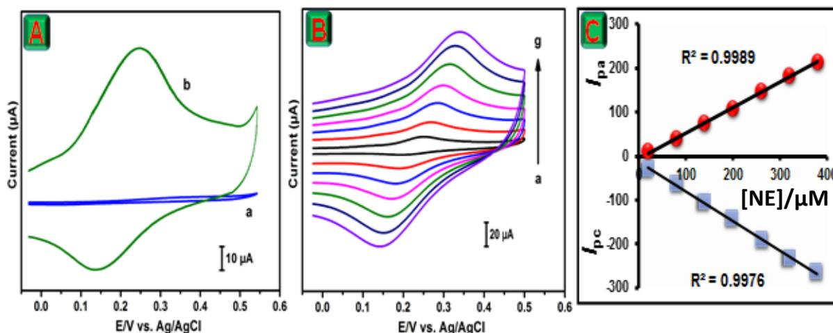
**Figure 3.** (A) Cyclic voltammogram shown at (a) bare SPCE, (b) sponge-like  $\text{Co}_3\text{O}_4$  particles/SPCE in  $0.05\text{M}$  phosphate buffer (pH 7) containing  $50 \mu\text{M}$  NE at the scan rate of  $50 \text{ mV s}^{-1}$ . (B) Cyclic voltammogram obtained at  $\text{Co}_3\text{O}_4$ /SPCE with different concentration of NE ( $50$  to  $350 \mu\text{M}$ ) using  $0.05\text{M}$  PBS (pH 7.0). (C) Plot of Peak Current vs. [NE]
