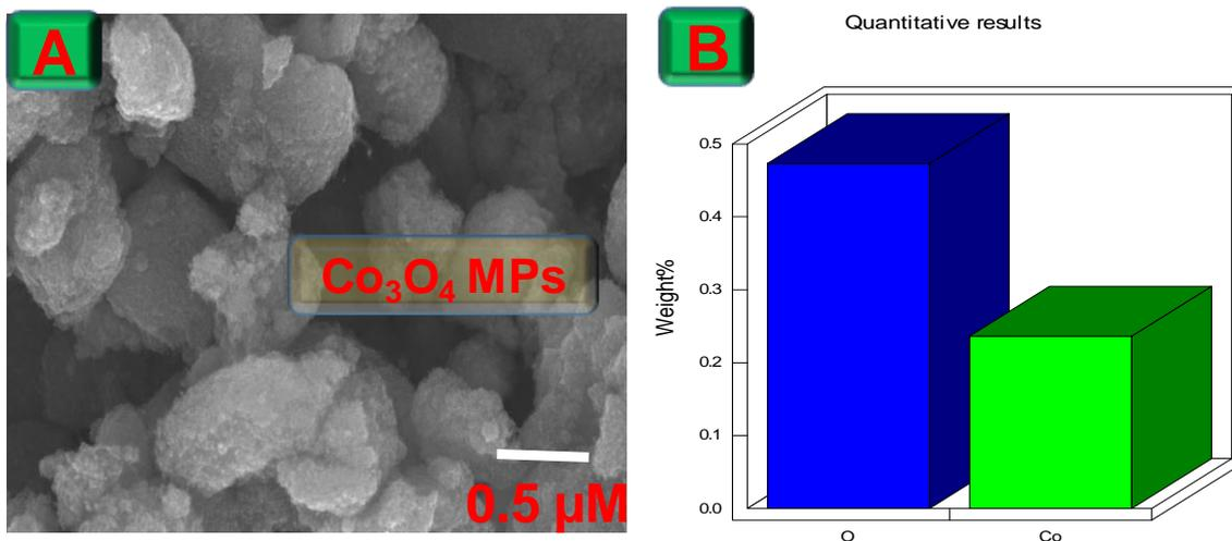
**Figure 1.** A) SEM image of sponge-like  $\text{Co}_3\text{O}_4$  Particles, B) Elemental Weight Percentage from EDX spectrum.
