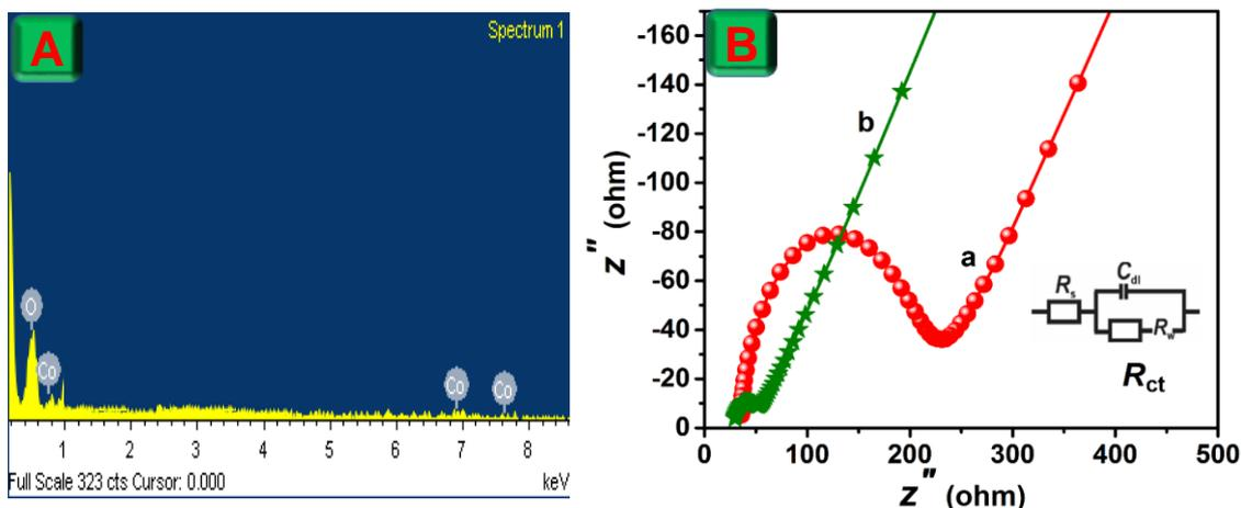
**Figure 2.** A) EDX spectrum of sponge-like  $\text{Co}_3\text{O}_4$  particles, B) EIS curves of unmodified SPCE (a), sponge-like  $\text{Co}_3\text{O}_4$  particles/SPCE (b) in 0.1 M KCl containing 5 mM  $[\text{Fe}(\text{CN})_6]^{3-/4-}$  solution.
