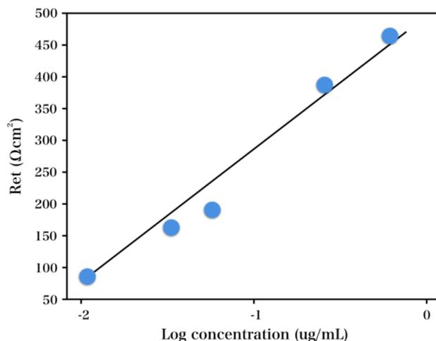
**Figure 5.** Calibration curve of the logarithm of testosterone concentration against the Ret collected from Ab-testosterone/Au(MPA)/APTES/ITO glass.
