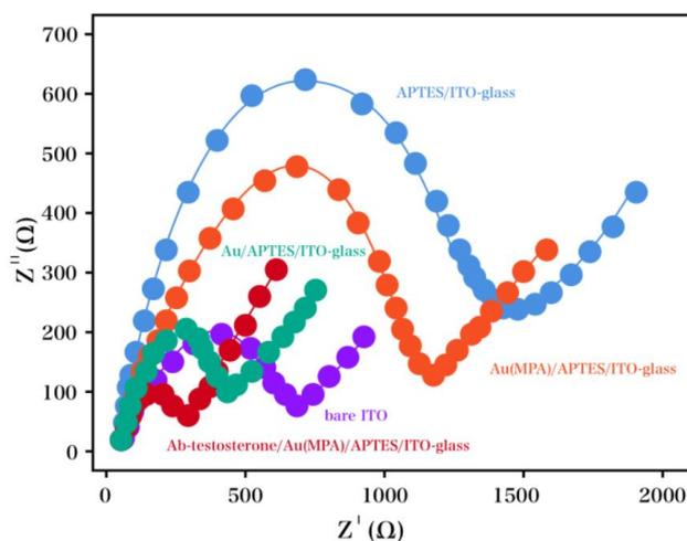
**Figure 3.** Nyquist plots at the bare ITO glass plate, APTES/ITO glass, Au(MPA)/APTES/ITO glass, Au/APTES/ITO glass and Ab-testosterone/Au(MPA)/APTES/ITO glass in pH 7.4 PBS (0.1 M KCl) + 2 mM  $[\text{Fe}(\text{CN})_6]^{3-/4-}$ .
