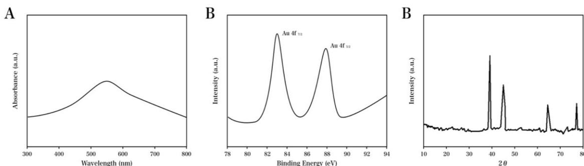
**Figure 1.** (A) UV-vis spectrum, (B) High resolution Au 4f scan and (C) XRD pattern of biosynthesized Au nanoparticles.
