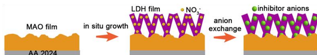
Figure 2. The schematic of growth process of the MAO/LDHs composite film.
