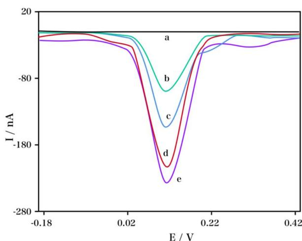
**Figure 4.** DPV curves of the  $\beta$ -CD accumulated on the (a) MCH coated AuE, ss-DNA-coated AuE before (b) and after hybridization with oligonucleotide solution (2  $\mu$ M) of the (c) non-complementary, (d) mismatched, and (e) complementary in 0.1 M of phosphate buffer solution (pH 7.0).
