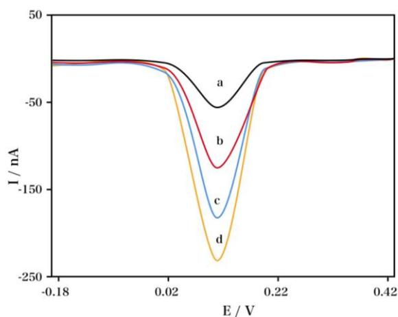
**Figure 1.** (A) DPV curves for the  $\beta$ -CD accumulated on the ss-DNA-modified AuE surface (a,b) before and (c,d) after hybridization with the complementary DNA using the AuE fabricated via different techniques: droplet self-assembly (b,d) and solution self-assembly (a,c).
