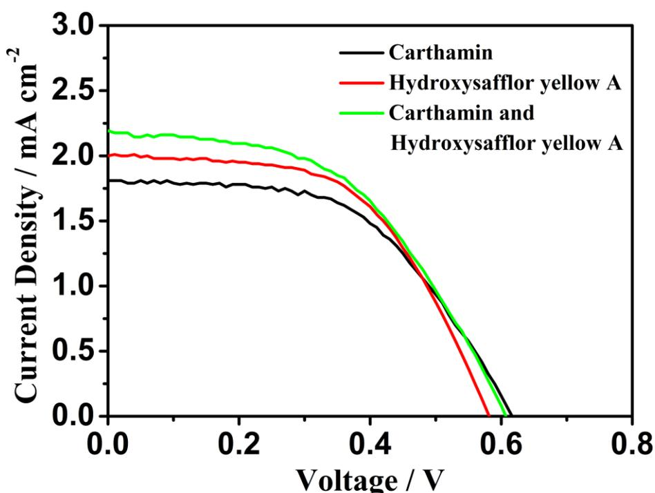
**Figure 5.**  $I$ - $V$  characteristic curves of different DSSC.
