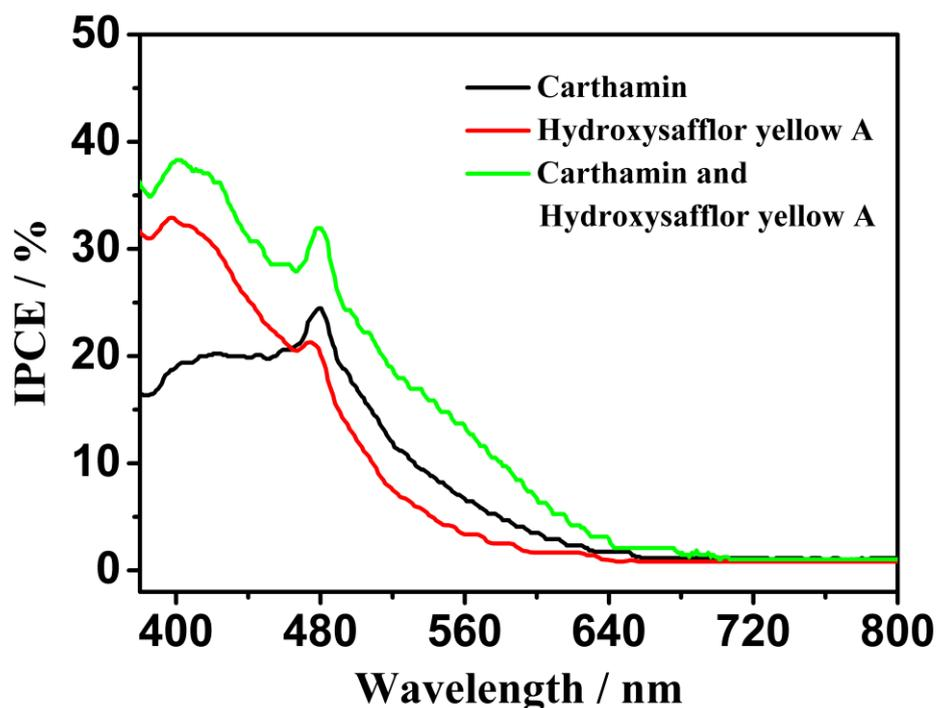
**Figure 6.** IPCE spectra of DSSCs based on different samples.
