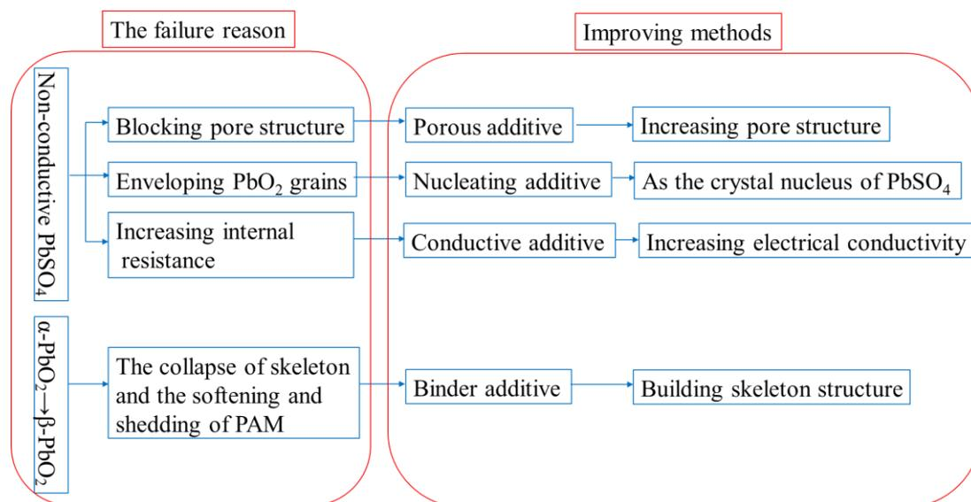
**Figure 1.** The failure reasons and improving methods of the battery.
