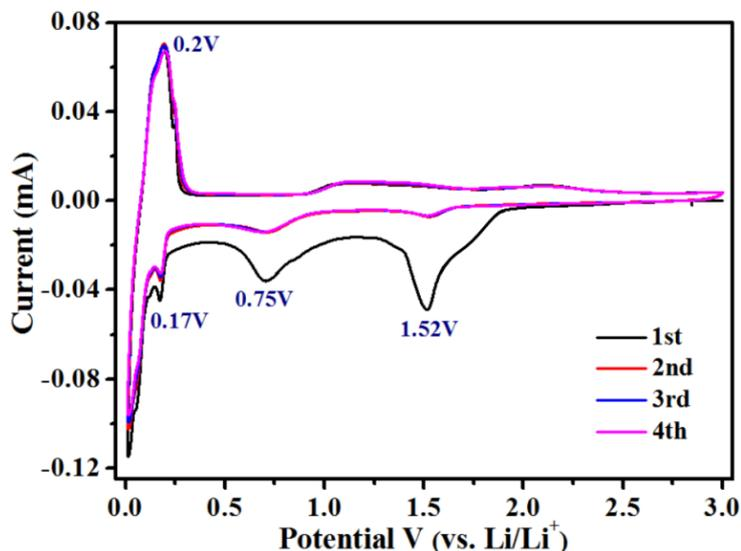
**Figure 2.** Cycle voltammetry profiles of 1/2.25-FePc/GN composite.
