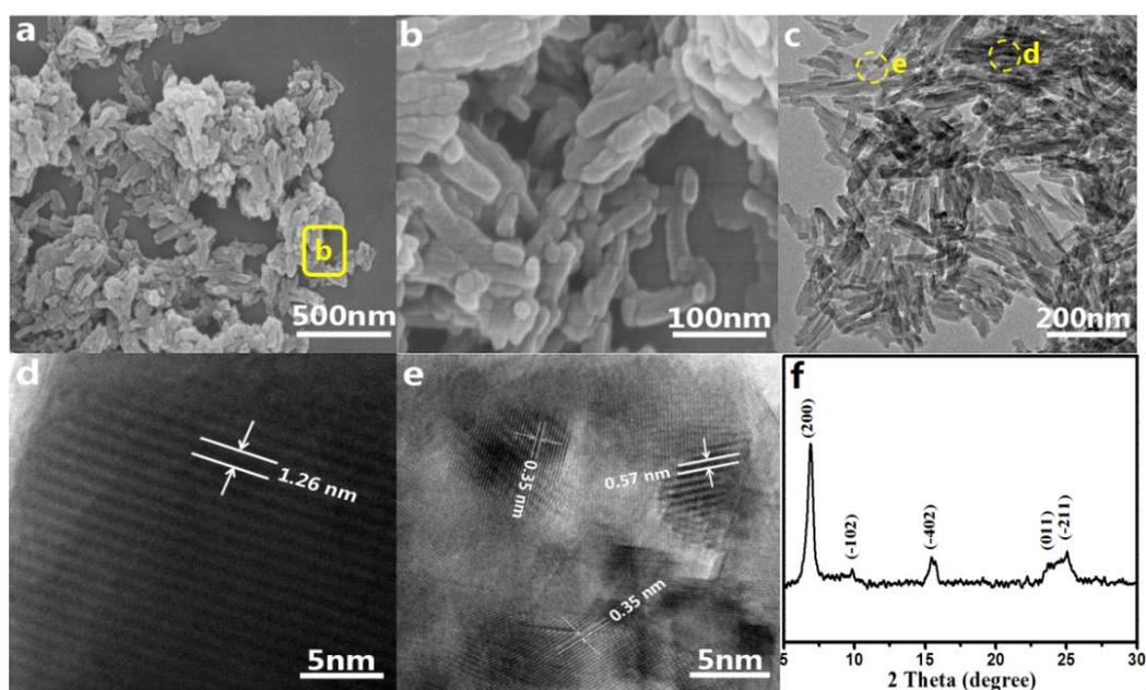
**Figure 1.** SEM and TEM images and X-ray pattern of the iron-phthalocyanine powder: low (a) and high (b) magnification SEM images; TEM (c) and HR-TEM (d, e) images; X-ray diffraction pattern (f).
