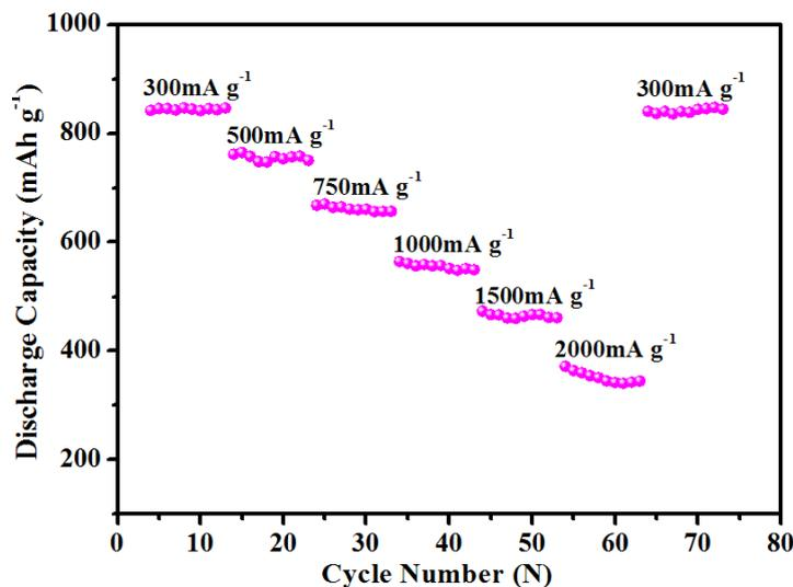
**Figure 5.** Cycling performance of 1/2.25-FePc/GN composite at various current densities between 300 and 2000 mA g<sup>-1</sup>.
