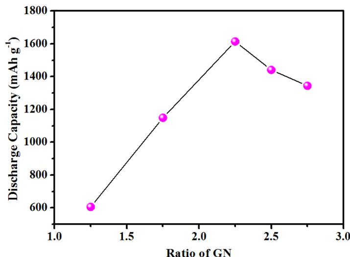
**Figure 6.** The specific capacity based on FePc at different weight ratios in the composites.
