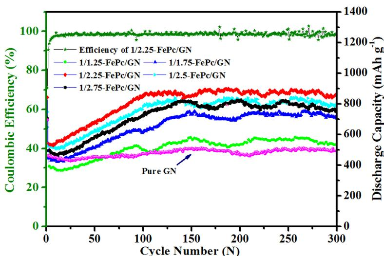
**Figure 4.** Cycle performance of FePc/GN in different weight ratios and pure GN at a current density of 300 mA g<sup>-1</sup>.
