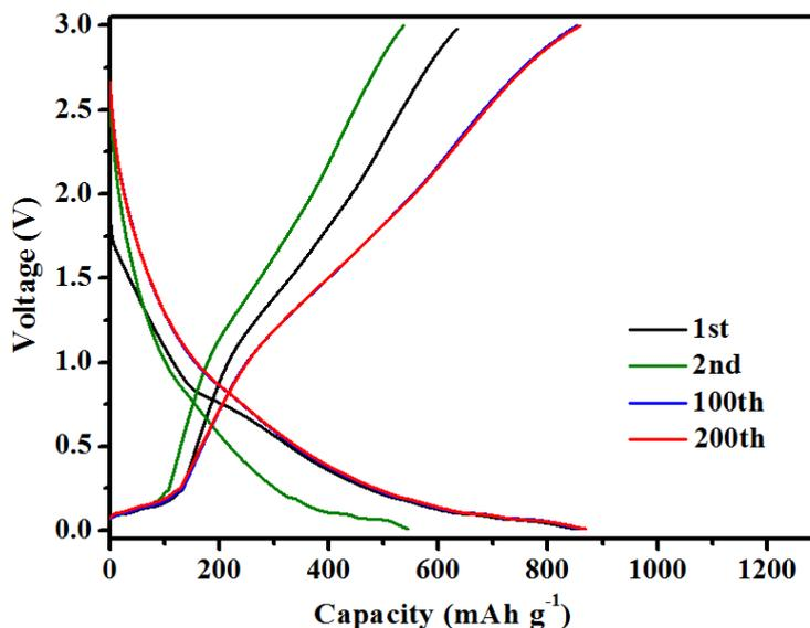
**Figure 3.** Charge and discharge curves at the 1<sup>st</sup>, 2<sup>nd</sup>, 100<sup>th</sup>, 200<sup>th</sup> cycles of 1/2.25-FePc/GN composite at a current density of 300 mA g<sup>-1</sup>.
