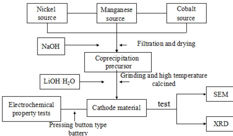
**Figure 1.** Preparation process flow diagram of co-precipitation method
