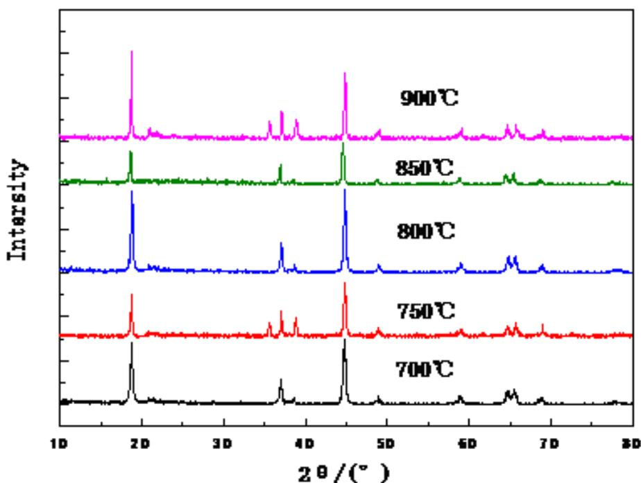
**Figure 2.** XRD patterns of samples prepared at different temperatures of calcine time for 8h
