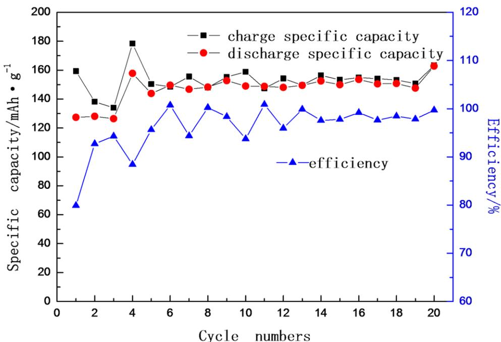
Figure 6. Cycle performance of charge-discharge curves at 0.1C rate
