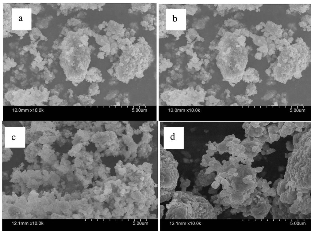
**Figure 3.** The SEM graphs of samples prepared at different temperatures (a=700°C; b=750°C; c=800°C; d=850°C)
