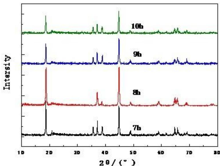
**Figure 4.** XRD patterns of samples prepared at different time of calcine temperature for 800°C
