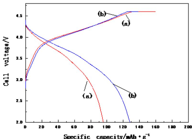
**Figure 5.** The first(a) and second(b) charge-discharge curves at 0.1C rate
