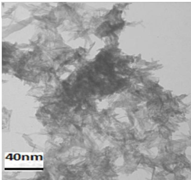
**Figure 3.** TEM image of CuO nanoparticles
