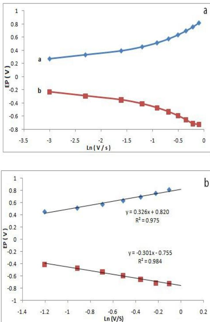
**Figure 6.** (a) The relationship between cathodic and anodic peaks potentials with natural logarithm of scan rates. (b) The linear dependence of the peak potentials vs natural logarithm of scan rates.
