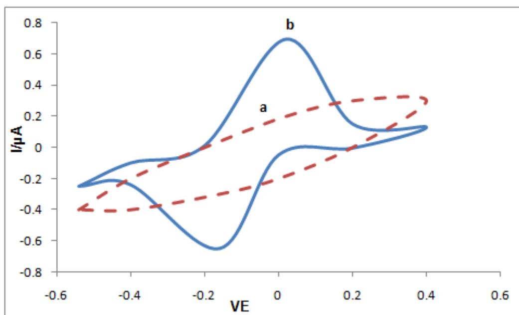
**Figure 4.** Cvs of Hb/CPE (a) and Hb/CuO/CPE (b) in 0.1 M PBS (pH=7) at a scan rate of 700 mV s<sup>-1</sup>
