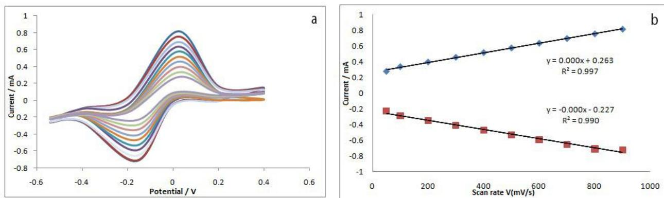
**Figure 5.** (a) CVs of Hb/CuO/CPE in  $0.1 \text{ M PBS}$  at different scan rates, from inner to outer:  $50, 100, 200, 300, 400, 500, 600, 700, 800, 900, 1000 \text{ mV s}^{-1}$ . (b) Plots of peaks currents vs scan rates.
