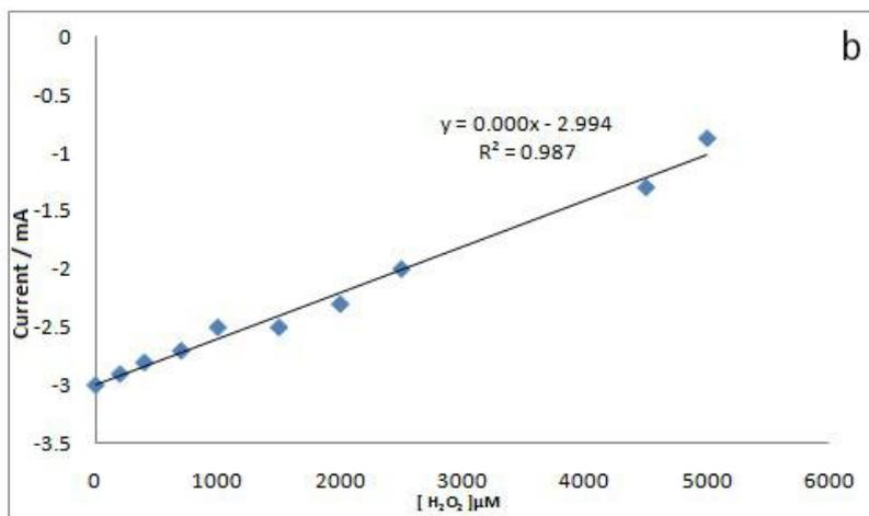
**Figure 8.** (a) CVs of Hb/CuO/CPE in 0.1M PBS (pH=7) at different concentrations of H<sub>2</sub>O<sub>2</sub> (0 to 5000). (b) Plot of cathodic peak currents vs scan rate H<sub>2</sub>O<sub>2</sub> concentrations from 0 to 4500 ( at 100 mV s<sup>-1</sup>)
