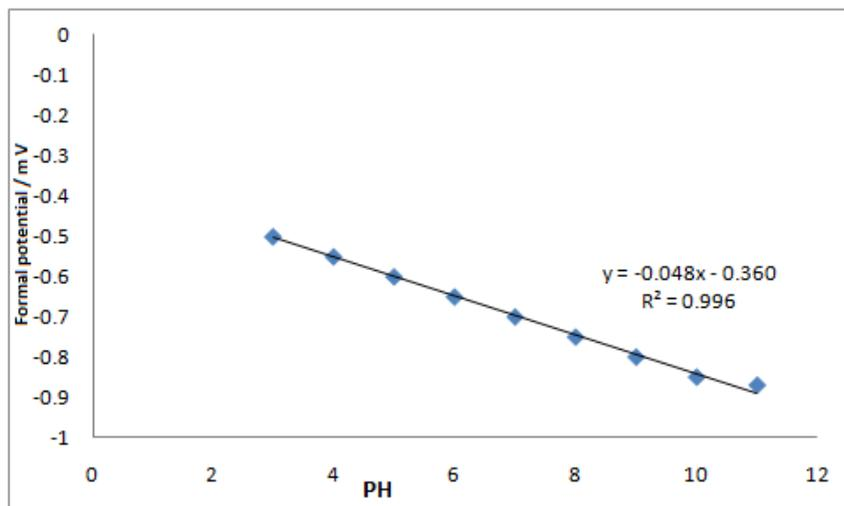
**Figure 7.** Effect of pH on formal potential of Hb/CuO/CPE in 0.1M PBS (pH=7) at 700 mV s<sup>-1</sup> scan rate.
