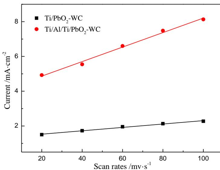
**Figure 8.** Plots of the current density at 1.60 V vs. the scan rate.
