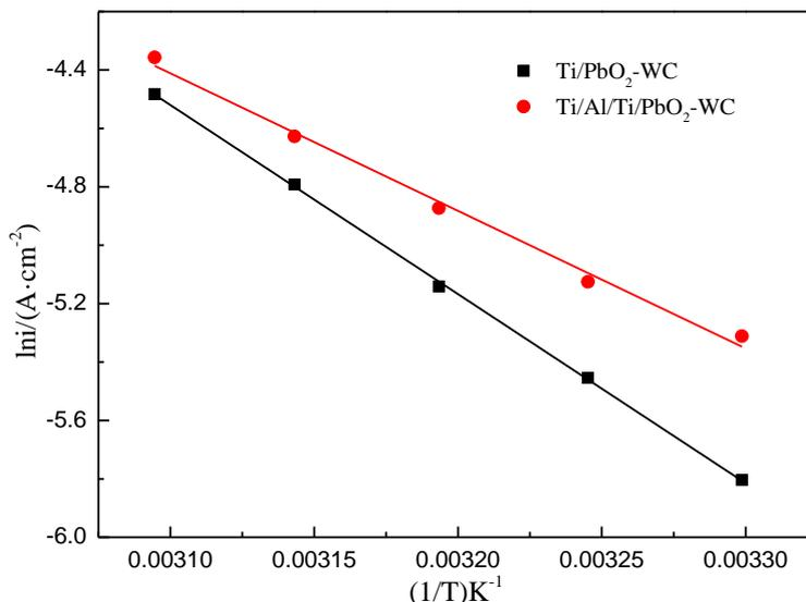
**Figure 6.** Arrhenius plots of the two composite electrodes
