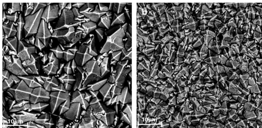
**Figure 1.** Surface morphology of (a)Ti/PbO<sub>2</sub>-WC composite electrode and (b)Ti/Al/Ti/PbO<sub>2</sub>-WC composite electrode.
