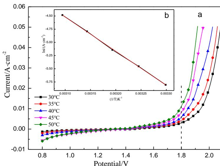
**Figure 5.** a. Ti/PbO<sub>2</sub>-WC composite electrode polarization curves at different electrolyte temperatures; b.  $\ln i - T^{-1}$  linear fitting curve
