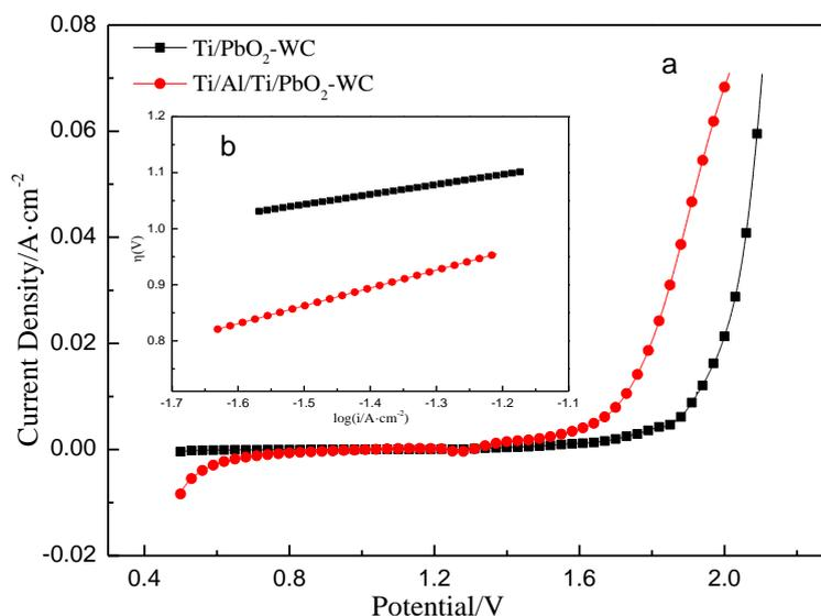
**Figure 4.** Anode polarization curves and Tafel linear fitting curves of  $\text{Ti/PbO}_2\text{-WC}$  composite electrode and  $\text{Ti/Al/Ti/PbO}_2\text{-WC}$  composite electrode.
