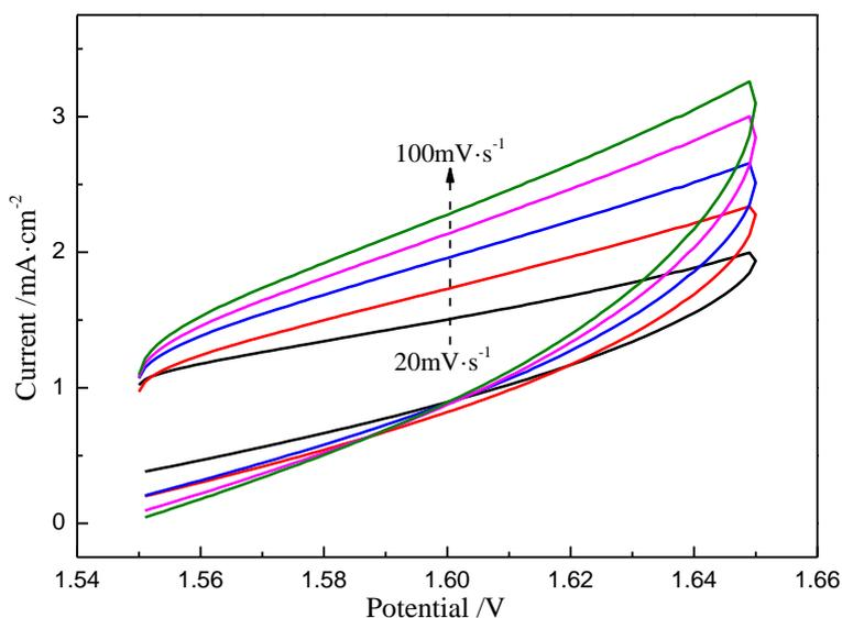
**Figure 7.** Voltammetric curves of the Ti/PbO<sub>2</sub>-WC composite electrode at different scan rates in the capacitive potential region (1.55-1.65 V)
