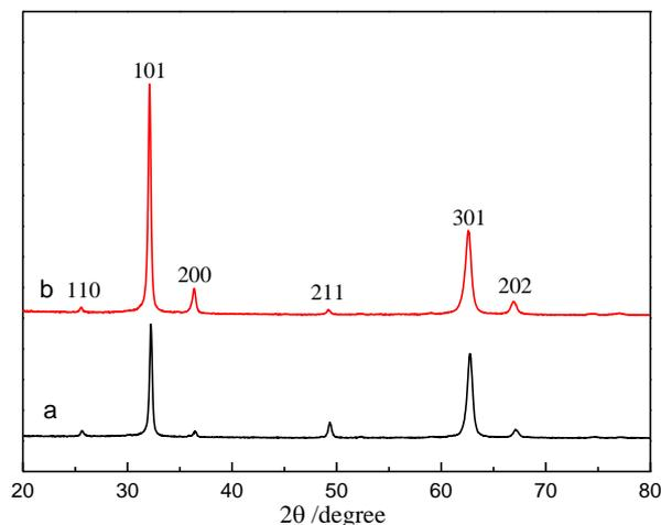
**Figure 3.** XRD patterns of (a)Ti/PbO<sub>2</sub>-WC composite electrodes and (b)Ti/Al/Ti/PbO<sub>2</sub>-WC composite electrodes.
