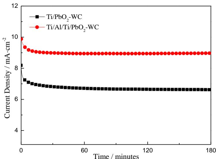
**Figure 9.** Chronoamperometric curves obtained on the two composite electrodes in the synthetic zinc electroplating electrolyte
