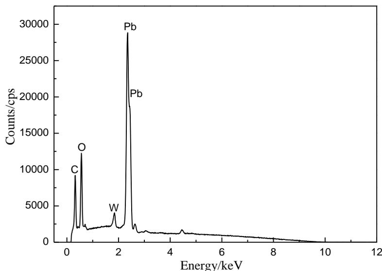
**Figure 2.** Energy spectrogram analysis results using mapping scanning for the Ti/Al/Ti/PbO<sub>2</sub>-WC composite electrode
