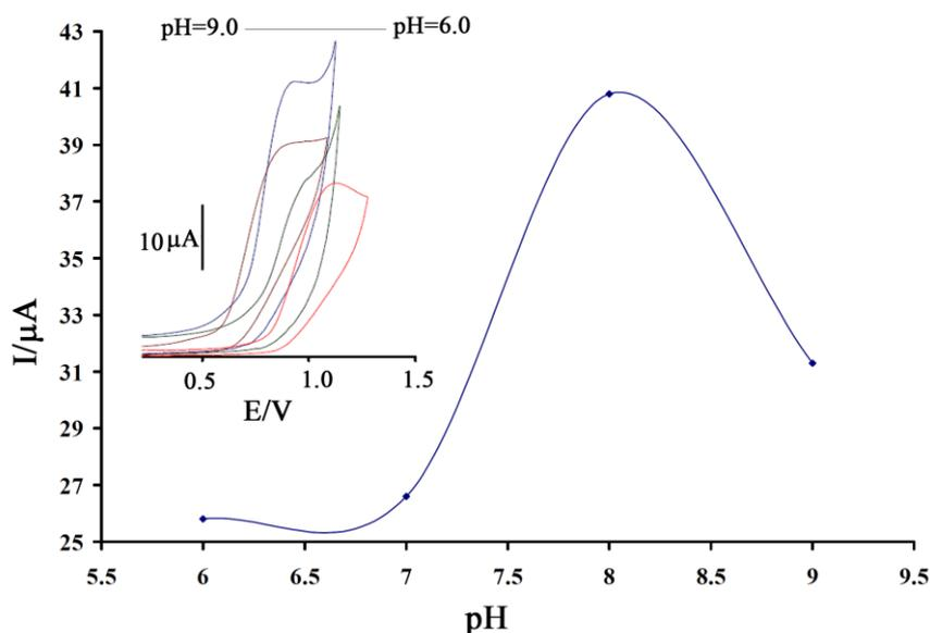
**Figure 2.** The current-pH curve for electro-oxidation of 500  $\mu\text{M}$  tramadol at a surface of 1,3-DI-Br/MgO/SWCNTs/CPE in the pH range 6.0-9.0. Insert) cyclic voltammograms of 500.0  $\mu\text{M}$  tramadol at a surface of 1,3-DI-Br/MgO/SWCNTs/CPE in the pH range 6.0-9.0
