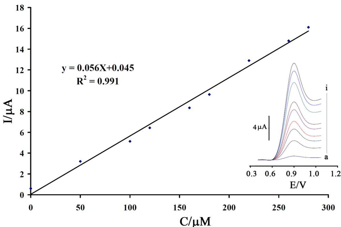
**Figure 7.** The linear relation between current and tramadol concentration. Insert) square wave voltammograms of 1,3-DI-Br/MgO/SWCNTs/CPE in the presence of a) 0.05, b) 50.0, c) 100.0, d) 120.0, e) 160.0, f) 180.0, g) 220.0, h) 260.0 and i) 280 μM tramadol.
