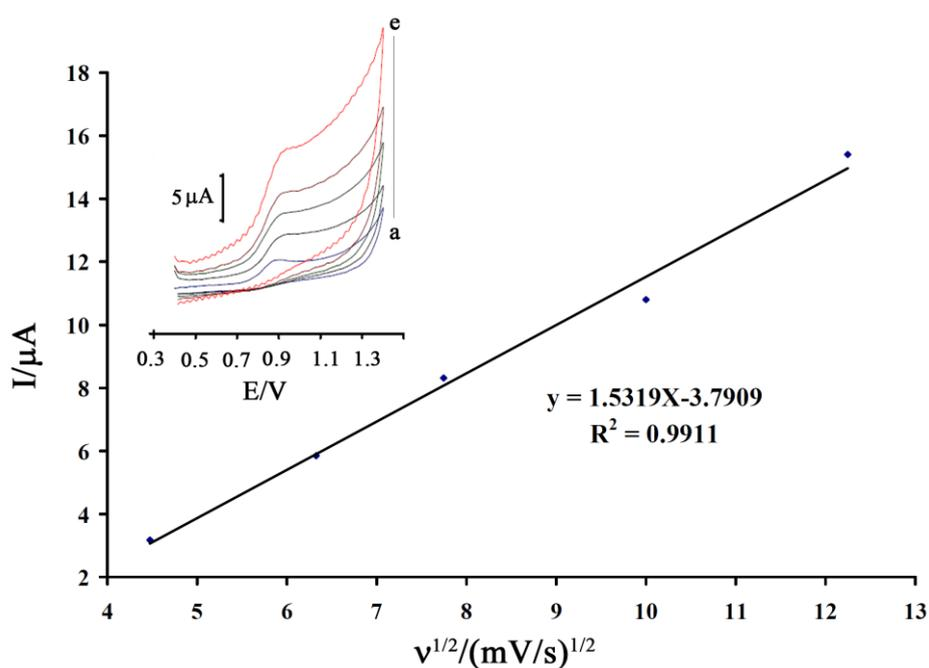
**Figure 4.** Cyclic voltammograms of 100.0 μM of tramadol at a surface of 1,3-DI-Br/MgO/SWCNTs/CPE at scan rate a) 20.0; b) 40.0; c) 60.0; d) 100.0 and e) 150 mV/s.
