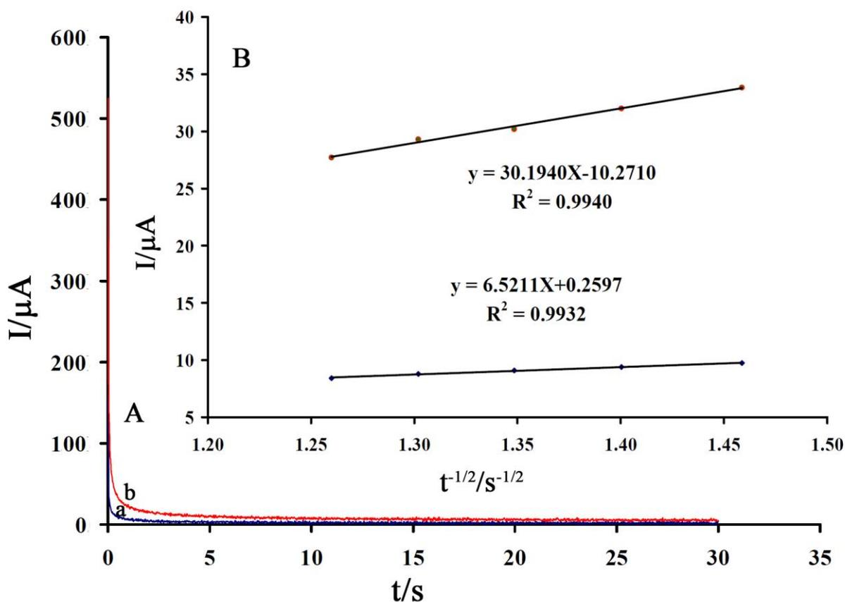
**Figure 5.** A) Chronoamperograms obtained at the 1,3-DI-Br/MgO/SWCNTs/CPE in the presence of (a) 300 and (b) 500  $\mu\text{M}$  tramadol. B) Plots of  $I$  vs.  $t^{-1/2}$  obtained from chronoamperometry.
