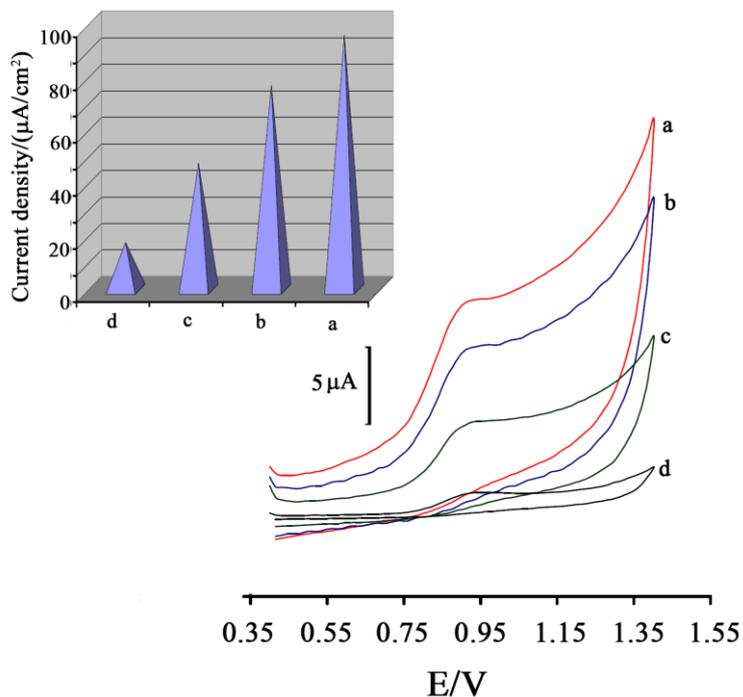
**Figure 3.** Cyclic voltammograms of 150.0 μM of tramadol at a surface of 1,3-DI-Br/MgO/SWCNTs/CPE (curve a), 1,3-DI-Br/CPE (curve b), MgO/SWCNTs/CPE (curve c) and CPE (curve d) in the pH=8.0. Insert) current density data obtained from cyclic voltammograms.
