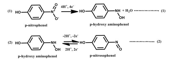
Scheme 2. Schematic representation of electron transfer processes involved in 4-NP at AgNDs/GCE
