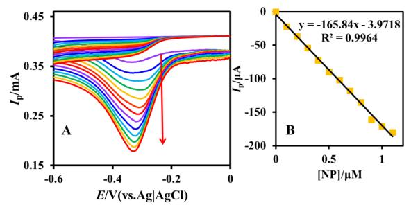
**Figure 4.** (A) CVs obtained at AgNDs/GCE in the absence (a) and presence (b-m) of NP (each addition of 0.25 mM) in 0.05 M PBS (pH 5) at the scan rate of 50 mV/s. (B) Calibration plot between [NP] and  $I_p$
