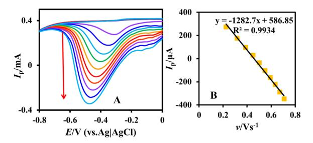
**Figure 5.** (A) CVs for varying scan rate (0.05 to 0.5 V/s) at AgNDs/GCE in 0.05 M PBS (pH 5) containing 1 mM NP. (B) Calibration plot for  $v^{1/2}$  vs  $I_p$
