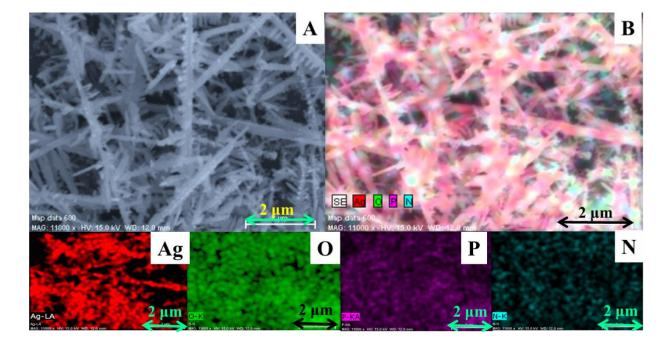
Figure 1. (A) SEM image of AgNDs. (B) Elemental mapping of AgNDs (Ag, O, P and N)
