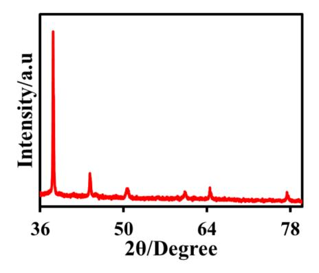
Figure 2. X-ray diffraction pattern of AgNDs
