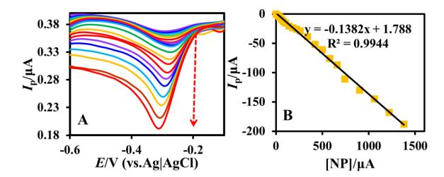
3.5 Electrochemical determination of NP: Linear sweep voltammetry (LSV)
