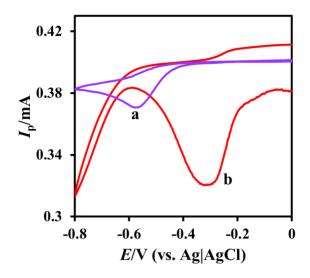
**Figure 3.** CVs observed at (a) unmodified and (b) AgNDs modified GCE in the presence of 1 mM hydrazine (electrolyte = 0.05 M PBS (pH 5))
