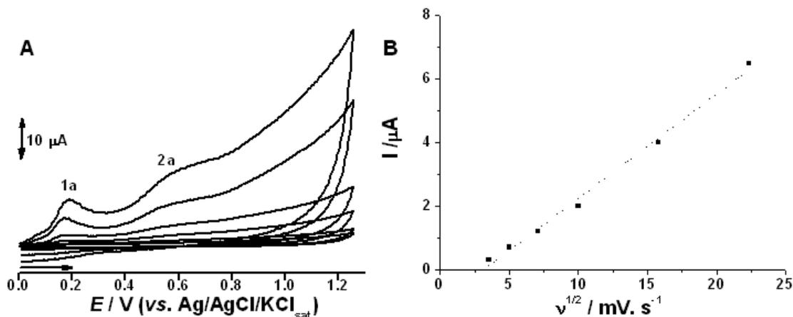
**Figure 1.** A. CV voltammograms of BT at different scan rates (500, 250, 100, 50, 25, 12.5 mVs<sup>-1</sup>) scan range from 0 to 1.3 V. B. Plot of peak current ( $I$ ) vs scan rate square root ( $v^{1/2}$ ) obtained from first anodic process (1a), determination coefficient ( $r^2$ ) = 0.983. All analysis carried out in 0.1 M PBS, pH 7.0 at GCE.
