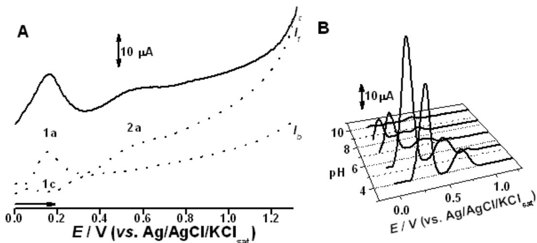
**Figure 2.** A. SW voltammograms of BT1. Pulse amplitude 50 mV, frequency of 50 Hz and a potential increment of 2 mV, corresponding to an effective scan rate ( $\nu$ ) of  $100 \text{ mVs}^{-1}$ . Analysis carried out in 0.1 M PBS, pH 7.0. B. DP voltammogram of BT samples at different pH (4.0, 5.5, 7.0, 8.5, 10.0). Pulse amplitude 50 mV, pulse width 0.5 s and scan rate  $10 \text{ mVs}^{-1}$ . Analysis carried out in 0.1 M PBS, at aforementioned pH at GCE.
