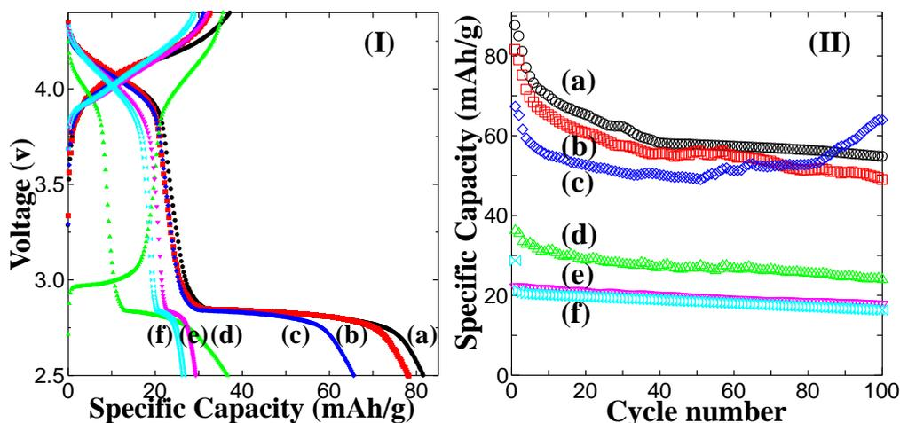
**Figure 4.** Galvanostatic charge/discharge curves (I) and cyclic performance at a rate of 1 C (II) of Ti-doped  $\text{Li}_4\text{Mn}_{5-x}\text{Ti}_x\text{O}_{12}$  cathode material: (a)  $x=0$ , (b)  $x=0.05$ , (c)  $x=0.1$ , (d)  $x=1$ , (e)  $x=2$ , (f)  $x=2.5$ , respectively.
