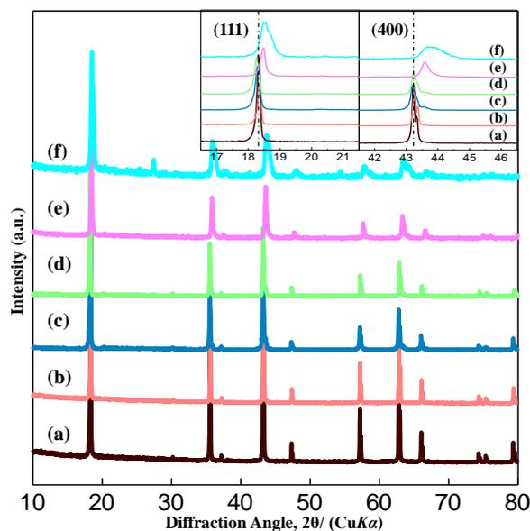
**Figure 2.** XRD patterns of Mn-doped  $Li_4Mn_{5-x}Ti_xO_{12}$  anode material, which annealed at 800 °C for 10 h: (a)  $x=5$ , (b)  $x=4.95$ , (c)  $x=4.9$ , (d)  $x=4$ , (e)  $x=3$ , (f)  $x=2.5$ , respectively.
