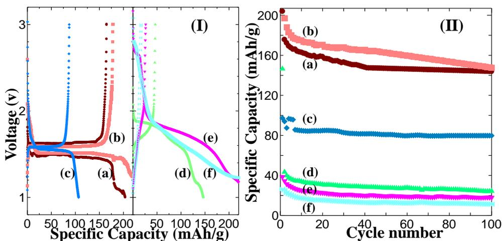
**Figure 5.** Galvanostatic curves (I) and cyclic performance at a rate of 1C (II) of Mn-doped  $\text{Li}_4\text{Mn}_{5-x}\text{Ti}_x\text{O}_{12}$  anode material: (a)  $x=5$ , (b)  $x=4.95$ , (c)  $x=4.9$ , (d)  $x=4$ , (e)  $x=3$ , (f)  $x=2.5$ , respectively.
