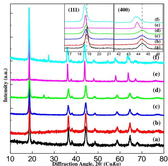
**Figure 1.** XRD patterns of Ti-doped  $\text{Li}_4\text{Mn}_{5-x}\text{Ti}_x\text{O}_{12}$  cathode material: (a)  $x=0$ , (b)  $x=0.05$ , (c)  $x=0.1$ , which annealed at 600 °C for 10 h; (d)  $x=1$ , (e)  $x=2$ , (f)  $x=2.5$ , which annealed at 800 °C for 10 h, respectively.
