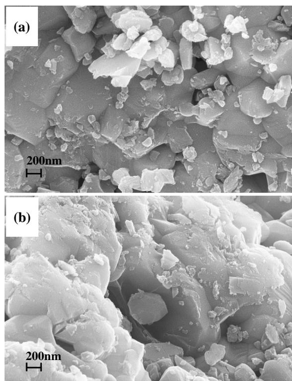
**Figure 3.** SEM images of (a)  $Li_4Mn_5O_{12}$  which annealed at 600 °C for 10 h and (b)  $Li_4Ti_5O_{12}$  which annealed at 800 °C for 10 h.
