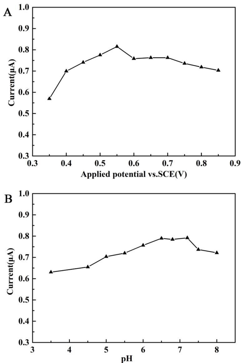
**Figure 4.** (A) Effects of applied potential on the response current of PANI-GRA/PtNPs/CS-GOD biosensor in 0.02 M phosphate buffer (pH 6.5) containing 0.5 mM glucose. (B) Effects of pH values on the response current of PANI-GRA/PtNPs/CS-GOD biosensor in different buffers containing 0.5 mM glucose.
