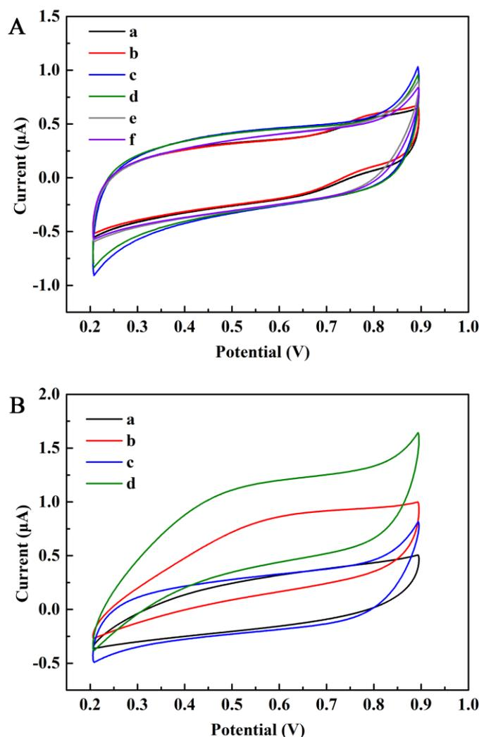
**Figure 3.** (A) CVs in 0.02 M phosphate buffer (pH 6.5) at 50 mV/s for (a) without glucose, and (b) with 0.5 mM glucose of Pt/PANI/PtNPs, (c) without glucose, and (d) with 0.5 mM glucose Pt/PANI-GRA/PtNPs, (e) without glucose, and (f) with 0.5 mM glucose Pt/PANI-GRA/PtNPs/CS. (B) CVs in 0.02 M phosphate buffer (pH 6.5) at 50 mV/s for (a) without glucose, and (b) with 0.5 mM glucose of Pt/PANI/ PtNPs/CS-GOD, (c) without glucose, and (d) with 0.5 mM glucose of Pt/PANI-GRA/PtNPs/CS-GOD.
