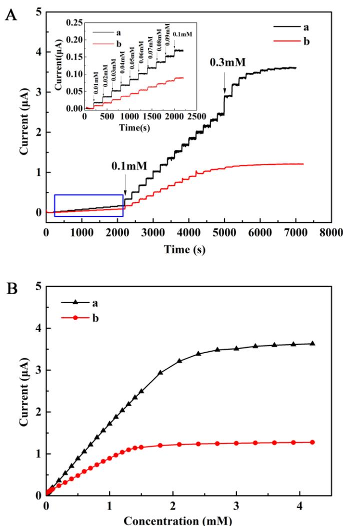
**Figure 5.** (A) Amperometric responses to successive injection of glucose at an applied potential of 0.55 V vs. SCE in 0.02 M phosphate buffer (pH 6.5) for (a) PANI-GRA-PtNPs/CS-GOD and (b) PANI/PtNPs/CS-GOD biosensors. Inset: the magnified part of the curve marked with blue square. (B) Current-Concentration curves of (a) PANI-GRA/PtNPs/CS-GOD and (b) PANI/PtNPs/CS-GOD biosensors.
