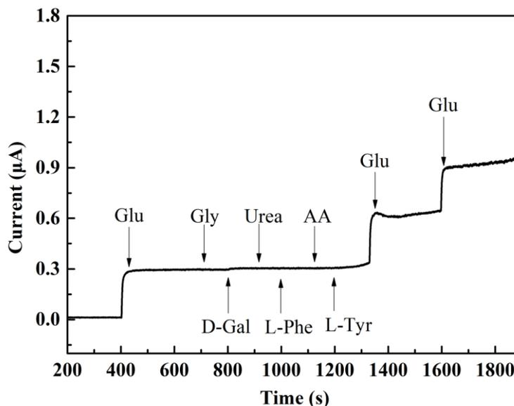
**Figure 6.** Effects of the interferences on the amperometric responses of the glucose biosensor in the presence of glucose.
