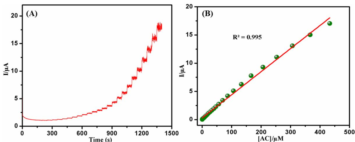
**Figure 3.** (A) Amperometric current response of different amount of AC at GO modified electrode, (B) calibration plot of  $I_{pa}$  vs [AC].
