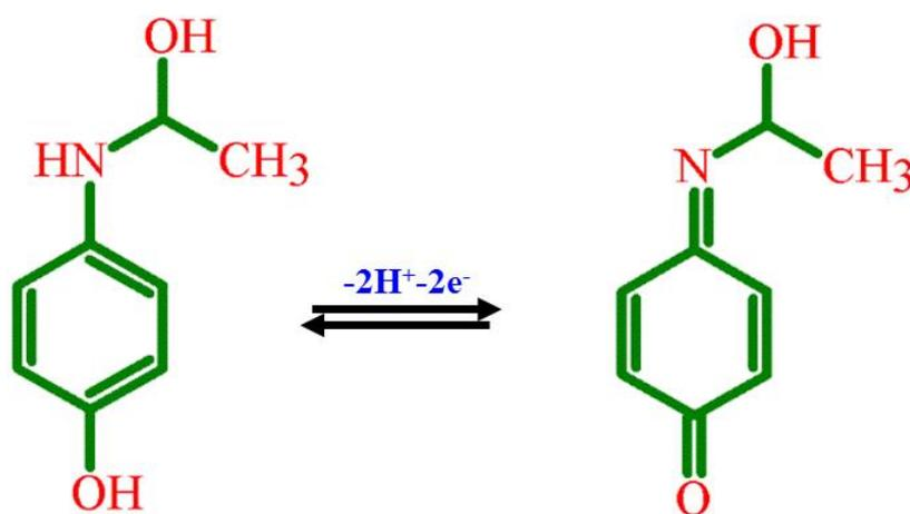
**Scheme 1.** Electrocatalytic oxidation mechanism of AC.
