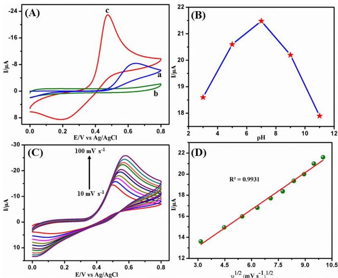
**Figure 2.** (A) CV of bare GCE (a), GO/GCE absence of AC (b), GO/GCE in the presence 500 μM AC (c) in 0.05 M PBS (pH 7.0) at a scan rate of 50 mVs<sup>-1</sup>. (B) Plot of oxidation peak current of AC vs. pH. (C) CV responses obtained from the GO/GCE in the presence of 500 μM AC in 0.05 M PBS (pH 7.0) at different scan rates from 10 to 100 mVs<sup>-1</sup> (D) I<sub>pa</sub> vs. square root of scan rate.
