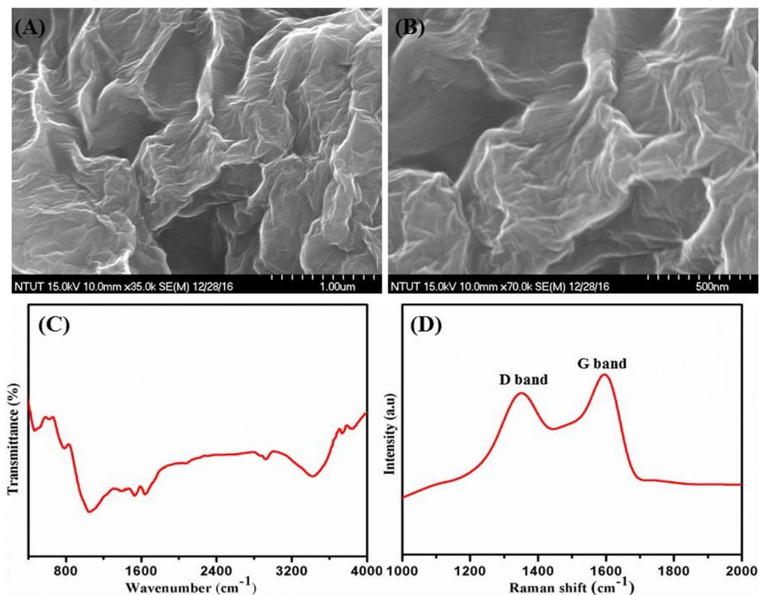
**Figure 1.** SEM images (A&B), FT-IR spectrum (C), Raman spectrum (D) of GO.
