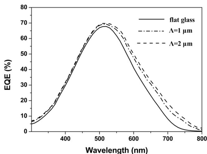
**Figure 6.** External quantum efficiency (EQE) spectra of three kind of n-i-p thin film silicon solar cells which were prepared on the flat, and patterned glass with  $\Lambda = 1$  and  $2 \mu\text{m}$
