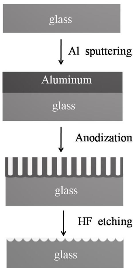
**Figure 1.** The schematic diagram of the entire experiment process.
