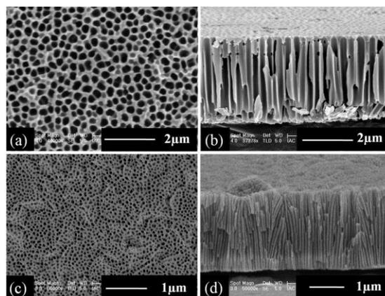
**Figure 2.** SEM images of porous anodic aluminum oxide which are fabricated on the glass substrate. (a) Top surface image and (b) cross section image of porous anodic aluminum oxide which were anodized in the phosphoric acid solution. (c) Top surface image and (d) cross image of porous anodic aluminum oxide which were anodized in the oxalic acid solution
