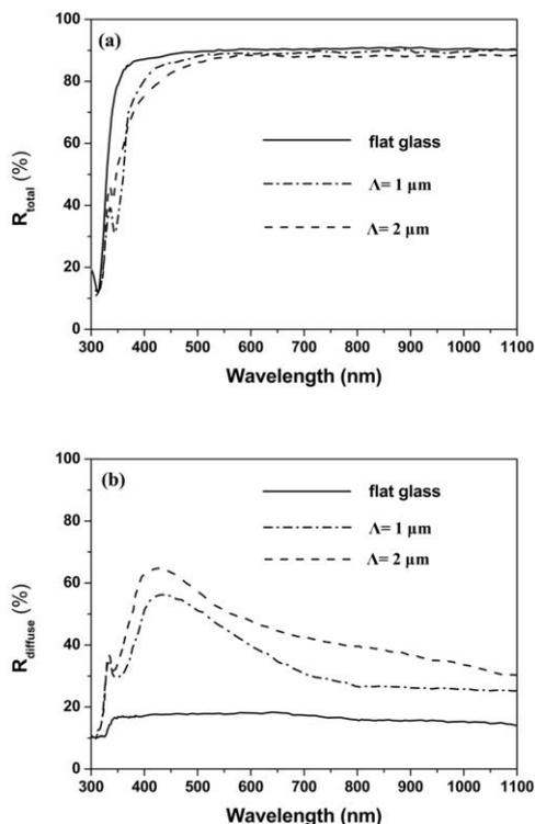
**Figure 4.** (a) Total reflectivity and (b) diffuse reflectivity spectra of the three back reflectors which were coated by Ag film.
