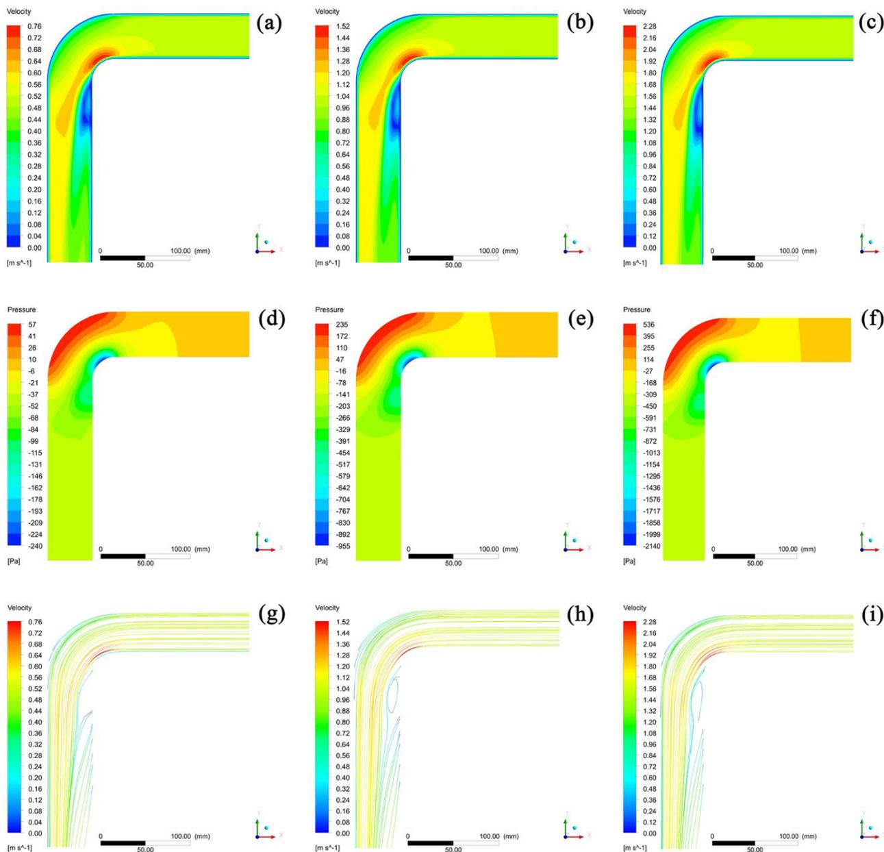
**Figure 5.** CFD simulation of the fluid flow velocity field distribution at the cross-section of pipe fitting at inlet fluid flow velocities of 0.5 m/s (a), 1.0 m/s (b), and 1.5 m/s (c); pressure distribution at inlet fluid flow velocities of 0.5 m/s (d), 1.0 m/s (e), and 1.5 m/s (f); and streamline contour at inlet fluid flow velocities of 0.5 m/s (g), 1.0 m/s (h), and 1.5 m/s (i).
