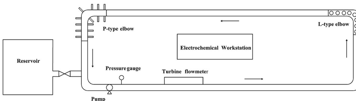
**Figure 3.** Dynamic corrosion platform.
