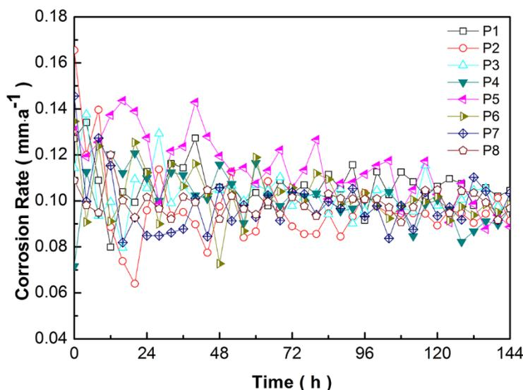
**Figure 11.** Corrosion rate of P-type pipe fitting in a stationary state.
