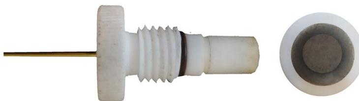
**Figure 1.** Specific form of the single electrode.
