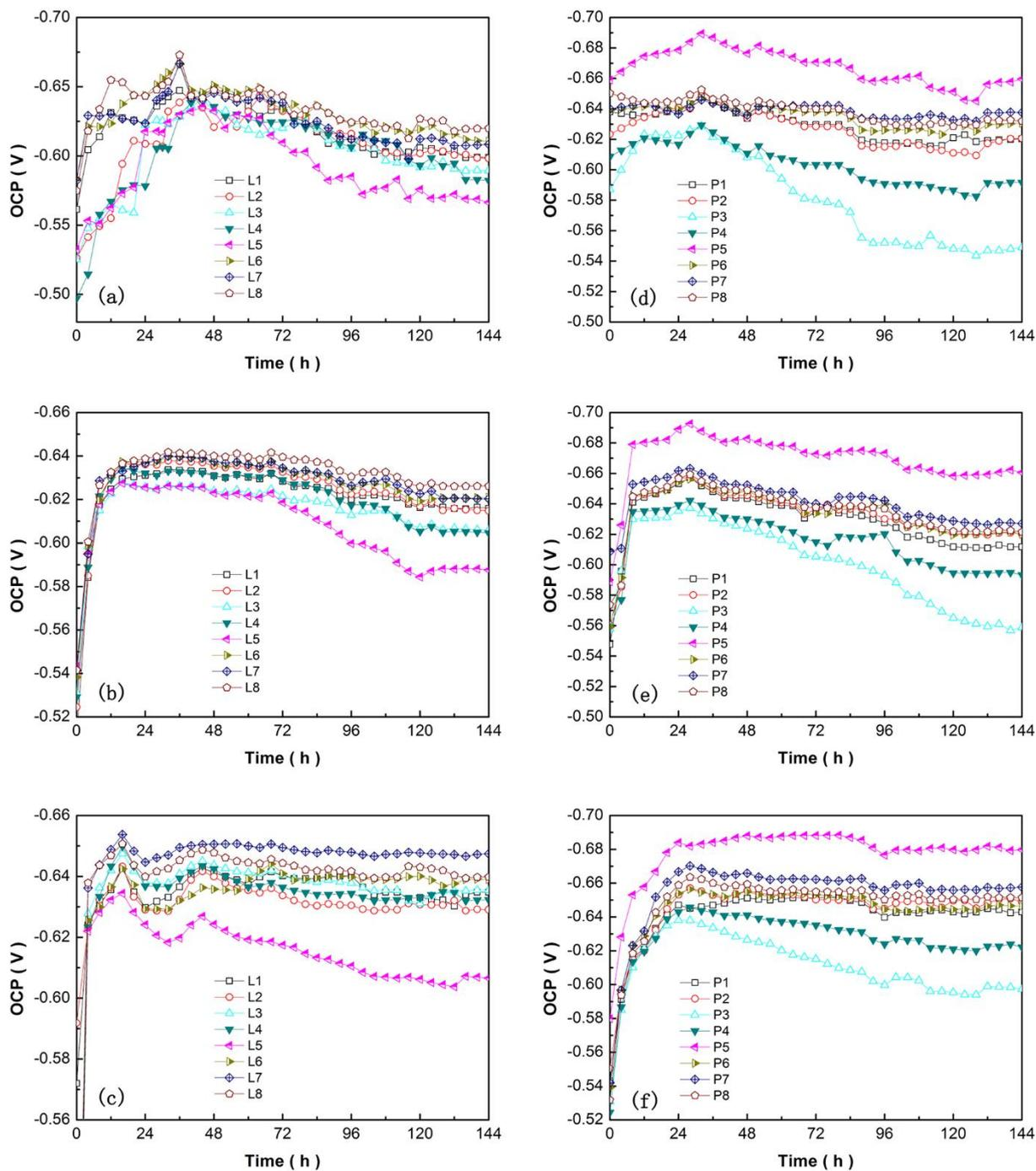
**Figure 9.** OCP measurements of L-type pipe fitting at inlet fluid flow velocities of 0.5 m/s (a), 1.0 m/s and (b), 1.5 m/s (c); and OCP measurements of P-type pipe fitting at inlet fluid flow velocities of 0.5 m/s (d), 1.0 m/s and (e), 1.5 m/s (f).
