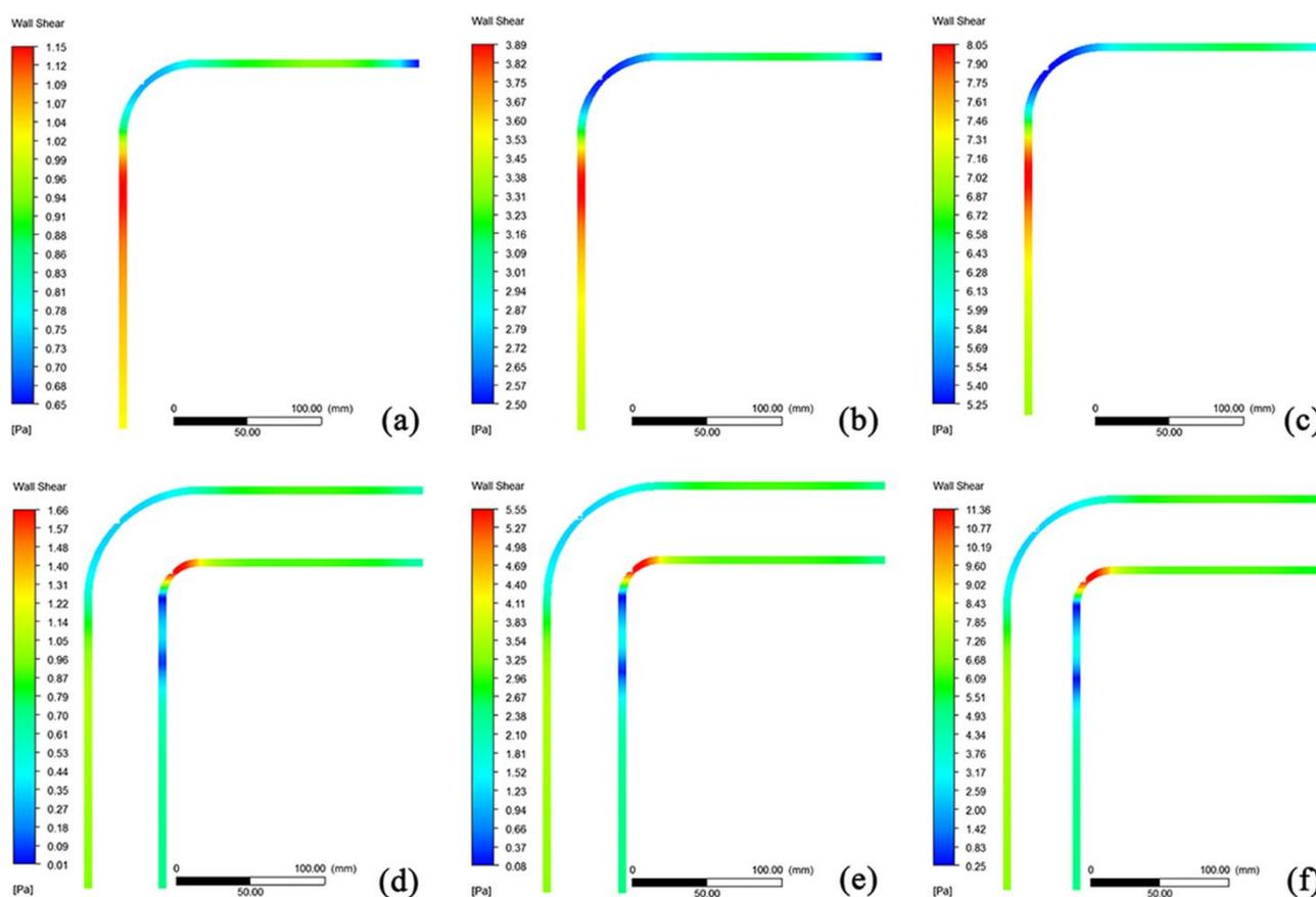
**Figure 6.** CFD simulation of wall shear stress distribution at the cross-section in the pipe fitting at inlet fluid flow velocities of 0.5 m/s (a), 1.0 m/s (b), and 1.5 m/s (c); and the top (bottom) of the elbow at inlet fluid flow velocities of 0.5 m/s (d), 1.0 m/s (e), and 1.5 m/s (f).
