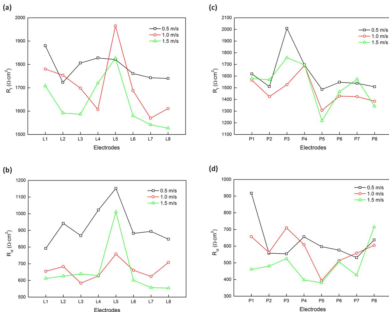
**Figure 17.** Fitted values of  $R_f$  and  $R_{ct}$  on L-type (a, b) and P-type (c, d) pipe fittings at an inlet fluid flow velocity of 0.5 m/s, 1.0 m/s, and 1.5 m/s.
