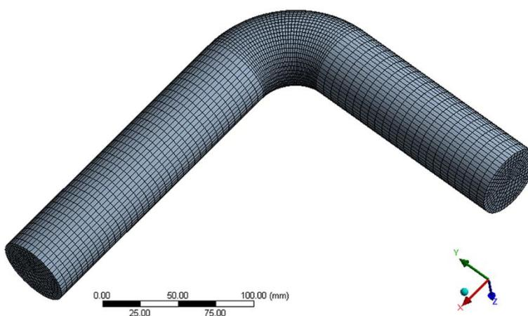
**Figure 4.** Meshing of model used in CFD simulation.
