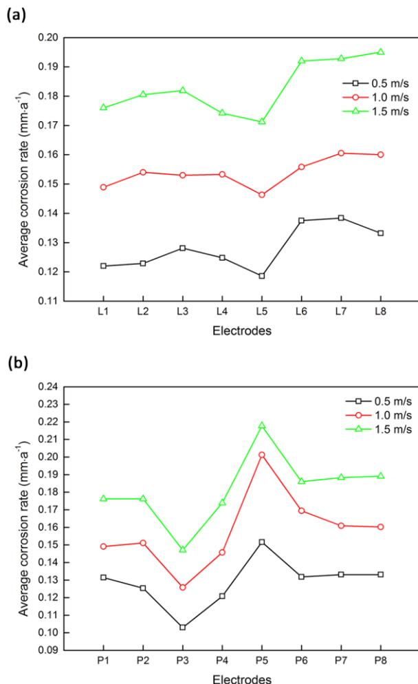
**Figure 13.** Stable average corrosion rate of each electrode of L-type pipe fitting (a) and P-type pipe fitting (b) after 144 h at an inlet fluid flow velocity of 0.5 m/s, 1.0 m/s and 1.5 m/s.
