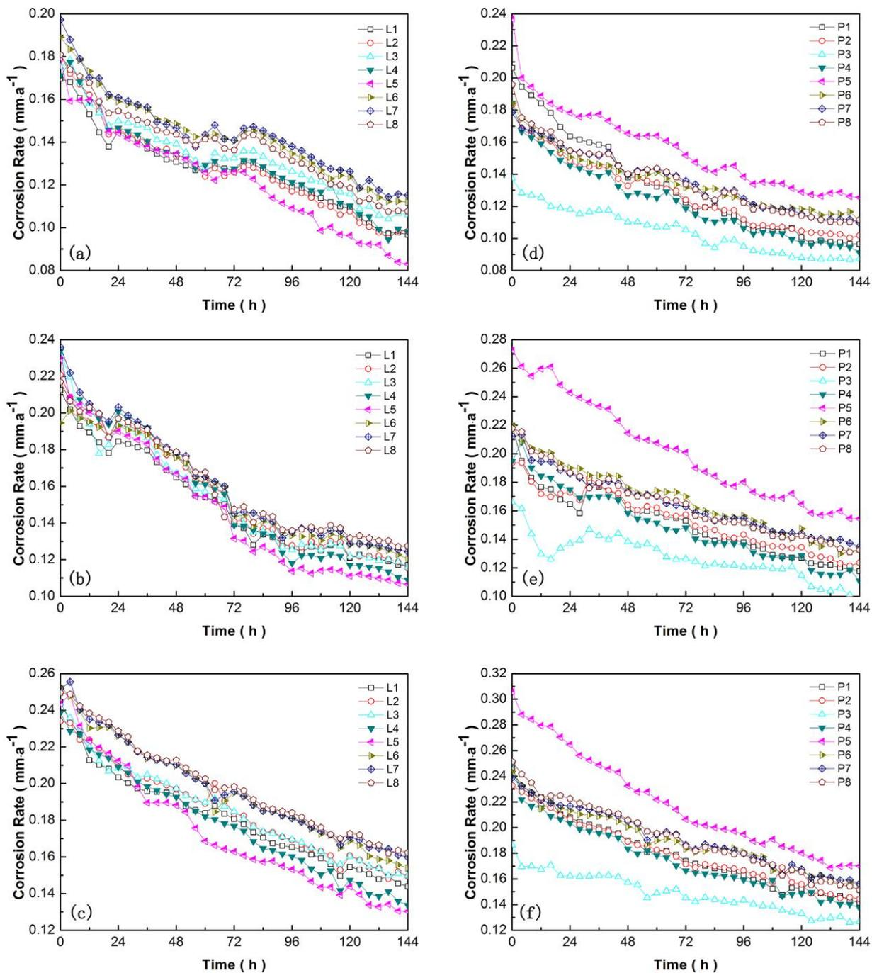
**Figure 12.** Corrosion rate of L-type pipe fitting at inlet fluid flow velocities of 0.5 m/s (a), 1.0 m/s (b), and 1.5 m/s (c), and corrosion rate of P-type pipe fitting at inlet fluid flow velocities of 0.5 m/s (d), 1.0 m/s (e), and 1.5 m/s (f).
