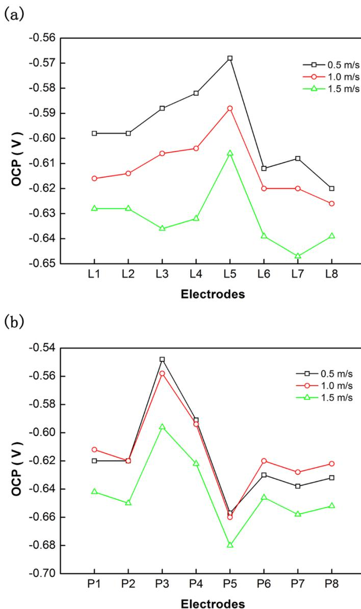
**Figure 10.** Stable average OCP of each electrode of L-type pipe fitting (a) and P-type pipe fitting (b) after 144 h at inlet fluid flow velocities of 0.5 m/s, 1.0 m/s and 1.5 m/s.
