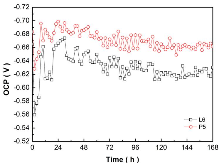
**Figure 7.** OCP changes on electrode L6 and P5 at an inlet velocity of 1.5 m m/s over 168 h.
