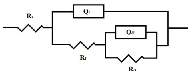
**Figure 16.** Equivalent circuit for EIS fitting.
