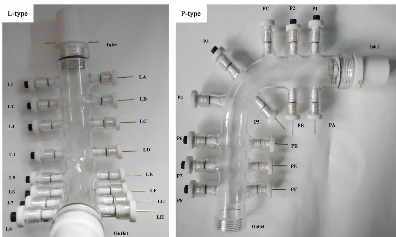
**Figure 2.** L-type (left) and P-type (right) elbow pipe fittings.
