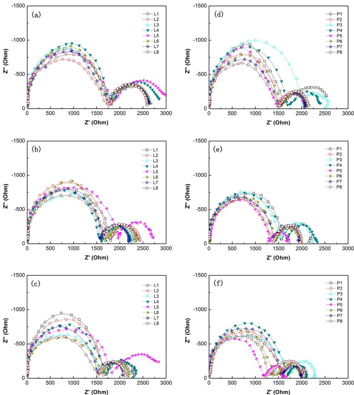
**Figure 15.** EIS plots measured on L-type pipe fittings at inlet fluid flow velocities of 0.5 m/s (a), 1.0 m/s (b), and 1.5 m/s (c), and EIS plots measured on P-type pipe fittings at inlet fluid flow velocities of 0.5 m/s (d), 1.0 m/s (e), and 1.5 m/s (f).
