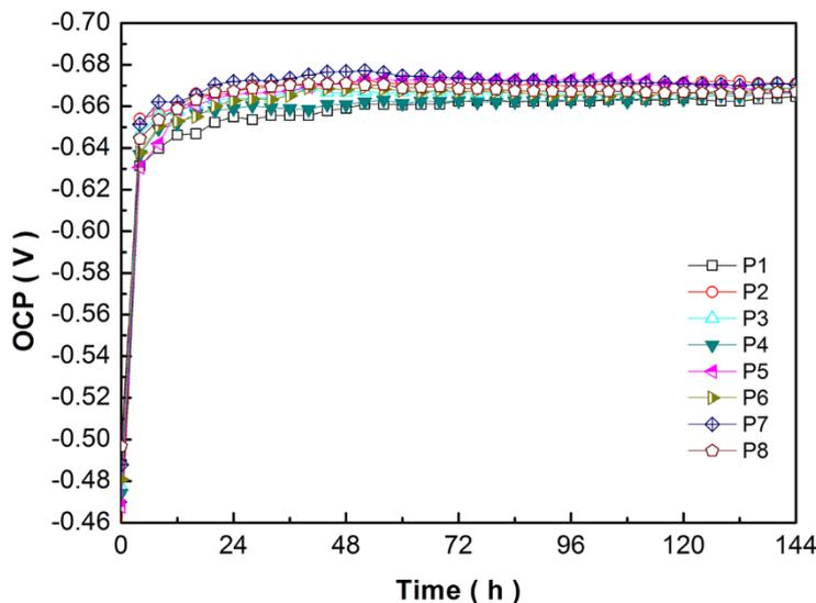
**Figure 8.** OCP measurements of P-type pipe fitting in a stationary state.
