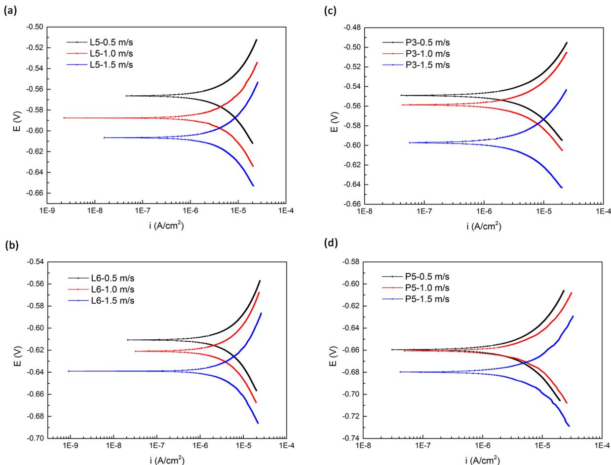
**Figure 14.** Polarization curves of L5 (a), L6 (b), P3 (c), and P5 (d) at an inlet fluid flow velocity of 0.5 m/s, 1.0 m/s, and 1.5 m/s.
