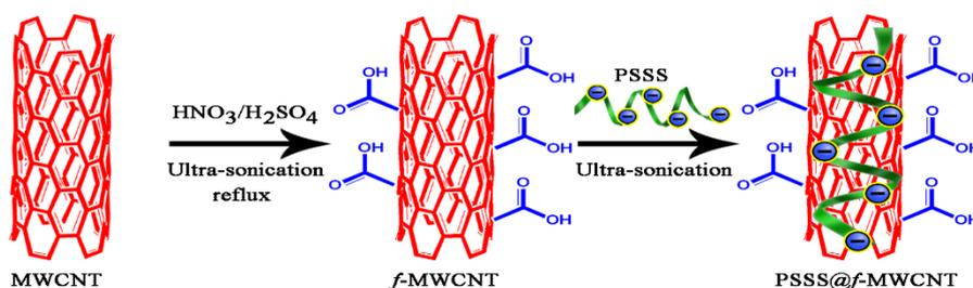
**Scheme 1.** Preparation of PSSS@*f*-MWCNTs composite.
