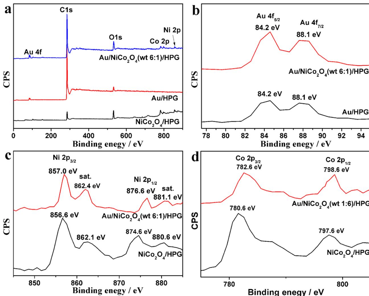
**Figure 2.** XPS spectra for Au/NiCo<sub>2</sub>O<sub>4</sub>(wt 6:1)/HPG of (a) survey, (b) Au 4f, (c) Ni 2p and (d) Co 2p.
