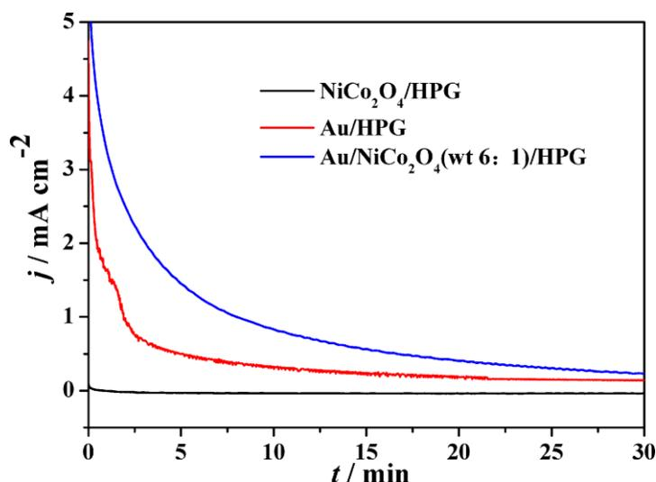
**Figure 5.** Chronoamperometry curves on NiCo<sub>2</sub>O<sub>4</sub>/HPG, Au/HPG and Au/NiCo<sub>2</sub>O<sub>4</sub>(wt 6:1)/HPG electrodes in 1.0 mol·L<sup>-1</sup> KOH containing 1.0 mol·L<sup>-1</sup> glycerol at a potential of -0.3 V.
