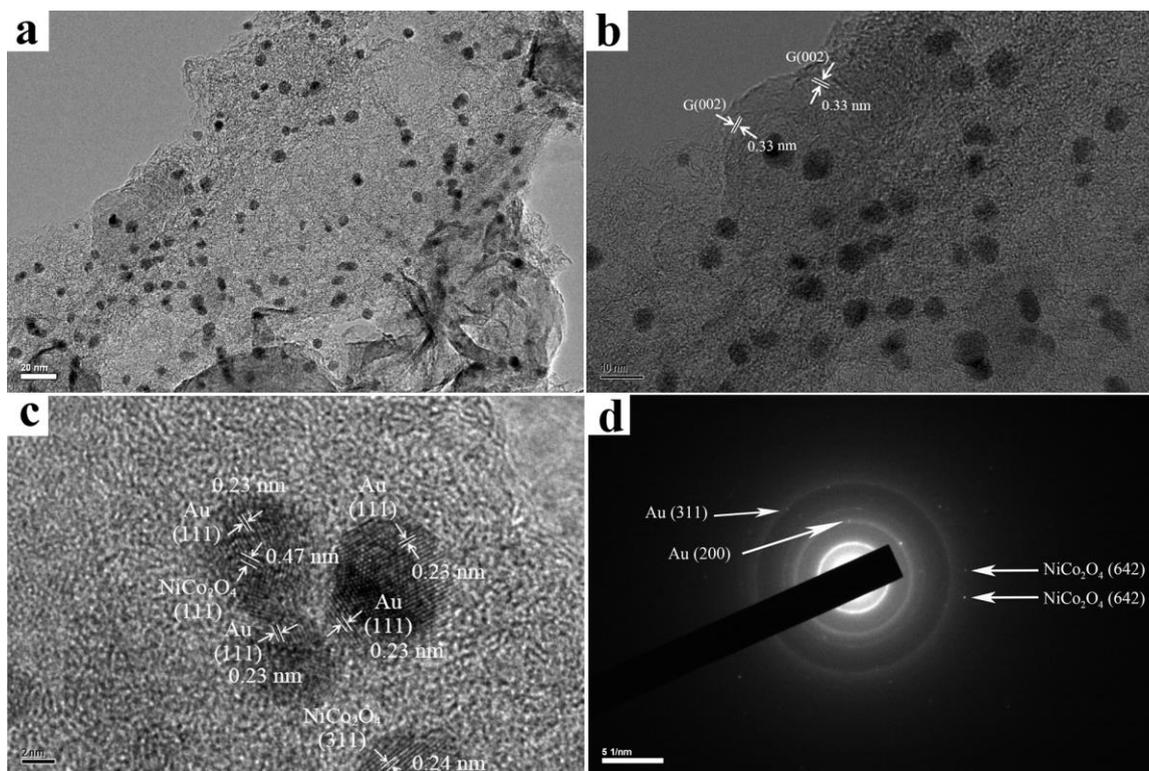
**Figure 3.** (a,b) TEM images, (c) HRTEM image and (d) SAED) pattern for Au/NiCo<sub>2</sub>O<sub>4</sub>(wt 6:1)/HPG.
