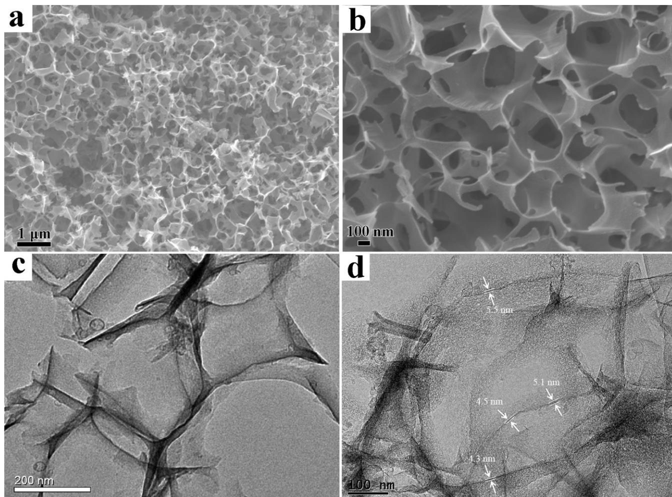
**Figure 1.** (a,b) SEM images and (c,d) TEM of 3D HPG.
