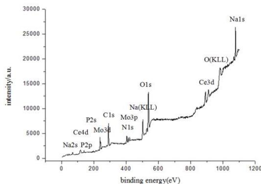
**Figure 5.** XPS spectra of protective film on steel surface formed by the ternary inhibitor after immersion for 72h at 30°C
