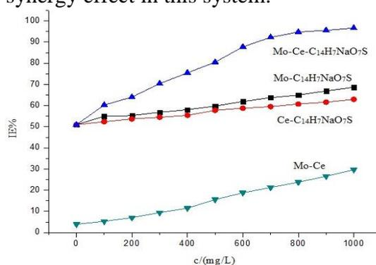
**Figure 2.** Inhibition efficiency for X80 steel in  $0.1\text{mol}\cdot\text{L}^{-1}$   $\text{H}_3\text{PO}_4$  solution of different corrosion inhibitor with different concentrations from weight loss method at  $30^\circ\text{C}$  for 72h
