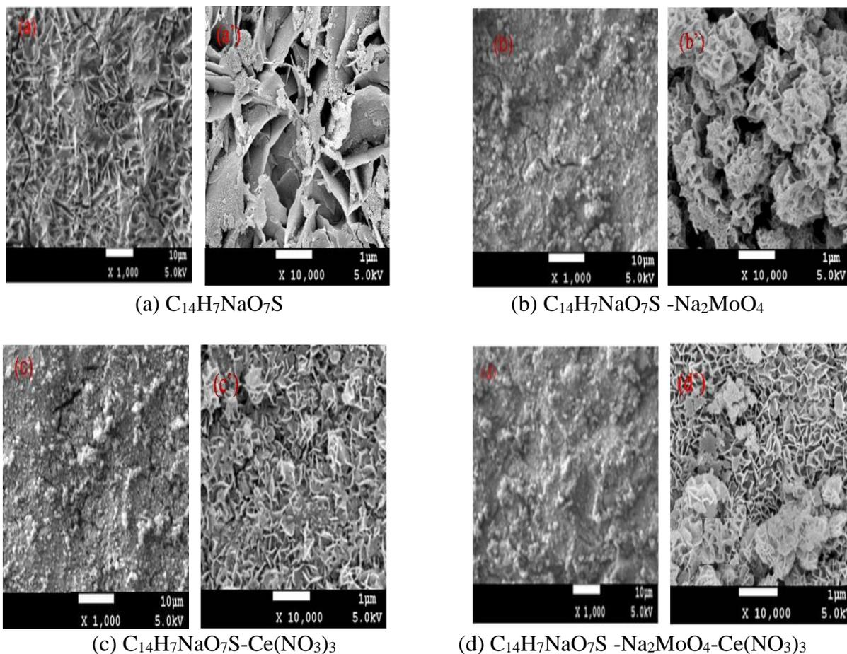
**Figure 4.** Microstructures of protective films on X80 steel surface formed by different inhibitors after immersion for 72h at 30°C
