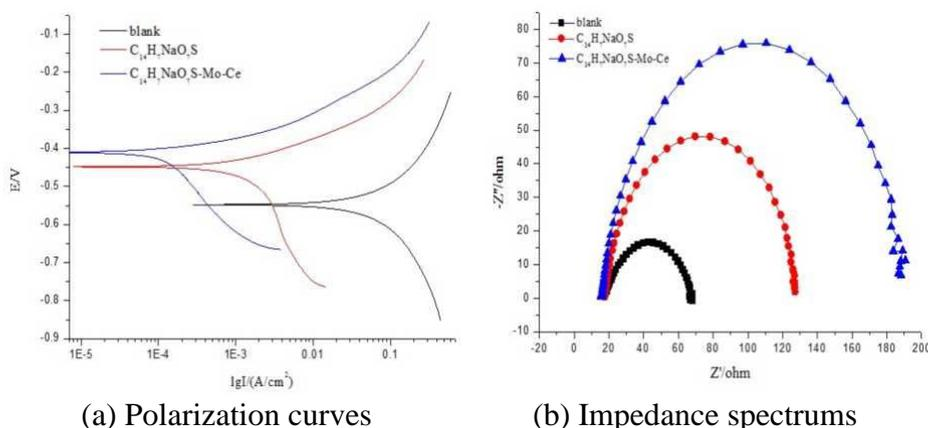
**Figure 3.** Electrochemical properties of X80 steel in 0.1mol·L<sup>-1</sup> H<sub>3</sub>PO<sub>4</sub> solution with and without different inhibitors at 30°C
