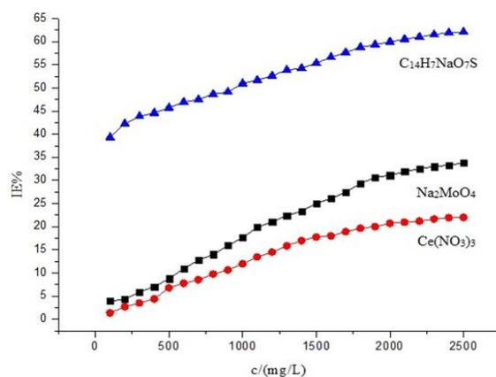
**Figure 1.** Inhibition efficiency for X80 steel in  $0.1 \text{ mol} \cdot \text{L}^{-1}$   $\text{H}_3\text{PO}_4$  solution of different corrosion inhibitor with different concentrations from weight loss method at  $30^\circ\text{C}$  for 72h
