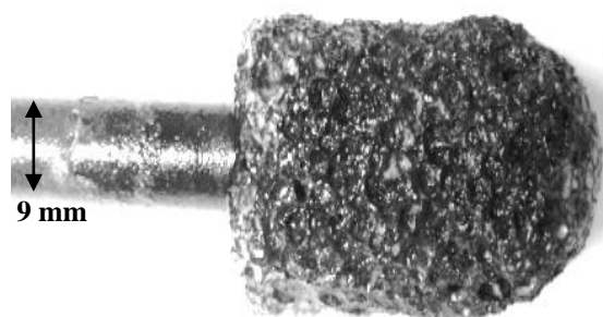
Figure 2. The example of deposited solid on the cathode surface after 3 hours of electrolysis process in \text{CaCO}_3 – \text{Li}_2\text{CO}_3 – \text{LiCl} electrolyte at 550°C under voltage supply of 4V.
