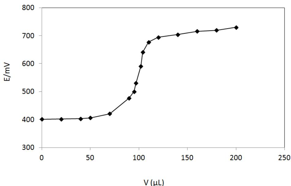
**Figure 4.** Potentiometric titration curve of 10.0 mL of a  $0.0001 \text{ mol l}^{-1}$  Fe(III) solution, with a  $0.01 \text{ mol l}^{-1}$  EDTA using the proposed membrane sensor as an indicator electrode.
