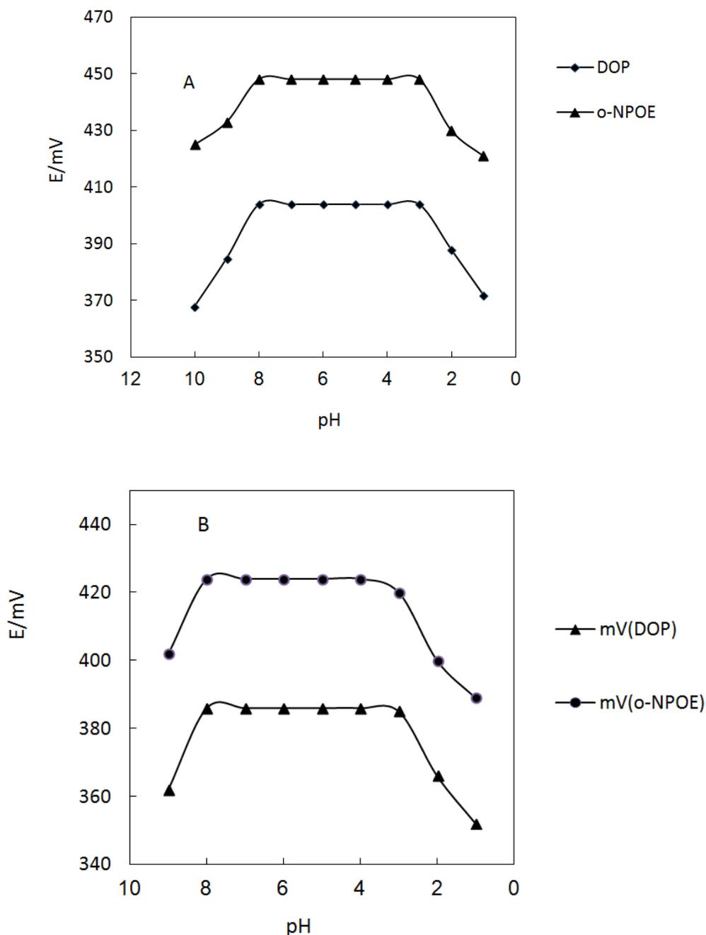
**Figure 3.** pH-potential Profile of Fe(III) membrane sensors at different concentrations. (A) 0.01 mol l<sup>-1</sup> (B) 0.001 mol l<sup>-1</sup>.
