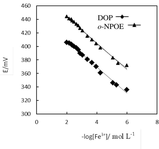
**Figure 1.** Calibration curve of the Fe(III) membrane sensors.
