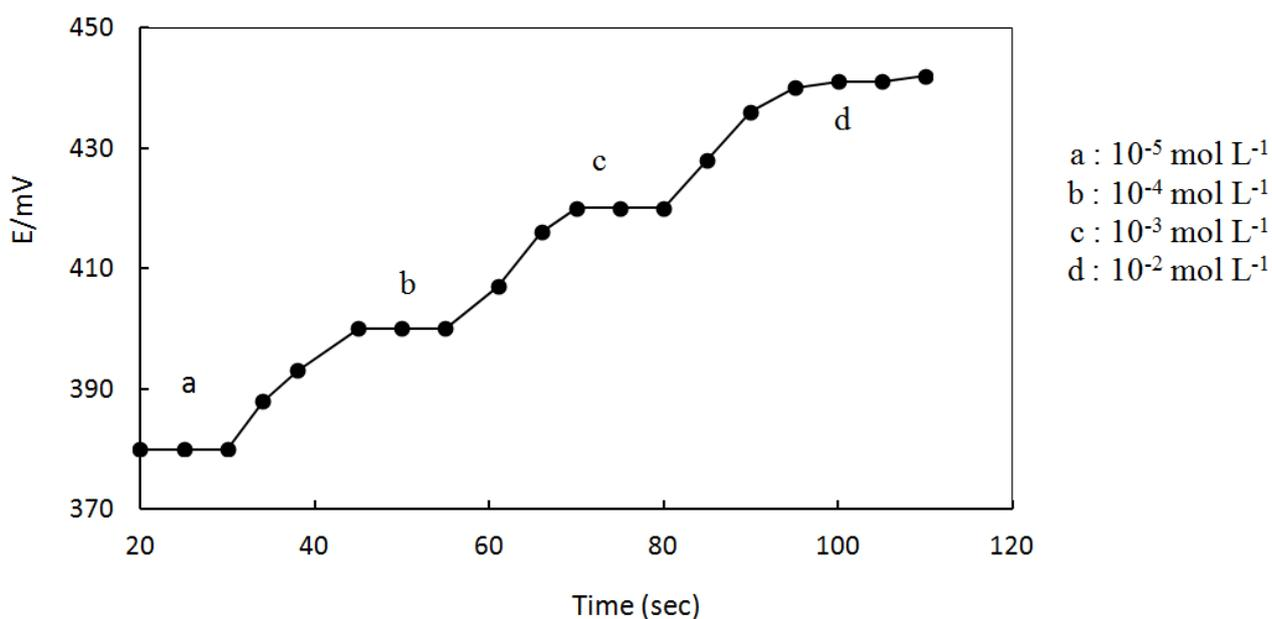
**Figure 2.** Dynamic response time of the electrode for step changes in the concentration of Fe(III).
