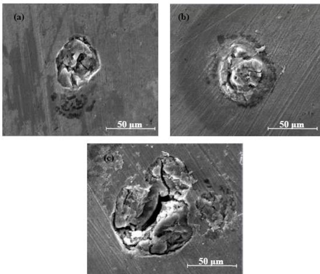
**Figure 4.** SEM micrographs of pits on the specimens after potentiostatic polarization in the different test solution: (a) 10 ppm  $\text{Cl}^-$ , (b) 10 ppm  $\text{Cl}^-$  + 5 ppm  $\text{SO}_4^{2-}$ , (c) 10 ppm  $\text{Cl}^-$  + 10 ppm  $\text{SO}_4^{2-}$
