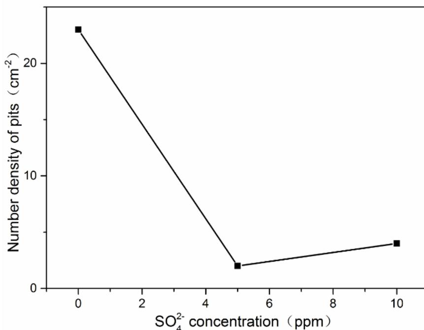
**Figure 3.** Number density of pits on specimens after potentiostatic polarization in the test solution with 10ppm  $\text{Cl}^-$  and added different concentration of  $\text{SO}_4^{2-}$
