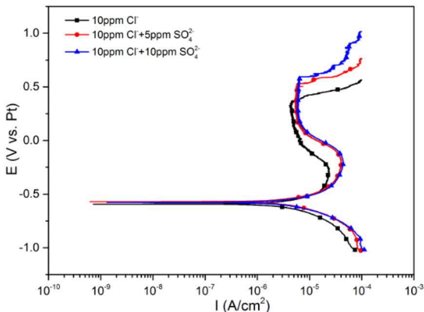
**Figure 1.** Polarization curves of 2Cr12MoV steel in the test solution with 10ppm  $\text{Cl}^-$  and added different concentration of  $\text{SO}_4^{2-}$
