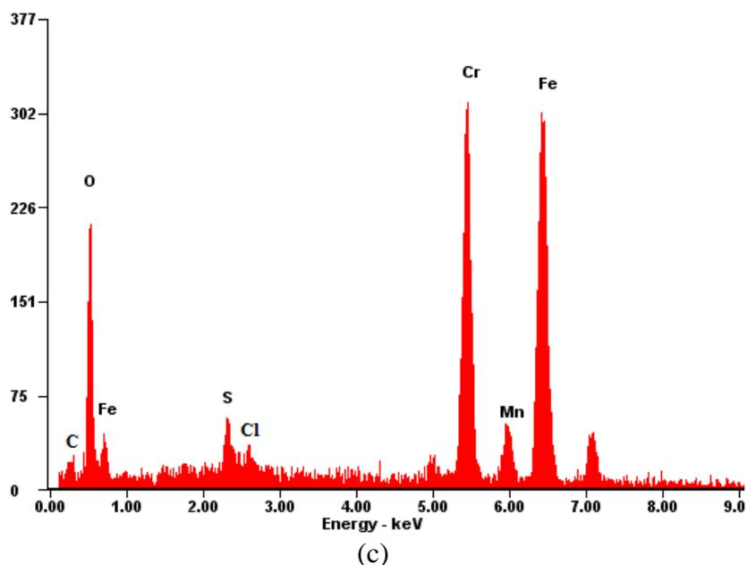
**Figure 5.** EDS spectra for corrosion products of inside pits on the specimens after potentiostatic polarization in different test solution: (a) 10 ppm  $\text{Cl}^-$ , (b) 10 ppm  $\text{Cl}^-$  + 5 ppm  $\text{SO}_4^{2-}$ , (c) 10 ppm  $\text{Cl}^-$  + 10 ppm  $\text{SO}_4^{2-}$
