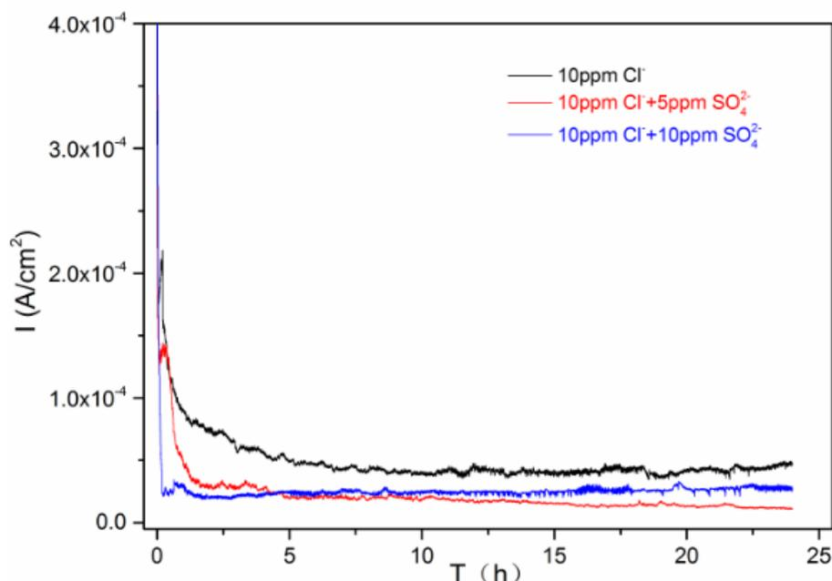
**Figure 2.** Current density varies with time for 2Cr12MoV steel in different test solution during potentiostatic polarization at applied 0.59 V (vs. Pt).
