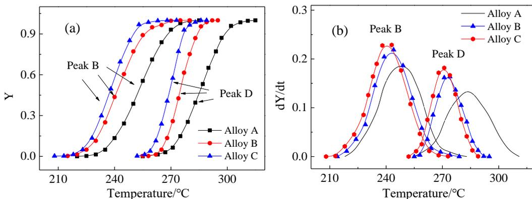
**Figure 7.** Plots of Y vs. T and  $dY/dt$  vs. T for the peak of  $\beta''$  phase and  $\beta'$  phase. (a) Plots of Y vs. T for the peak of  $\beta''$  phase and  $\beta'$  phase; (b) Plots of  $dY/dt$  vs. T for the peak of  $\beta''$  phase and  $\beta'$  phase
