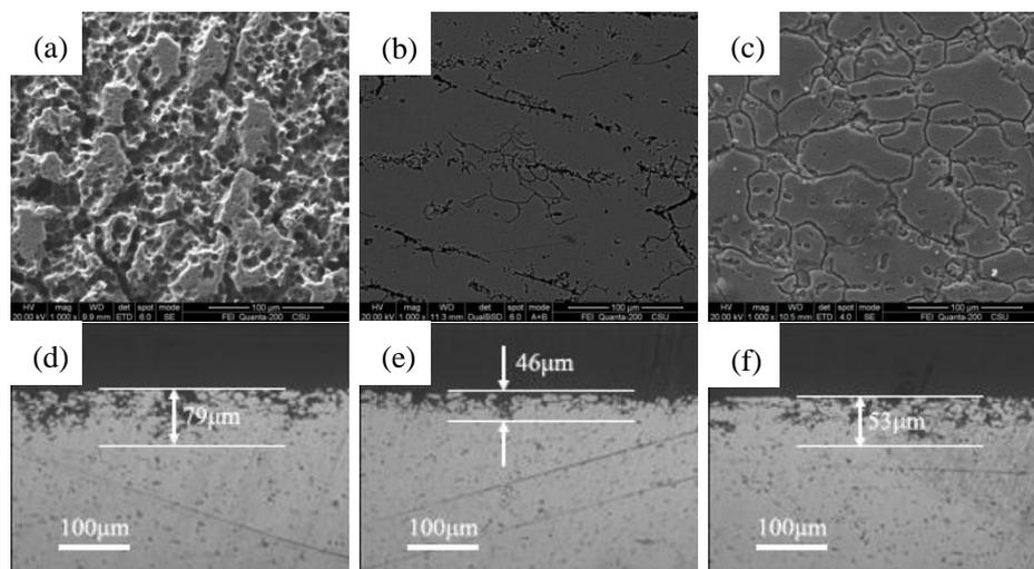
**Figure 2.** Surface morphologies and corresponding cross-sections of the corroded alloys with different Ag contents: (a,d) alloy A, (b,e) alloy B, and (c,f) alloy C.
