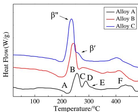
**Figure 5.** DSC curves of the tested alloys
