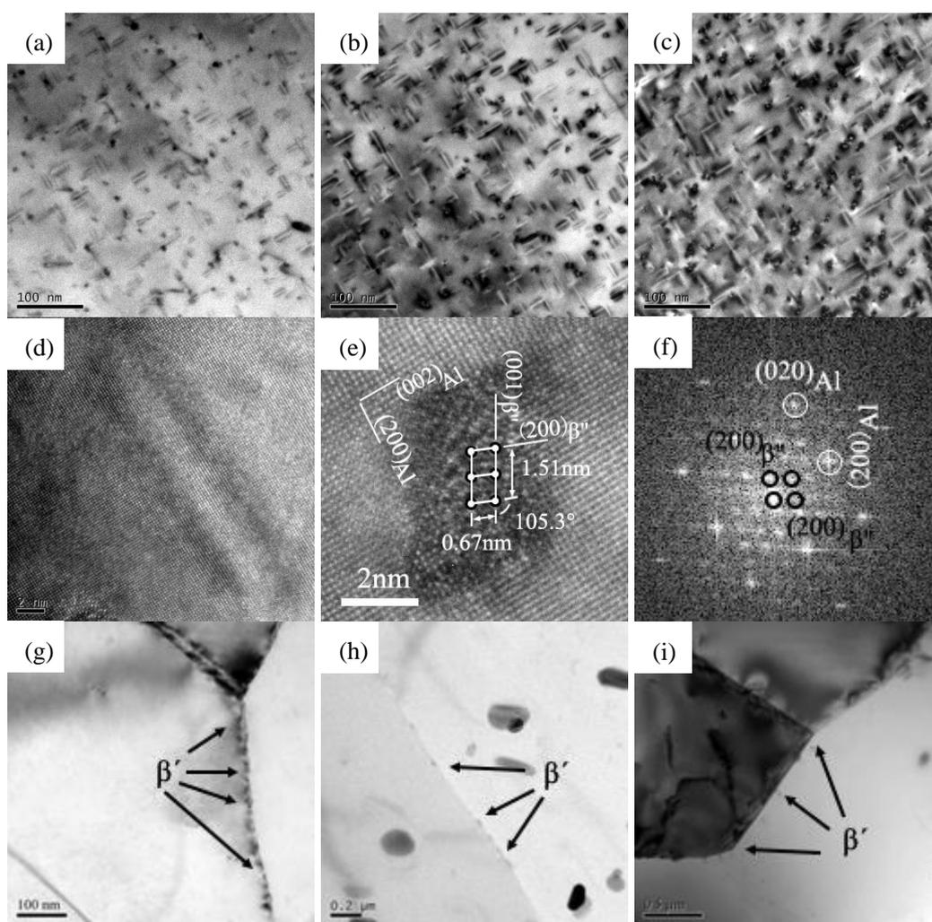
**Figure 4.** TEM images of the alloys with different Ag. (a, g) Alloy A; (b, h) Alloy B; (c, i) Alloy C; (d) HRTEM images of a  $\beta''$  precipitate and (e, f) the corresponding FFT pattern.
