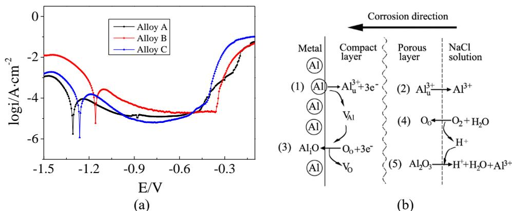
**Figure 3.** Polarization curves of the tested alloys and corrosion processes occurring in the oxide film. (a) Polarization curves of the tested alloys; (b) Physicochemical processes occurring in the oxide film.  $Al_u^{3+}$ : aluminum cation in a instability cation position.  $V_{Al}$ : aluminum vacancy at metal phase.  $V_o$ : oxygen vacancy at compact layer.  $O_o$ : oxygen ion in anion state
