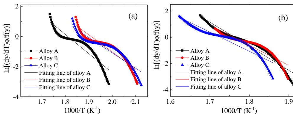
**Figure 8.** Plots of  $\ln[(dy/dT)\phi]$  vs.  $(1/T)$  for given Y values to determine the kinetic parameters of the  $\beta''$  and  $\beta'$  exothermic peaks of the three Alloys. (a)  $\beta''$  phase exothermic peak; (b)  $\beta'$  exothermic peak
