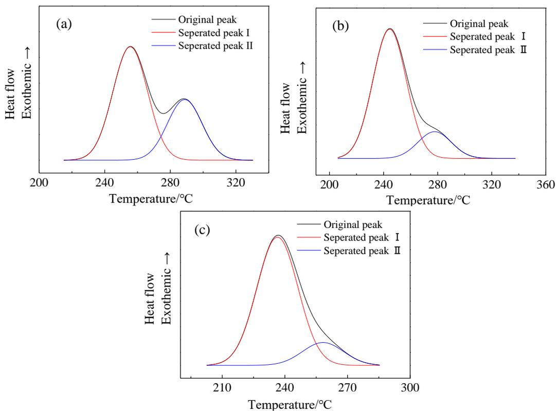
**Figure 6.** Separation results of overlap peak of  $\beta''$  phase and  $\beta'$  phase. (a) Alloy A; (b) Alloy B; (c) Alloy C
