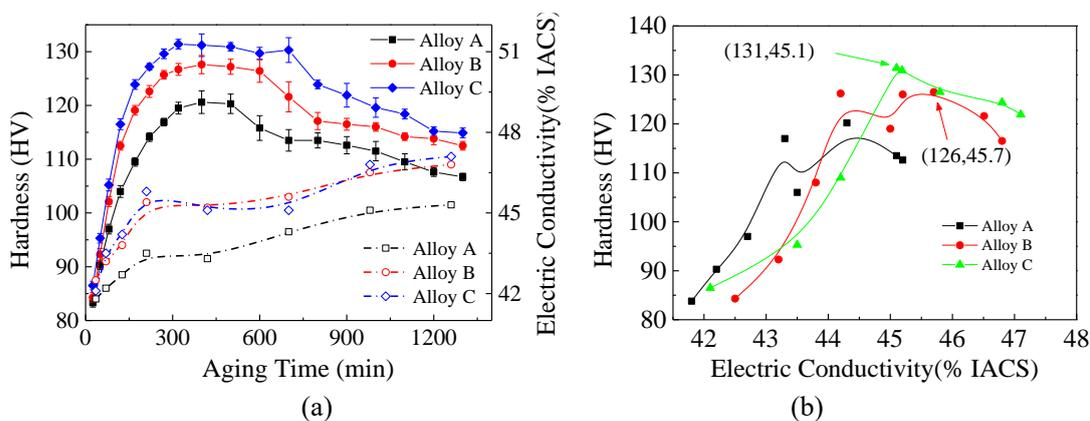
**Figure 1.** Relationships between hardness, electric conductivity of the samples and aging time: (a) Vickers hardness curves; (b) the hardness as a function of the electrical conductivity
