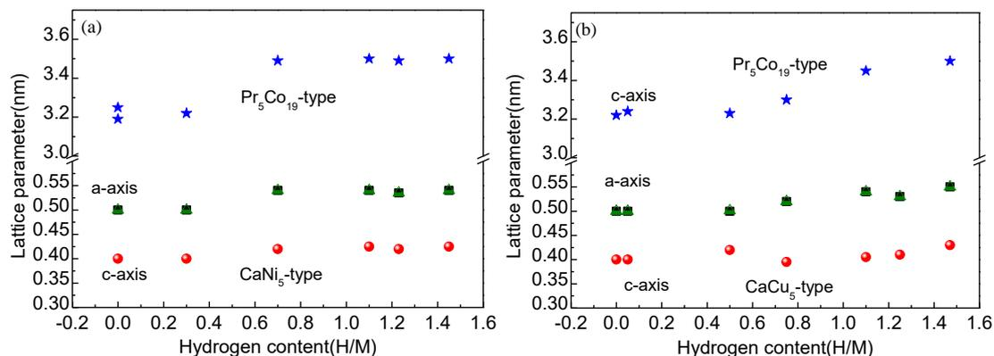
**Figure 9.** Lattice parameter of  $\text{LaNi}_5$ -type phase and  $\text{Pr}_5\text{Co}_{19}$ -type phase in hydriding/dehydriding (a) as-cast alloys (b) annealed alloys
