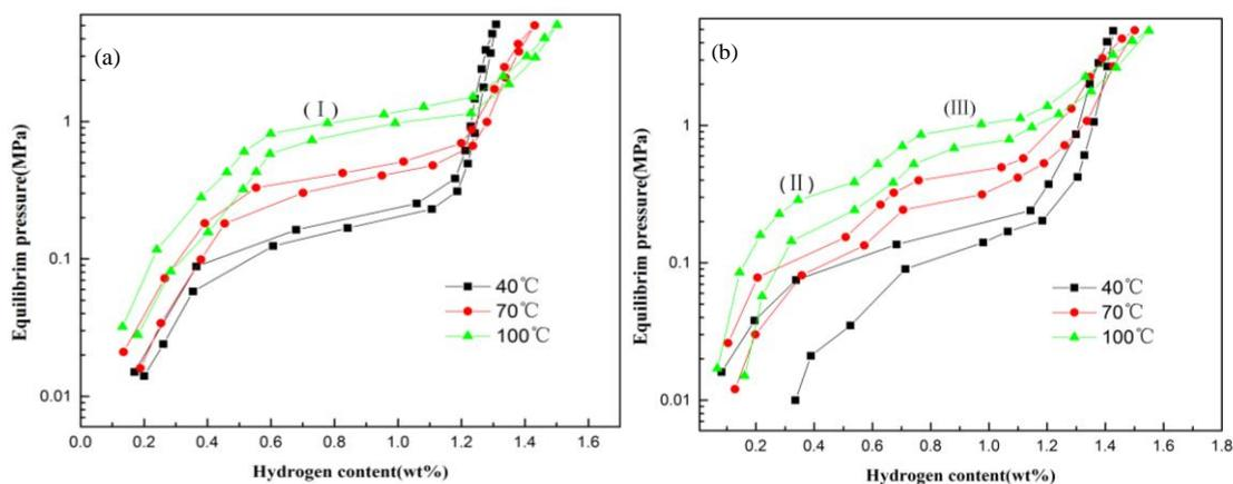
**Figure 3.** *P-C-T* curves of the as-cast (a) and annealed (b)  $\text{La}_{0.8}\text{Mg}_{0.2}\text{Ni}_{4.0}\text{Co}_{0.5}$  alloys at different temperatures.
