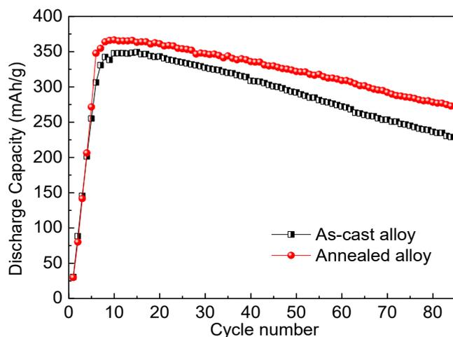
Figure 6. Discharge capacity of as-cast and annealed  $\text{La}_{0.8}\text{Mg}_{0.2}\text{Ni}_{4.0}\text{Co}_{0.5}$  alloys within 80 cycles.
