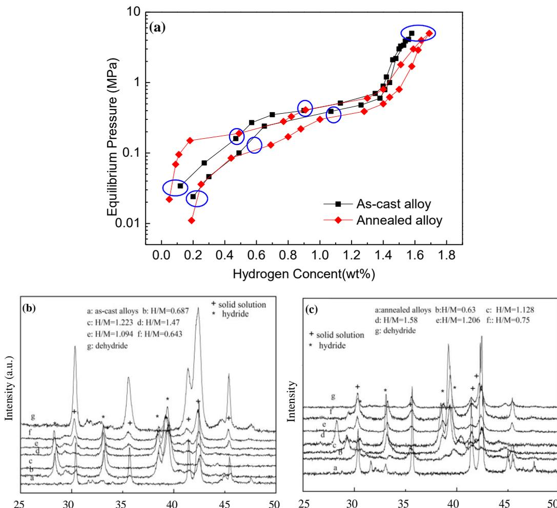
**Figure 8.** *P-C-T* curves (a) and XRD profiles of as-cast (b) and annealed (c)  $\text{La}_{0.8}\text{Mg}_{0.2}\text{Ni}_{4.0}\text{Co}_{0.5}$  alloys at different hydriding/dehydriding pressures of (a).
