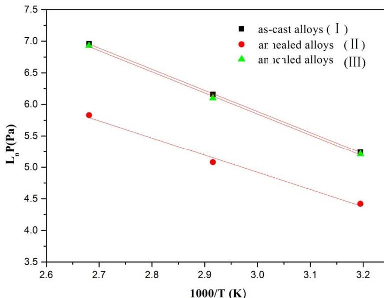
**Figure 4.** Van't Hoff plots for as-cast and annealed  $\text{La}_{0.8}\text{Mg}_{0.2}\text{Ni}_{4.0}\text{Co}_{0.5}$  alloys.
