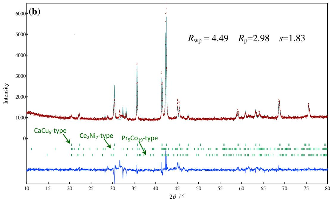
**Figure 1.** XRD profiles of the as-cast (a) and annealed (b)  $\text{La}_{0.8}\text{Mg}_{0.2}\text{Ni}_{4.0}\text{Co}_{0.5}$  alloys.  $\text{CaCu}_5$ -type,  $\text{Pr}_5\text{Co}_{19}$ -type and  $\text{Ce}_2\text{Ni}_7$ -type phases are used as the model. The phase peaks are shown with vertical bars, and the difference between the observed and calculated profiles is shown with the blue line below.
