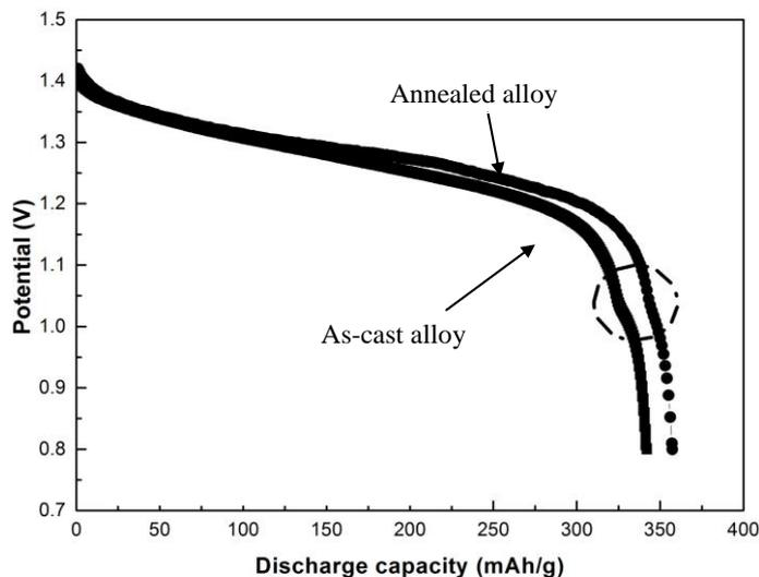
Figure 5. Discharge curves of as-cast and annealed  $\text{La}_{0.8}\text{Mg}_{0.2}\text{Ni}_{4.0}\text{Co}_{0.5}$  alloys
