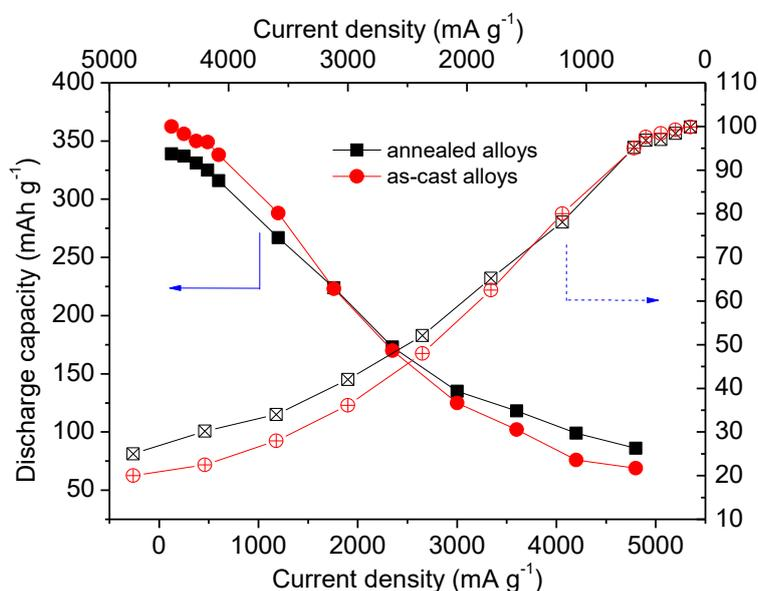
**Figure 7.** Discharge capacity and high rate dischargeability curves of as-cast and annealed  $\text{La}_{0.8}\text{Mg}_{0.2}\text{Ni}_{4.0}\text{Co}_{0.5}$  alloys
