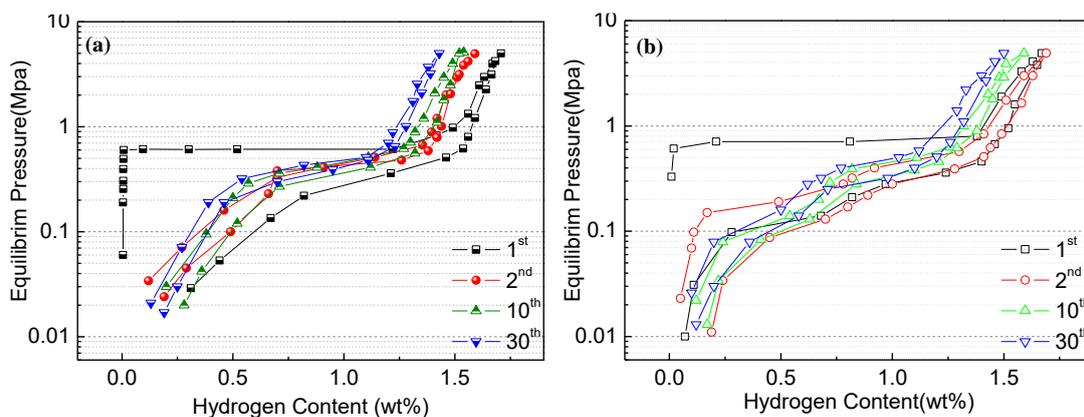
**Figure 2.** *P-C* curves at different cycles of as-cast (a) and annealed (b)  $\text{La}_{0.8}\text{Mg}_{0.2}\text{Ni}_{4.0}\text{Co}_{0.5}$  alloys at 70 °C.
