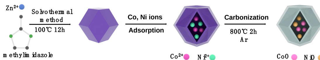
Figure 1. Synthetic scheme of CoO-NiO@ZIF-C
