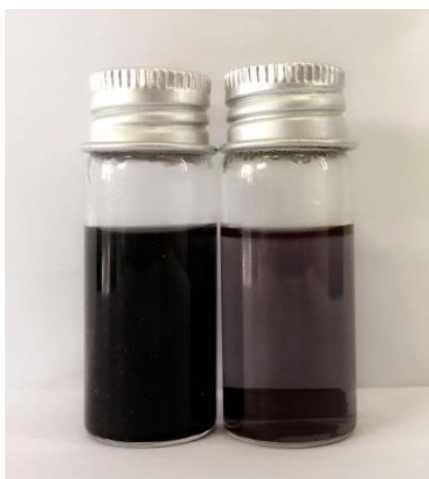
Figure 1. Photos show tubes containing mixture of reducing reagent ( \text{NaBH}_4 ) and \text{HAuCl}_4 solution (50:50); before (left), and after adding the inorganic monolith (right), showing changed the colour of the monolithic rod from white to black after incubation in oven at 100 ^{\circ}\text{C} for 4 h.
