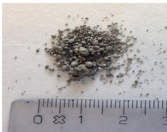
Figure 6 The photo of tin obtained by electrolysis.
