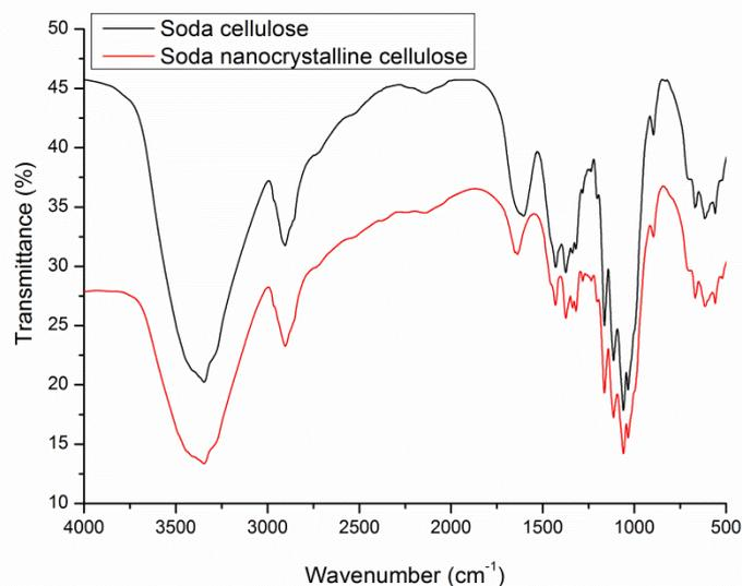
**Figure 2.** FTIR-spectra of Soda cellulose and Soda nanocrystalline cellulose
