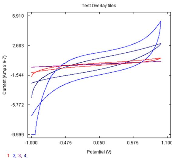
**Figure 9.** The overlay of cyclic voltammetry curves of the NCC-PHA-LiClO<sub>4</sub> polymer electrolyte film.
