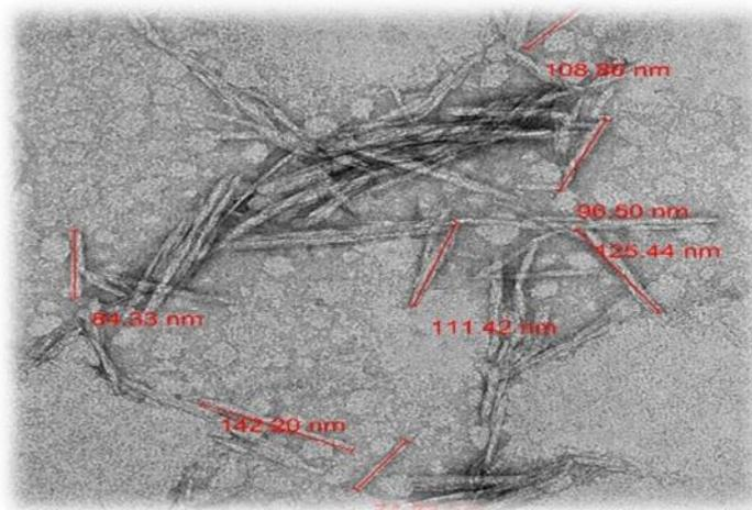
**Figure 6.** TEM image of Soda nanocrystalline cellulose
