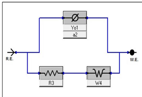
**Figure 7.** An equivalent electrical circuit used for electrochemical impedance spectroscopy (EIS) fitting
