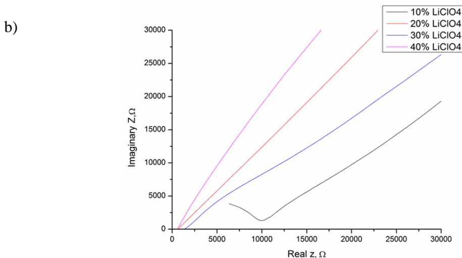
**Figure 8.** Nyquist plots of a) soda NCC-PHA-0 % LiClO<sub>4</sub> and b) Different percentage of LiClO<sub>4</sub> (10%, 20%, 30% and 40%) in soda NCC-PHA-LiClO<sub>4</sub> film
