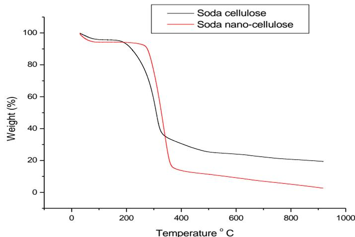
**Figure 5.** TGA thermograms of Soda cellulose and Soda nanocrystalline cellulose
