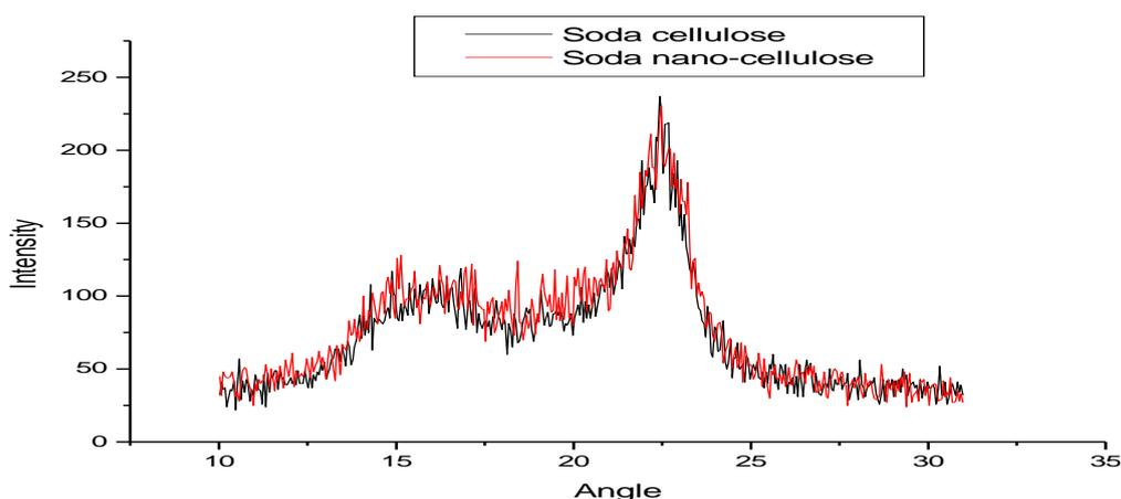
**Figure 4.** X-ray diffraction pattern of Soda cellulose and Soda nanocrystalline cellulose
