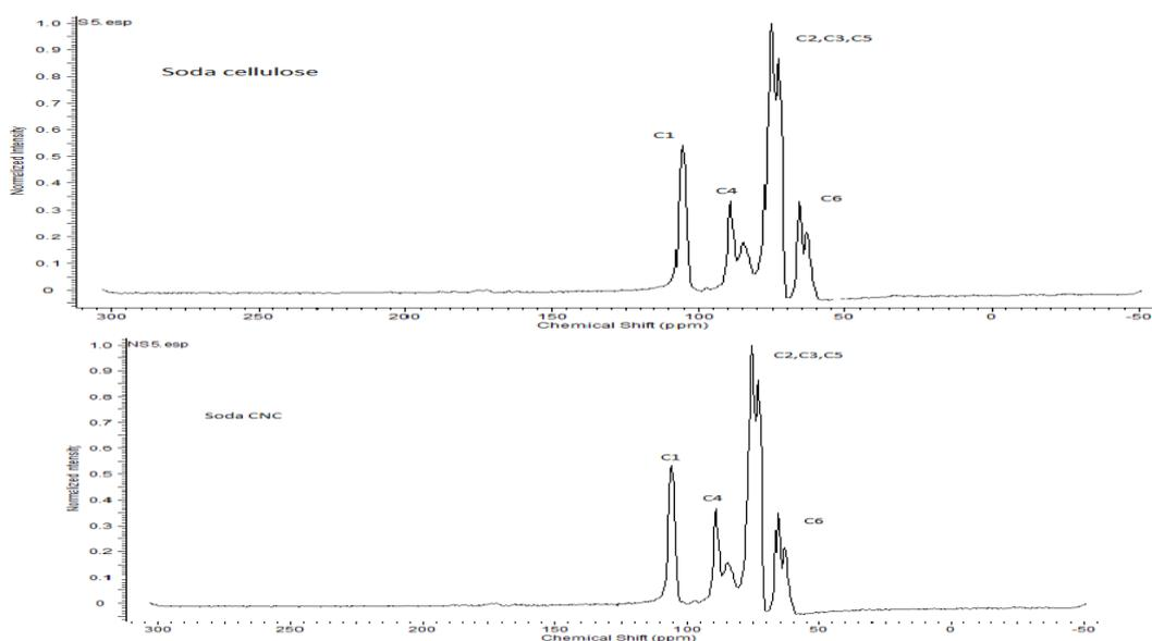
**Figure 3.** Solid state CP/ MAS  $^{13}\text{C}$  NMR spectra of Soda cellulose and Soda nanocrystalline cellulose
