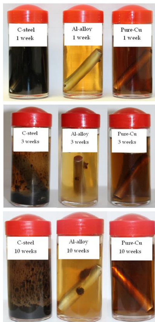
Figure 2. Optical photographs for ROWE/metal systems for different immersion times at room temperature ( 22 \pm 1 °C).
