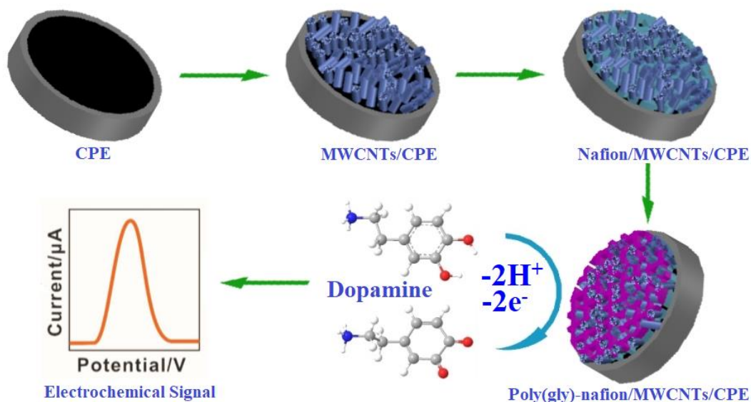
Scheme 1. Schematic illustration of Poly(gly)-nafion/MWCNTs/CPE fabrication
