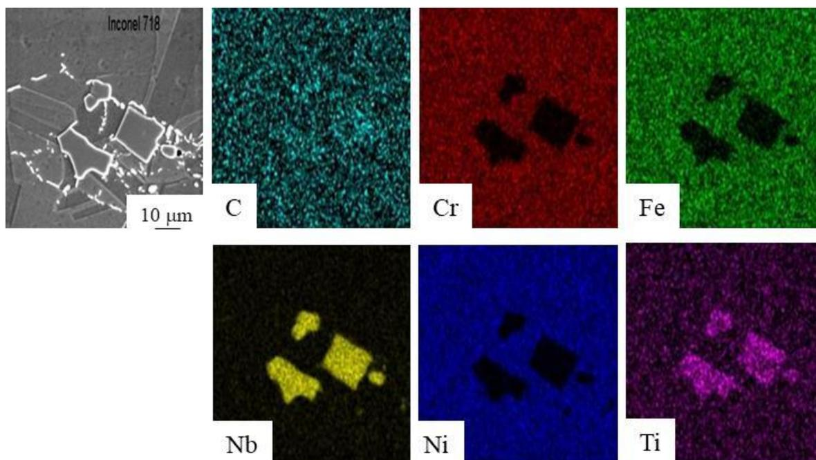
**Figure 3.** Elemental mapping performed in the BM of Inconel 718.
