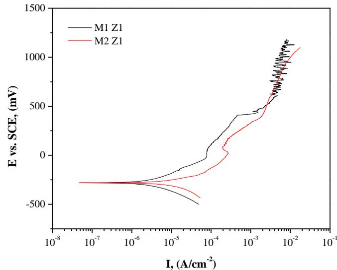
**Figure 8.** Potentiodynamic polarization; M1 low heat input, M2 high heat input.
