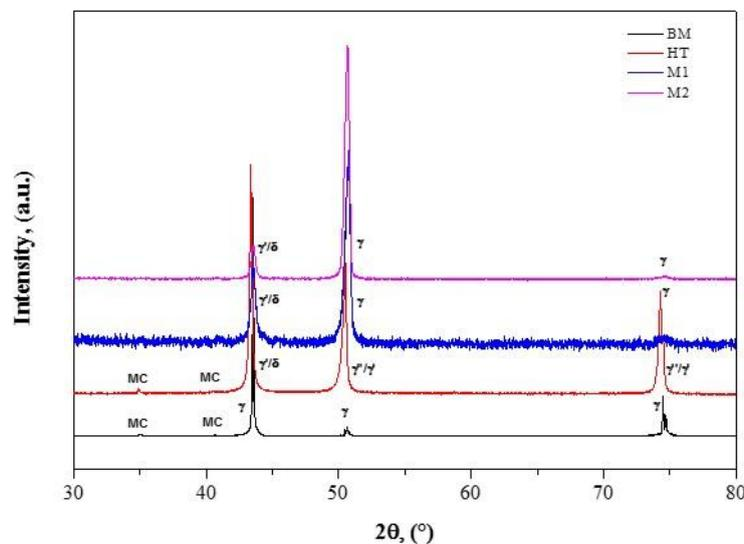
Figure 7. X ray diffraction analysis of the base metal, heat treatment and welds of Inconel 718.
