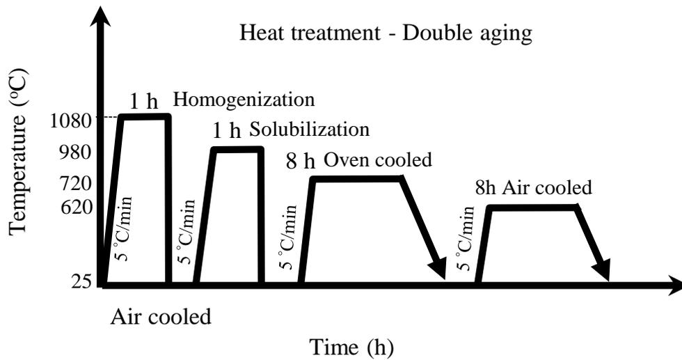
**Figure 1.** Heat treatment cycle performed in the samples of Inconel 718.
