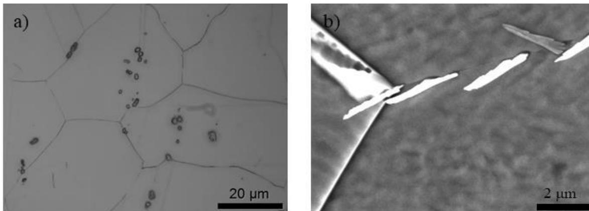
**Figure 4.** Images of heat treatment of Inconel 718; a) Optical, b) SEM.
