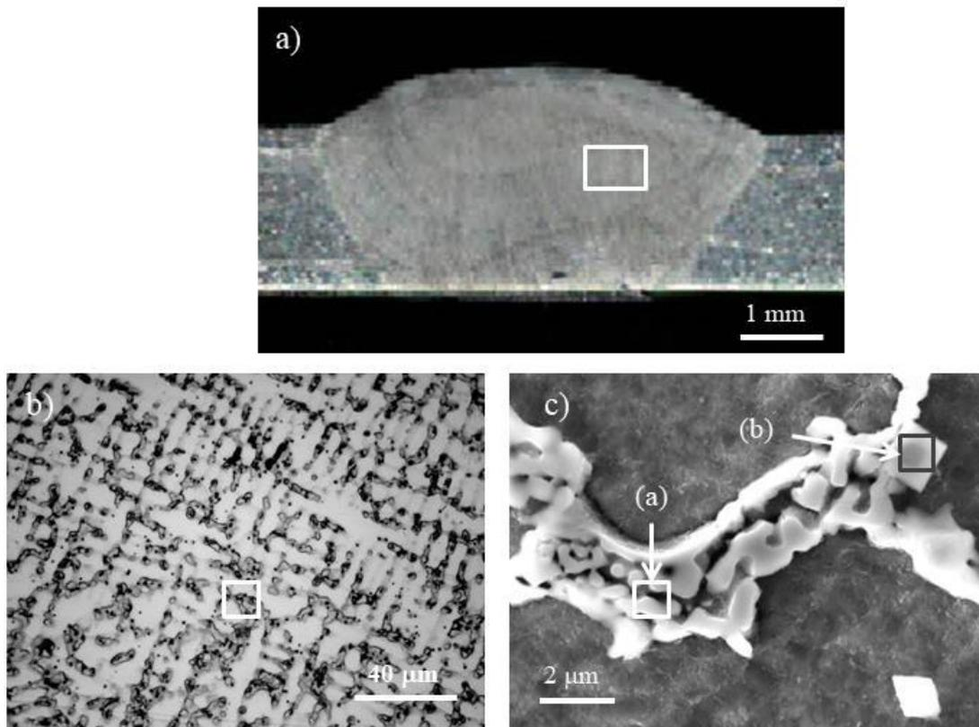
**Figure 6.** Weld of Inconel 718 with high heat input, a)macro, b) weld pool, c) analyzed particle.
