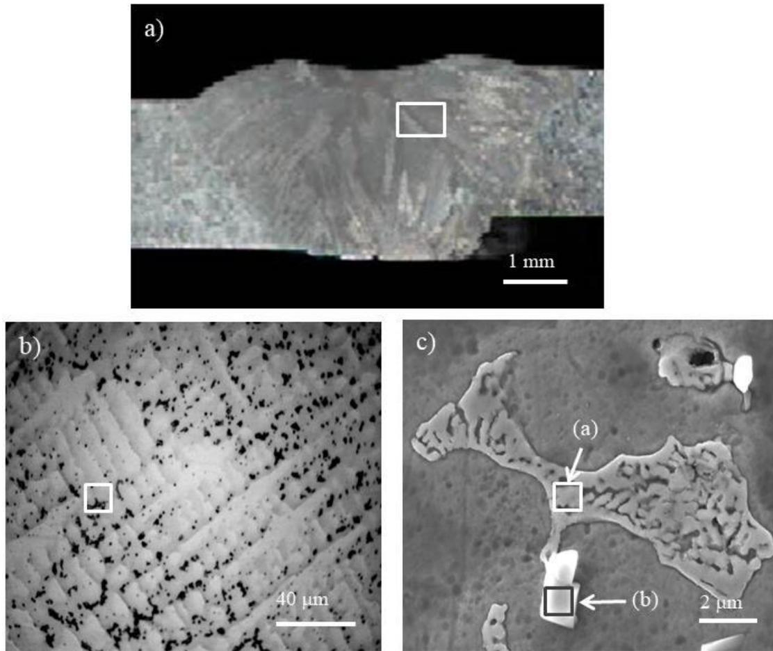
**Figure 5.** Weld of Inconel 718 with low heat input, a)macro, b) weld pool, c) analyzed particle.
