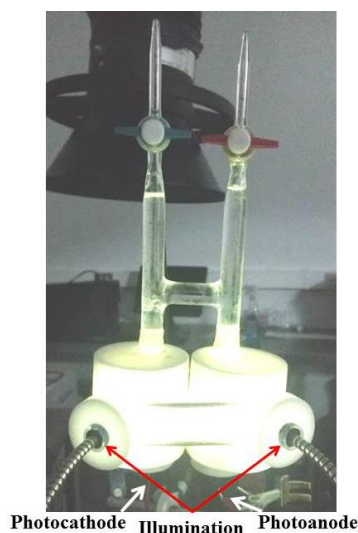
Figure 1. Photoelectrochemical cell used in the water electrolysis experiments, with photoelectrodes of n\text{-Fe}_2\text{O}_3 and p\text{-Cu}_2\text{O}
